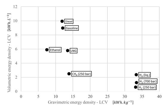
Figure 0.5 – Comparison of energy densities per mass and per volume of several liquid and gaseous fuels (LCV data from [6–8])
