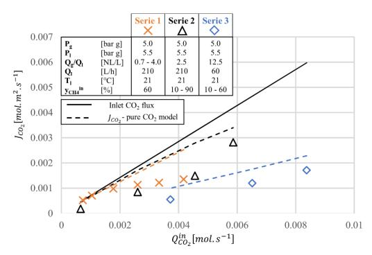
Figure 4.8 – Comparison of experimental and numerical absorbed CO<sub>2</sub> fluxes from a biogas mixture *Open-loop configuration*
