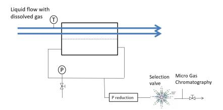
Figure 2.22 - Dissolved gas analytical module set-up
