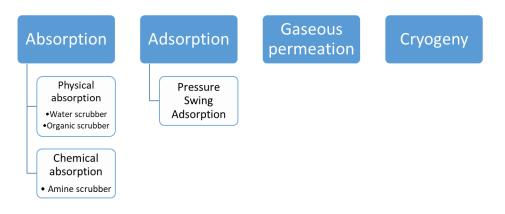
Figure 1.8 – Available biogas upgrading technologies according to their separation principle
