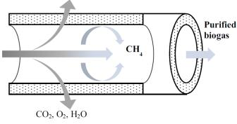
Figure 1.14 – Principle of membrane permeation [61]
