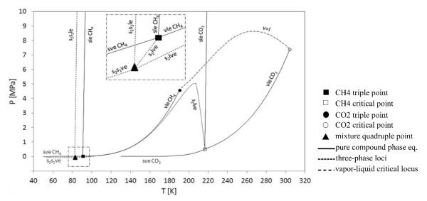
Figure D.1 – Pressure-temperature equilibrium behaviour for the CH<sub>4</sub>-CO<sub>2</sub> system [83]
