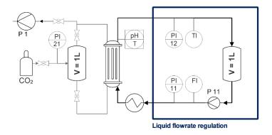
Figure 2.23 - Experimental set-up for the measurement of Henry coefficient
