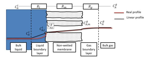
Figure 1.27- Concentration profile at the gas-liquid interface during absorption
