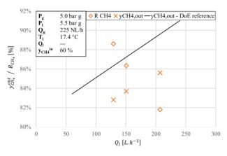
Figure 3.21 – Process performances of an alternative degassing system compared to reference configuration *The DoE curve is the response of the DoE model*
