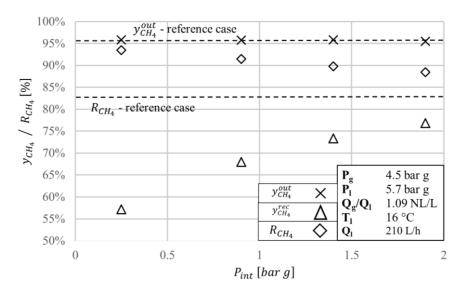
Figure 3.23 - Addition of methane recycling loop: influence of intermediate gas pressure
