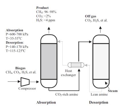
Figure 1.12 - Simplified process flow diagram of an amine scrubber [61]
