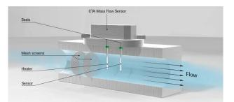
Figure 2.19 – Principle of the In-Flow CTA flowmeter [219]
