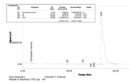
Figure 2.15 - Chromatogram of Molsieve 5Å column for a synthetic biogas sample
