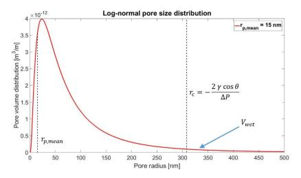
Figure 2.9 – Membrane log-normal pore size distribution Nomenclature is introduced in paragraph 1.6.3
