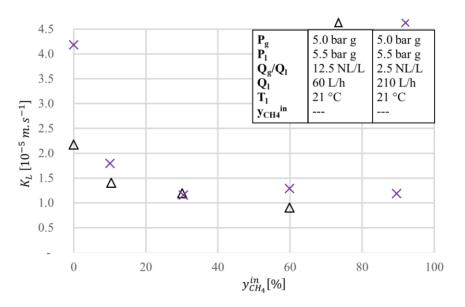
Figure 3.16 – Variation of the overall mass transfer coefficient K<sub>L</sub> according to the inlet gas composition *Open-loop configuration*
