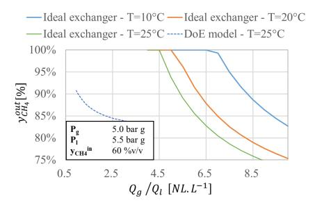
Figure 3.6 – Influence of  $Q_g/Q_1$  ratio on the biomethane quality: comparison of the DoE quadratic model with ideal exchanger performances DoE model is applied with  $Q_g = 205 \text{ NL} \cdot h^{-1}$
