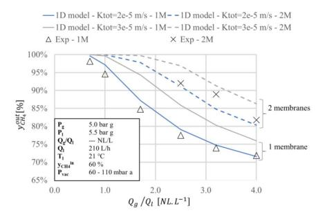
Figure 3.9 – Comparison of biomethane quality at different  $Q_g/Q_l$  ratio with one or two membrane modules (1M and 2M) *Open-loop configuration* – *Ktot* =  $K_L$
