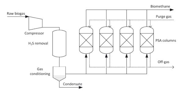
Figure 1.13 – Simplified process flow diagram of a PSA unit [59]
