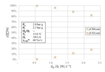
Figure 3.1 - Influence of biogas flowrate in open-loop configuration
