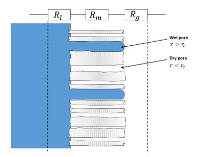
Figure 4.6 – Membrane porosity and membrane wetting modelling
