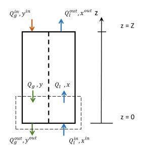
Figure 1.25- Counter-current absorption in a gas-liquid exchanger
