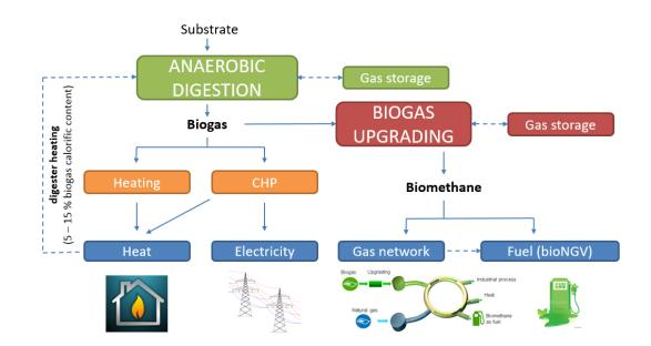
Figure 1.3 – Biogas applications in energy systems
