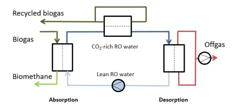
Figure 3.22 - Simplified closed-loop configuration with methane recycling loop 1:1:1
