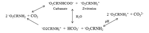
Figure 1.11 – Reaction scheme for CO<sub>2</sub> absorption in aqueous amine or amino acid salt solution [71]
