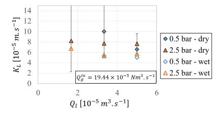
$\label{eq:KL} Figure \ 3.15-Variation \ of the overall mass transfer \ coefficient \ K_L \ with \ liquid \ flow rate \ for \ a \ constant \ inlet \ gas \ flow$
