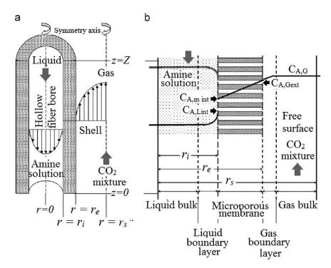
Figure 1.29– Schematic representation of the mass transfer domains in a hollow fiber membrane [205] *(a) velocity profiles of gas and liquid phases; (b) local concentration gradients*
