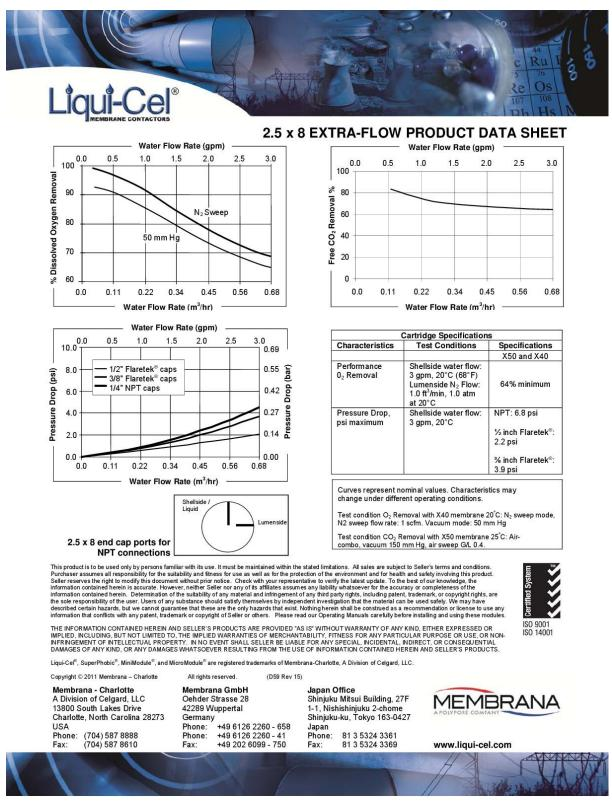
Figure H.1 – 2.5"x8" Extra-Flow module data sheet
