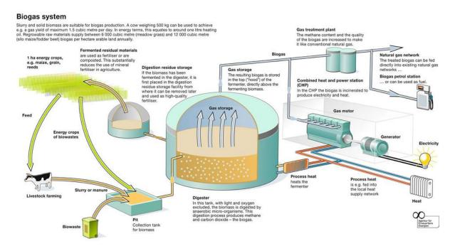
Figure 1.6 – Anaerobic digestion process (Source: Wheatleys)
