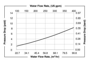
Curves represent nominal values, generated using water at 20°C. Test condition  $O_2$  Removal: X40 membrane,  $N_2$ -vacuum combo mode,
