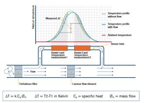
Figure 2.18– Principle of a thermal mass flowmeter [218]
