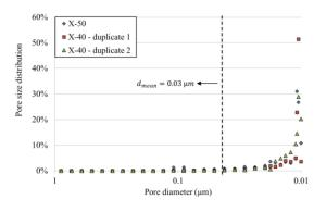
Figure 2.3– Pore size distribution results from Hg porosimetry
