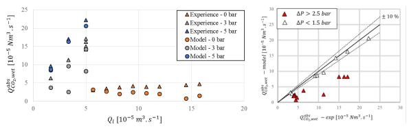
Figure 4.4 – Model validation in the membrane wet mode
