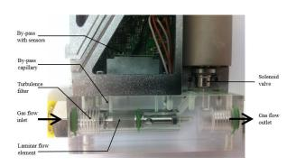
Figure 2.17 – Cross-sectional view of a thermal mass flow controller
