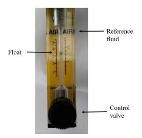
Figure 2.21 - Rotameter equipped with a control valve
