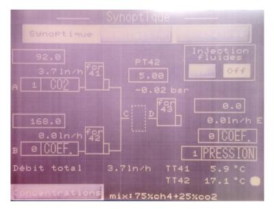
Figure 2.11 – Control interface of the gas chassis
