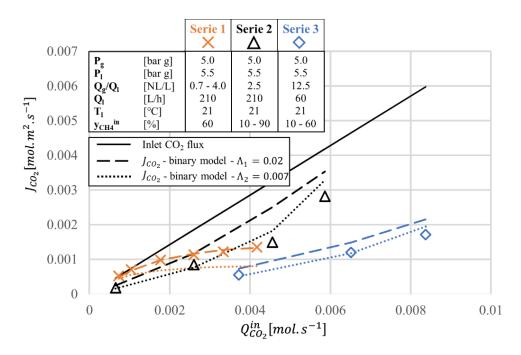
Figure 4.10 – Comparison of experimental absorbed CO<sub>2</sub> fluxes from a biogas mixture with numerical results from corrected model *Open-loop configuration*
