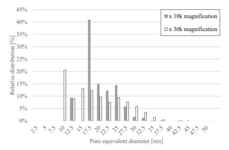
Figure 2.7 – Influence of SEM-FEG magnification on relative pore size distribution derived from image processing X-40 fibers – EHT=3.00 kV – WD=3.7mm – Diaphragm=30.00 μm
