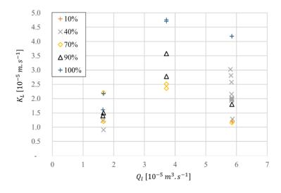
Figure 3.18 – Variation of the overall mass transfer coefficient according to the liquid flowrate and inlet CO<sub>2</sub> molar fraction - synthesis *Open-loop configuration*
