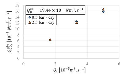
Figure 3.12 – Experimental absorbed CO<sub>2</sub> flow dependence on liquid flowrate at different transmembrane pressures in the dry mode for a constant inlet gas flow in the dry regime *Open-loop configuration – The transmembrane pressure*  $\Delta P$  *is specified in the legend*
