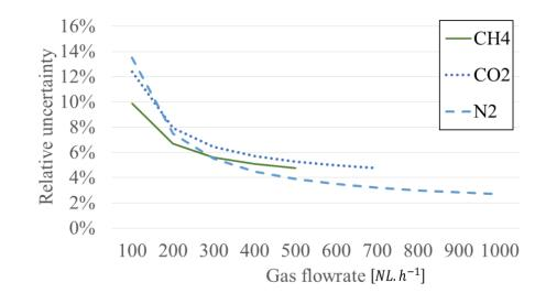
Figure 2.20 – Relative uncertainty according to gas component and gas flowrate in the In-Flow CTA flowmeters
