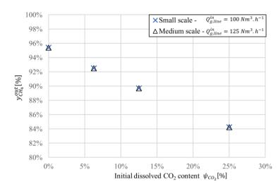
Figure 5.5 – Biomethane quality according the dissolved CO<sub>2</sub> content at the liquid inlet The large scale case is equivalent to the medium scale one
