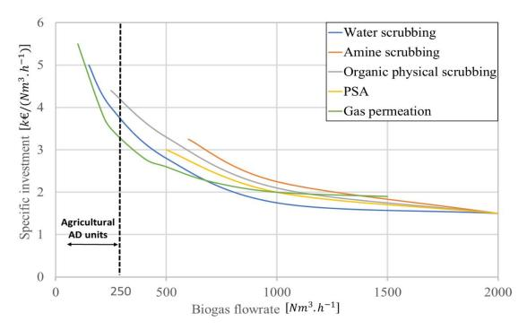
Figure 1.18 – Specific investment for a biogas upgrading unit according to the biogas flowrate [10]
