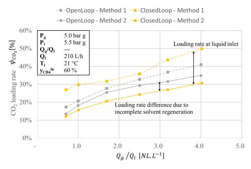
$\label{eq:Figure 3.8-Influence of $Q_g/Q_1$ ratio and process configuration on the $CO_2$ loading rate at the absorption liquid outlet$$
