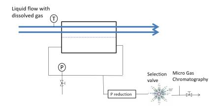
Figure N.1 - Dissolved gas analytical module set-up
