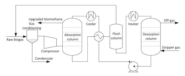
Figure 1.10 - Simplified flow diagram process of an organic solvent scrubber [58]
