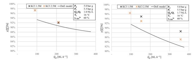
Figure 3.24 – Influence of mineral salt solution: biomethane quality according to inlet biogas flowrate  $Left: Q_g/Q_l = 1.0 NL. L^{-1} - Right: Q_g/Q_l = 1.7 NL. L^{-1}$
