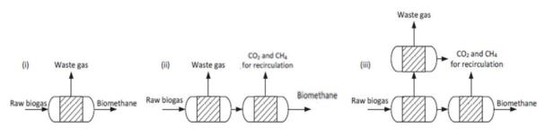
Figure 1.15 - Commercially available designs for membrane-based process [10]
