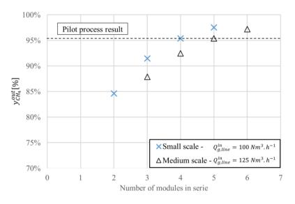
Simulations were then run for one process line in each case with an increasing number of modules (Figure 5.4).
