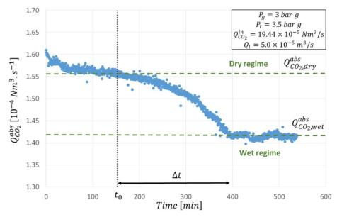
Figure 3.11 – Evolution of CO<sub>2</sub> absorbed flowrate over time *Open-loop configuration*
