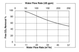
Curves represent nominal values using water. Characteristics may change under different operating conditions. Test condition  $O_2$  Removal with X40 membrane 20°C (68° F): N<sub>2</sub>-vacuum combo mode, vacuum: 50 mm Hg N<sub>2</sub> sweep flow 0.40 Nm<sup>3</sup>/hr (0.25 scfm). Test condition CO\_2 Removal with X50 membrane 25°C: Air-vacuum combo mode, vacuum 75 mm Hg, air sweep flow 1.6 Nm<sup>3</sup>/hr (1 scfm).
