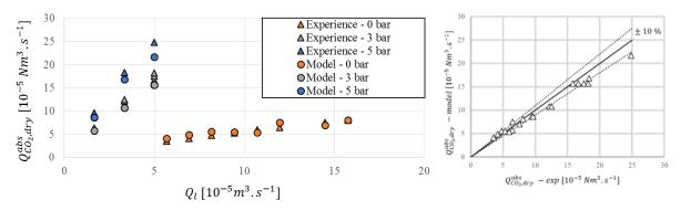
Figure 4.3 – Model validation in the membrane dry mode
