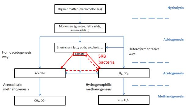
Figure 1.1 – Main steps of anaerobic digestion (adapted from [17])
