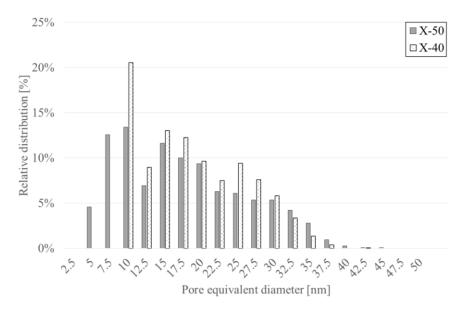
Figure 2.8 – Relative pore size distribution according to fiber type derived from image processing  $X 30k magnification - EHT=3.00 kV - WD=3.7mm - Diaphragm=30.00 \mu m$
