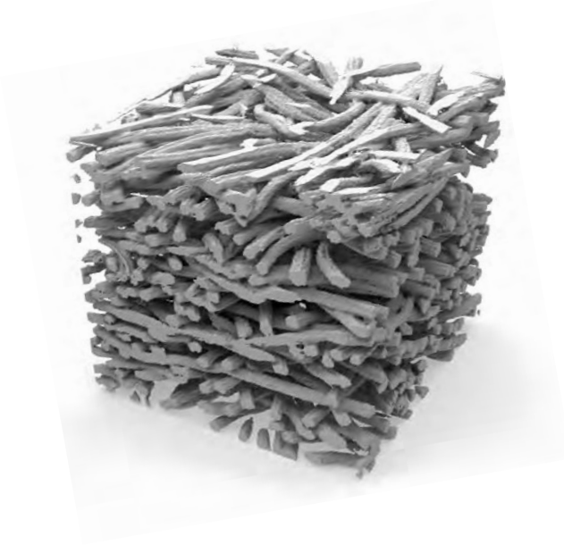
Figure 2.3: Volume rendering of a tomographic data set “0019” showing a fiber fleece. The visualized sub-volume consists of 512^3 out of 2048^3 pixels with a size of 0.65\ \mu\text{m} . The data were acquired by means of phase-contrast \mu\text{CT} using synchrotron radiation.
