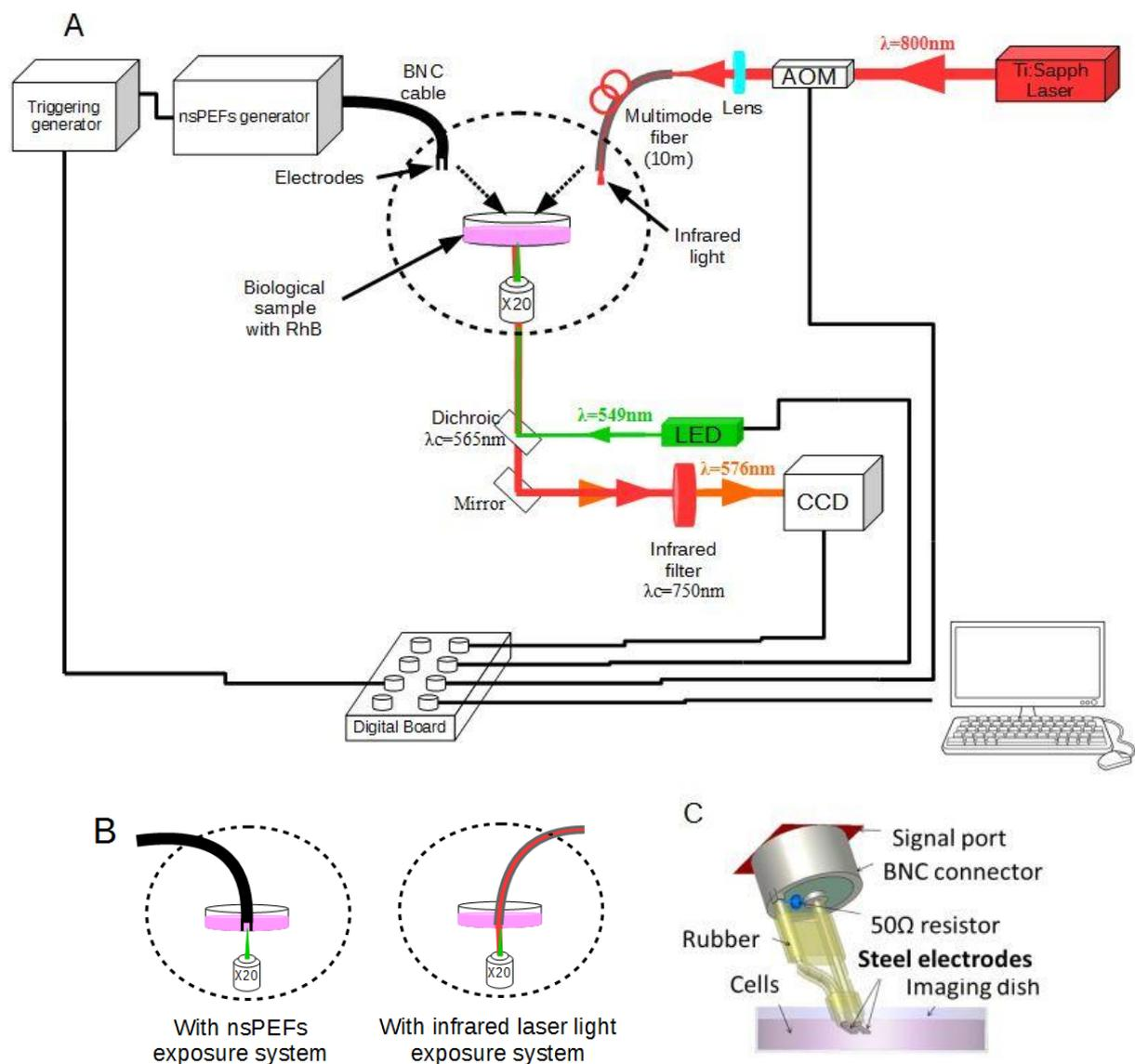
**Figure II-2** Experimental setup used for temperature measurement with RhB in cells exposed to infrared radiation and nsPEFs. A. General setup. B. A zoom on the petri dish. C. Schematic representation of the electrodes used to deliver nsPEFs.
