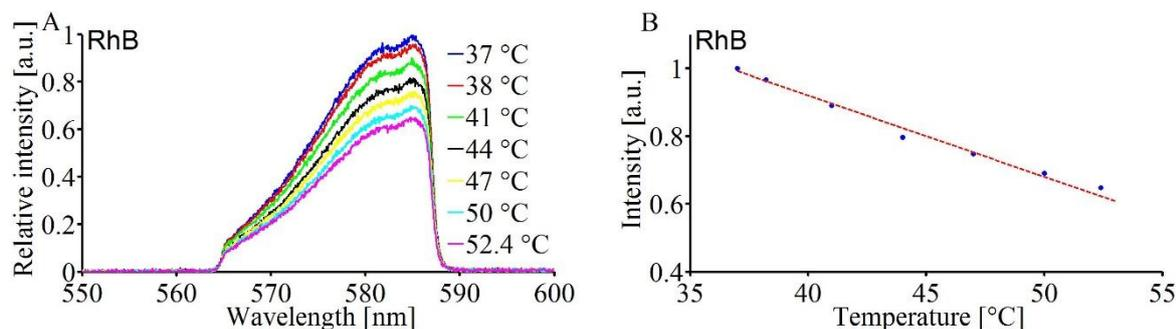
**Figure II-13** Calibration procedure made in water solution with RhB at 50  $\mu\text{M}$  by measuring RhB spectrum at different temperature. A. Evolution of the RhB fluorescence spectrum with the temperature. B. RhB relative intensity decreased of 2.4 %. $^{\circ}\text{C}^{-1}$  with 37  $^{\circ}\text{C}$  as reference temperature value.
