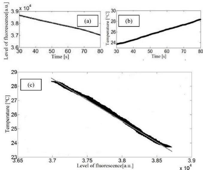
Fig. 2. (a), recording of the level of fluorescence versus time. (b), recording of the temperature with external thermometer versus time. (c), Conversion of fluorescence intensity into temperature. Results of measurement in black, linear fit in grey.
