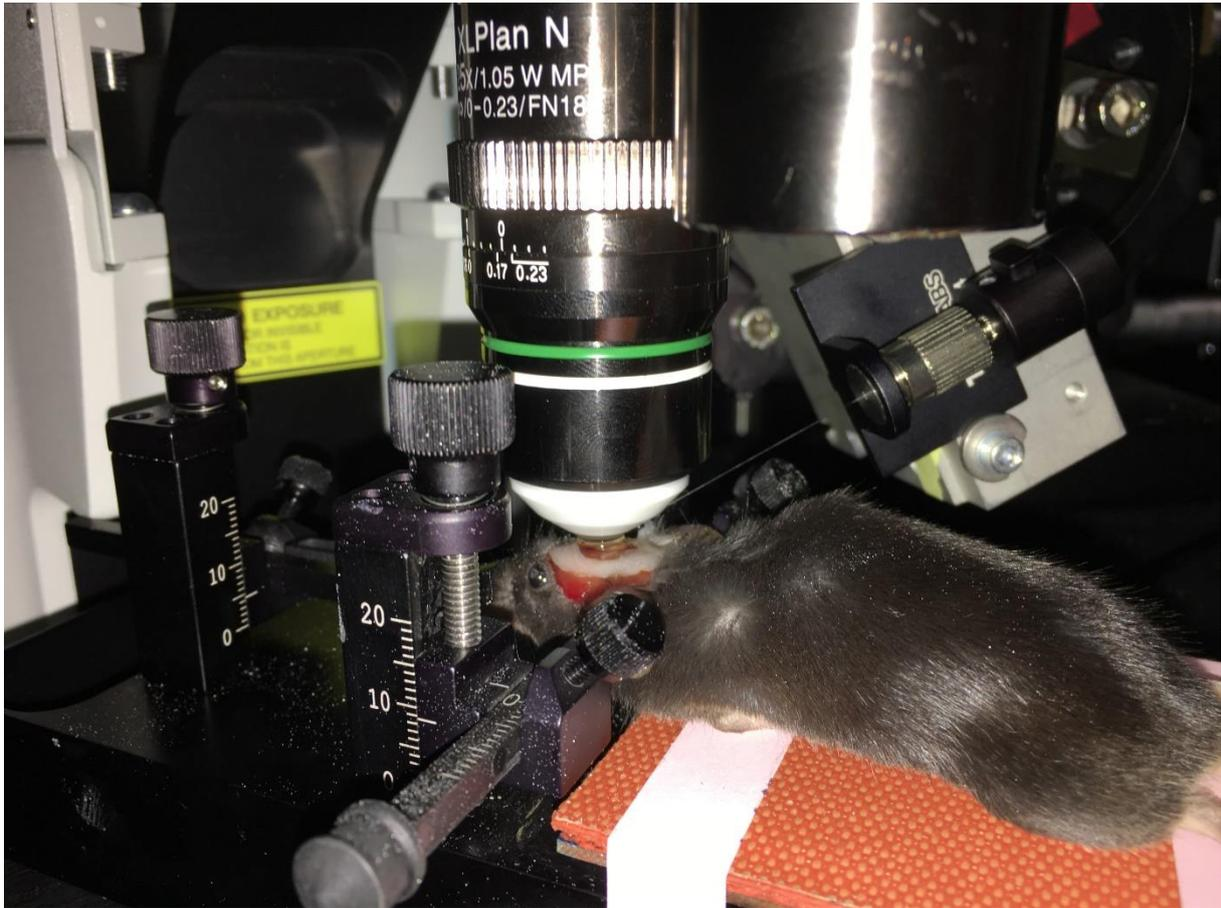
**Figure IV-6** Image of a part of the setup surrounding the mouse. It includes the 25X microscope objective, the micromanipulator allowing the positioning of the optical fiber and the mouse lying on a heating blanket.
