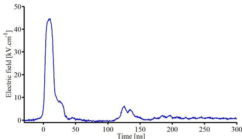
**Figure II-3** nsPEF shape recorded with an oscilloscope.
