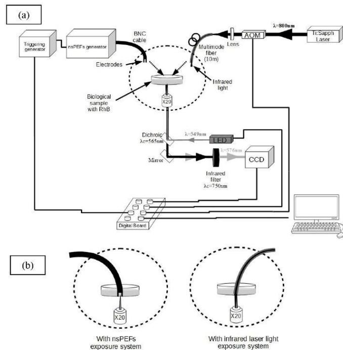
Fig. 1. (a). Experimental setup. (b). Zoom on the delivery of nsPEFs and infrared in the petri dish.
