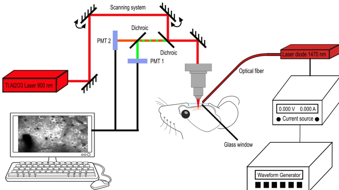
**Figure IV-5** Experimental setup.
