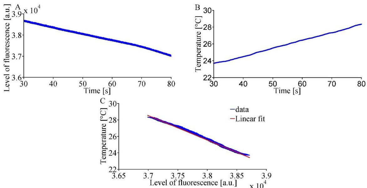
**Figure II-4** Calibration procedure made in water solution with RhB at 50  $\mu\text{M}$ . A. Evolution of the fluorescence intensity of RhB over time. B. Evolution of the temperature probed with Luxtron external thermometer over time. C. Relation between RhB fluorescence intensity and temperature.
