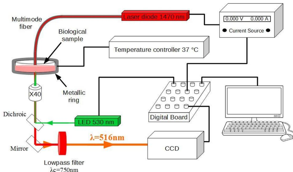
**Figure II-12** Experimental setup to make temperature measurements in cells exposed to 1470 nm radiation
