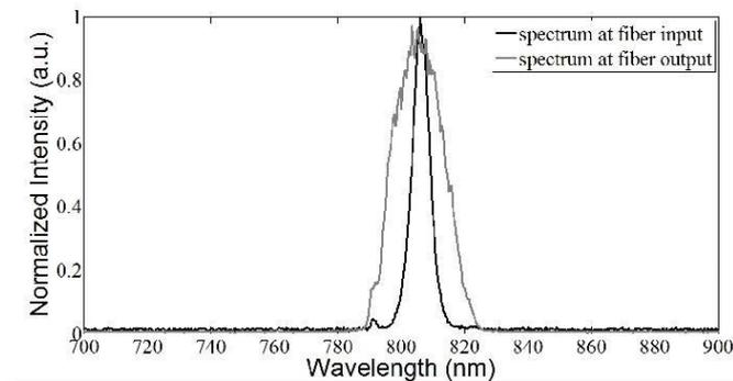
Fig. 3. Spectral broadening due to the fiber.
