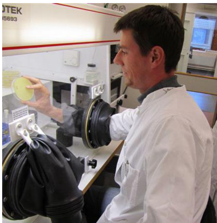
Figure 22. Glove box used for C. botulinum cultivation.
