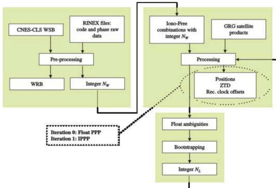
**Figure 3.5** – Integer ambiguity fixing that is applied at CNES-CLS IGS AC and implemented in GINS-PC. The terms WSB and WRB are wide-lane satellite bias and wide-lane receiver bias, respectively. Source: [Fund et al. 2013].
