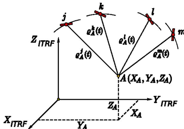
**Figure 3.3** – Principle idea of GPS-PPP configuration.  $X_A$ ,  $Y_A$  and  $Z_A$  are the cartesian coordinates of the GPS station. The small case latin letters  $j$ ,  $k$ ,  $l$  and  $m$  signify visible satellites at epoch. The greek letter  $\rho$  represents range measurements between the corresponding satellite and the geodetic site. The ITRF in the subscript shows the reference system. Source: Hofmann-Wellenhof and Moritz [2005].
