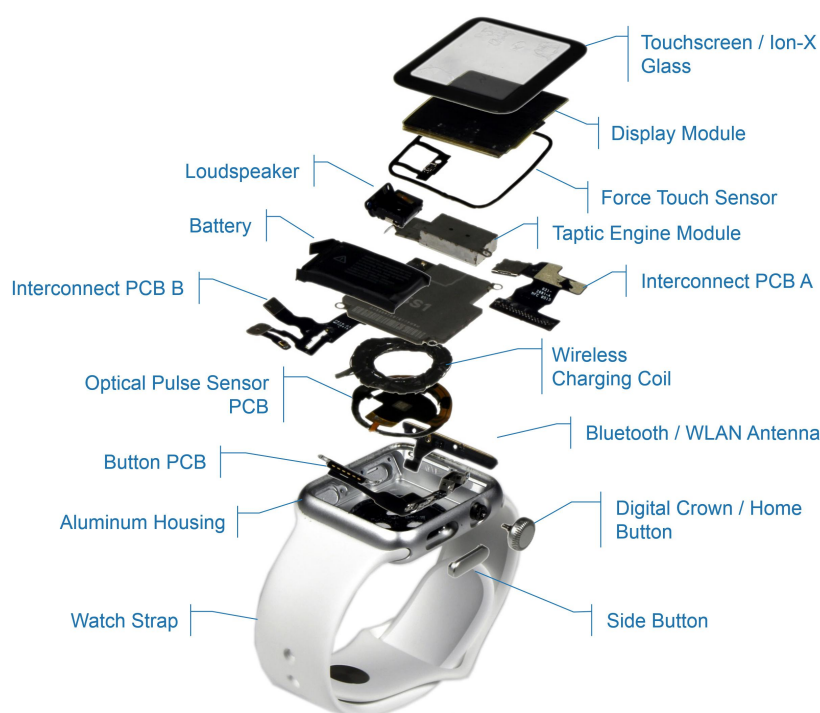
Figure 1.1: Exploded view of an Apple Watch, source from [1].
