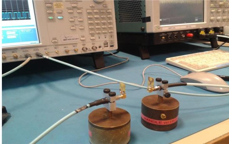
Figure 4.19 Setup with two monopole antennas placed face to face in short distance configuration.
