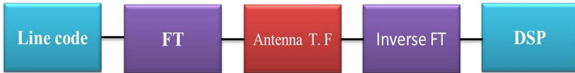
Figure 2.4 Procedure used to simulate the transmission of Polar RZ and Manchester line codes in the frequency domain with an antenna transmission transfer function. FT: Fourier Transform; T.F: Transfer Function; DSP: Digital Signal Processing.
