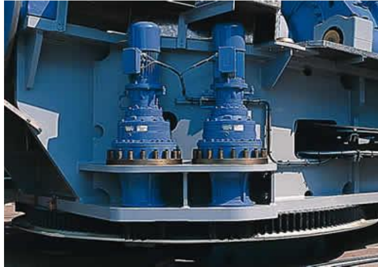
Figure 4.21. Yaw drive of a wind turbine
