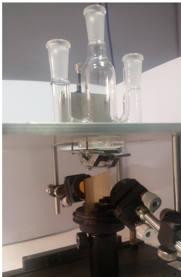
Figure 3.4 A picture of the SEIRAS setup. The incident IR beam is guided through a gold-coated glass slide to the gold coated mirrors which were directed to the ATR crystal with 60^\circ angles. Glass cell is mounted on the optical setup via metal holder stand.
