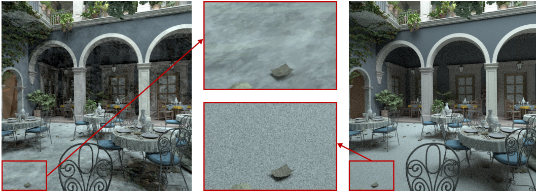
Figure 5.5: Left: coherent path tracing 128spp. Right: path tracing with Cranley Patterson rotation 128spp. Artifacts of coherent path tracing are induced by the re-utilization of the same sampling sequence for each pixel. The structured noise is more prominent on flat surfaces.
