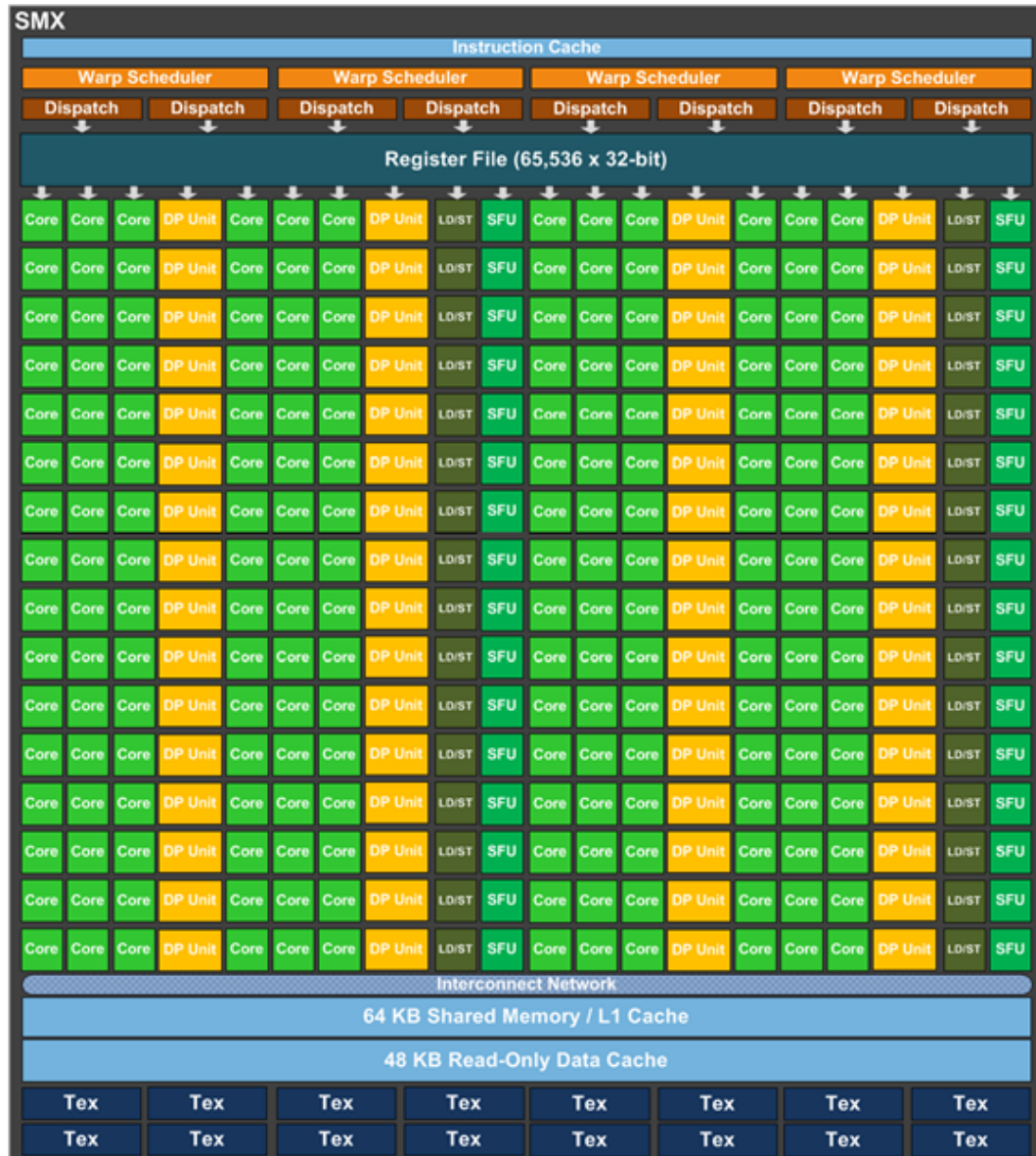
Figure 3.3: A detailed view of a Kepler SMX, courtesy of NVIDIA.
