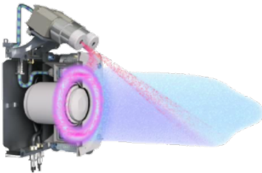
Figure 1.7 – Artist view of a standard HET operation with a side hollow cathode [15]: (dark blue) the xenon ions, (light blue) the neutral xenon, and (pink) the electrons, which are either trapped by the magnetic field inside the channel or neutralizing the expelled xenon ions.
