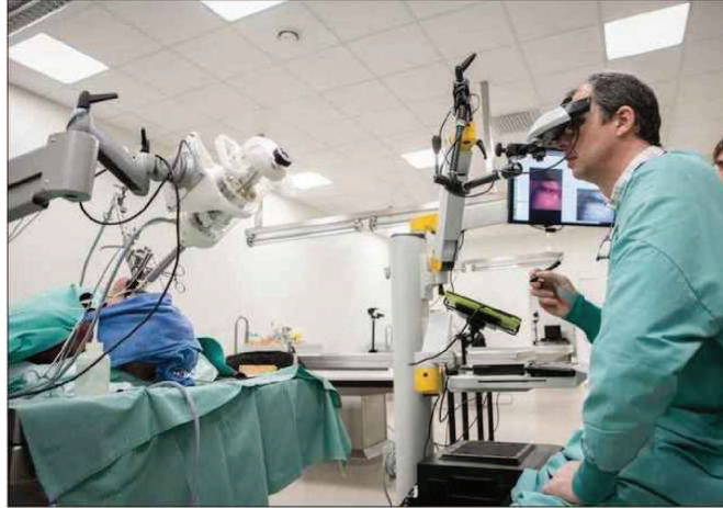
FIGURE 1.8: Surgeon Tavernier drawing on a tactile tablet the laser path using the new concept of \mu RALP.
