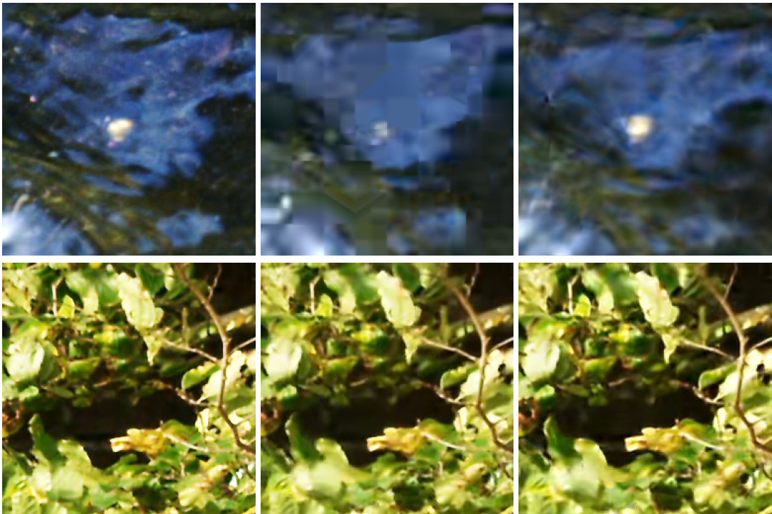
Figure 3.3 – Examples of visual comparison between default compression and proposed method in [9]. Left: original frames, middle: compressed frames with HEVC and right: synthesized frames at the decoder side.
