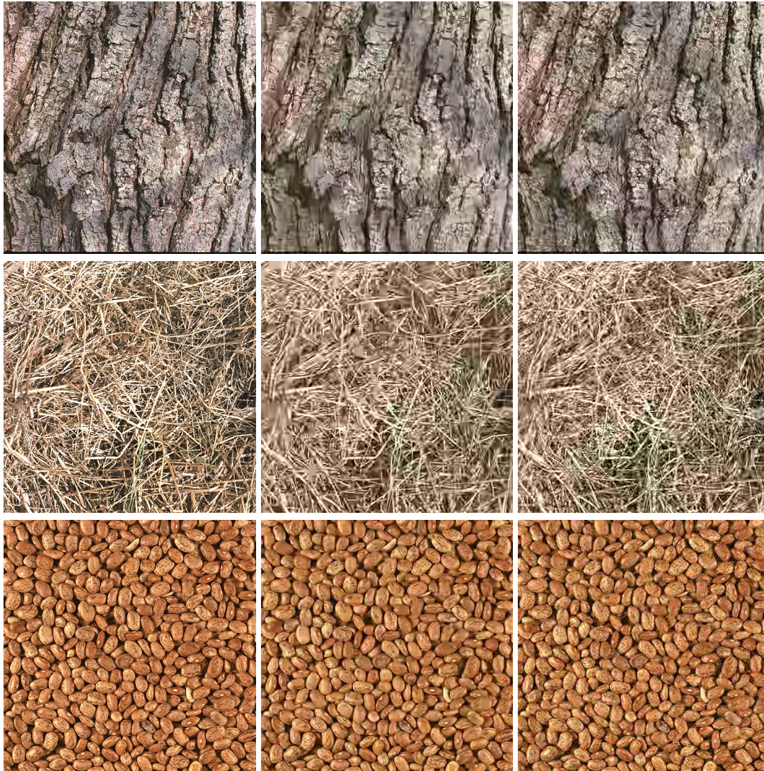
Figure 7.10 – Examples of decoded textures using the same QP. From left to right: Original texture, compressed using HEVC default metrics and using STSIM.
