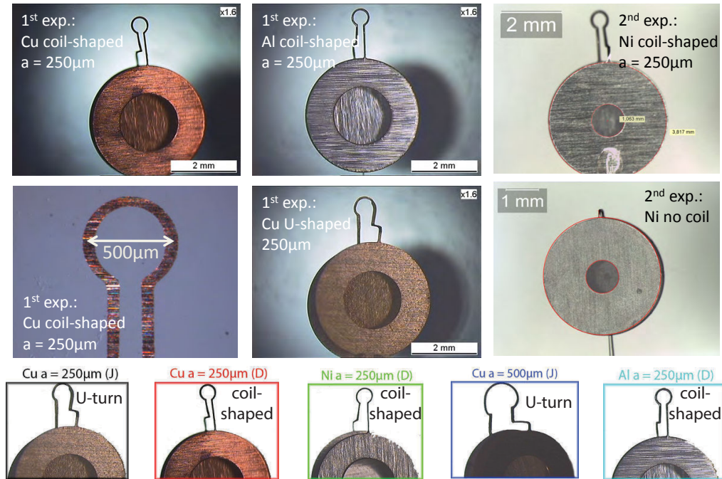
Figure 8.2 – Photographs of capacitor-coil target samples.
