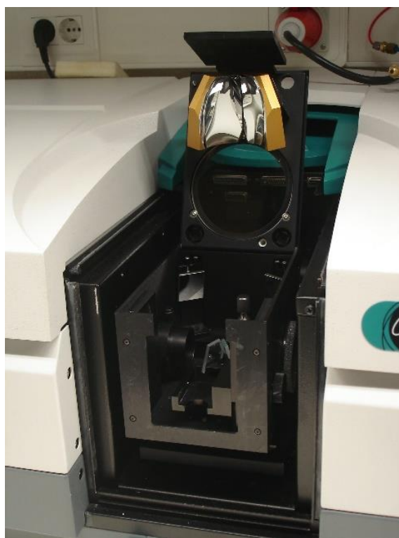
Figure C-2 – Picture of Praying Mantis accessory coupled in Varian Cary 5000 UV-Vis-NIR spectrophotometer available at CATHPRO/CQE (IST, Lisbon).
