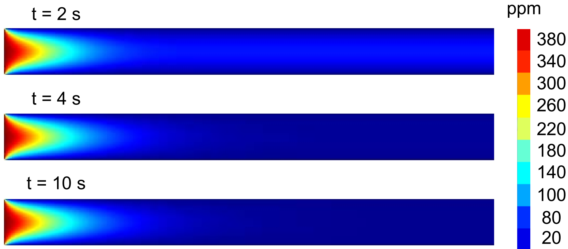
Figure V-13 – Simulation results for NO concentration profile over the first 10 mm of a single channel of base-600 monolith.
