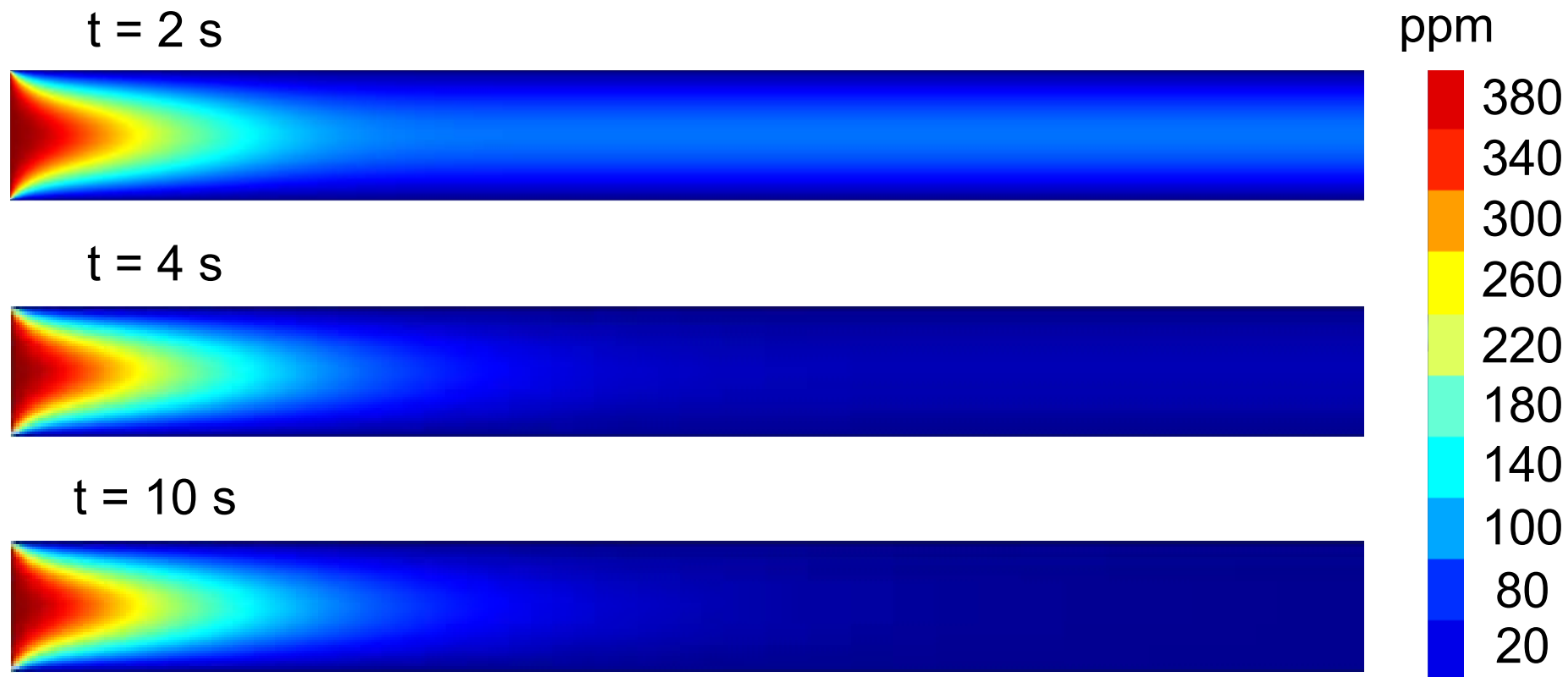
Figure V-12 – Simulation results for NO concentration profile over the first 10 mm of a single channel of base-400 monolith.
