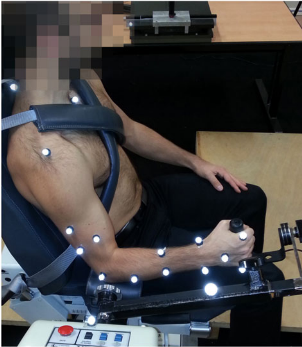
Figure 1. Experimental set-up during a maximal isometric joint torque measurement of the elbow flexion.
