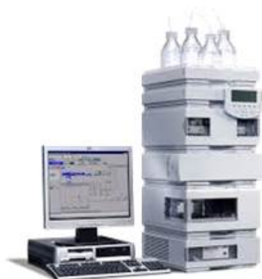
FIG. II.8 – Agilent 1100 series HPLC system.
