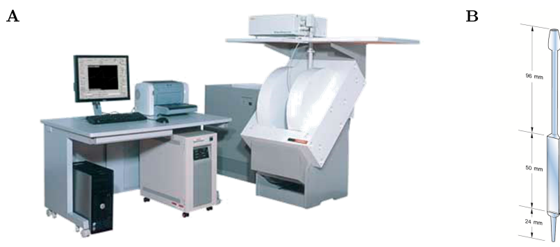
FIG. II.6 – (A) JEOL FA – 300 series ESR spectrometer and (B) JEOL quartz flat cell.
