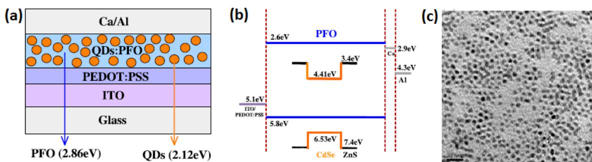
**Figure 1.2:** A schematic of a single layer device structure that shows CdSe/ZnS QDs embedded in a PFO layer sandwiched between ITO and Ca/Al electrodes. Arrows indicate the EL energy peaks of the QDs and PFO (a). Energy level diagram of the device, where all indicated energies are with respect to the vacuum level (b). HR-TEM of 80 wt% QD embedded in PFO (c). The figures are taken from [59].
