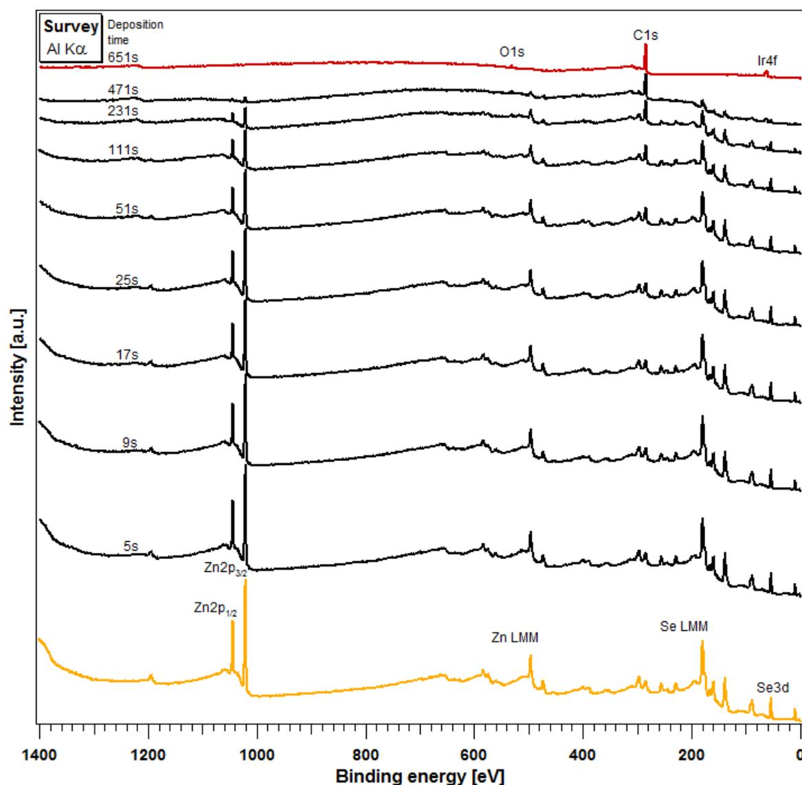
**Figure 5.4:** Survey spectra of ZnSe and the step-wise deposited Ir(BPA) in the interface experiment for a ZnSe/Ir(BPA) bilayer. The total times for each of the Ir(BPA) deposition steps are indicated.
