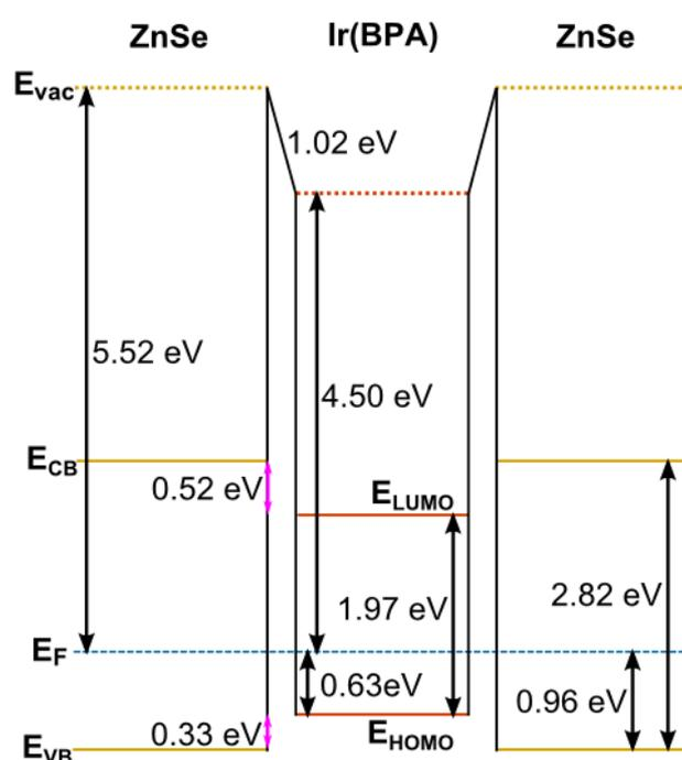
**Figure 5.19:** Energy band alignment at the internal interfaces of the 19% ZnSe+Ir(BPA) composite. This band diagram displays the dye frontier orbitals being sandwiched by the ZnSe energy levels. The difference in the measured  $\phi$  of the pristine ZnSe and the calculated  $\phi$  of the dye in the composite is assigned to a 1.02 eV interface dipole that leads to the measured lineup.
