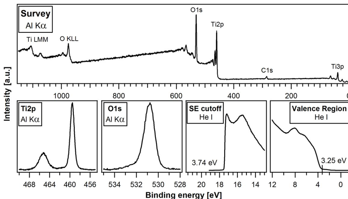
**Figure E.1:** Survey spectrum and detailed spectra of the Ti2p and O1s emissions from the pristine nc-TiO<sub>2</sub> layer, together with the spectra of the SE cutoff and valence region.
