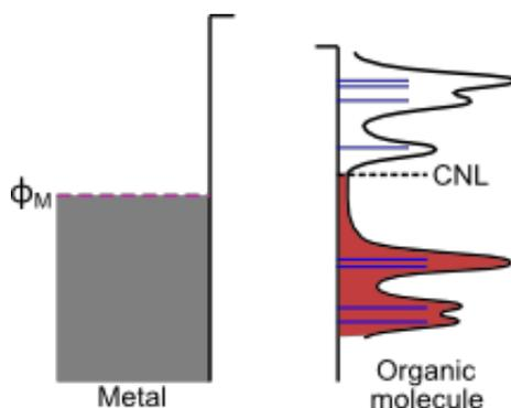
**Figure 2.22:** At weakly interacting metal/organic interfaces, charge transfer tends to align the organic CNL and metal work function. This gives rise to an induced dipole at the interface and to the partial pinning of the Fermi level in the organic energy gap.
