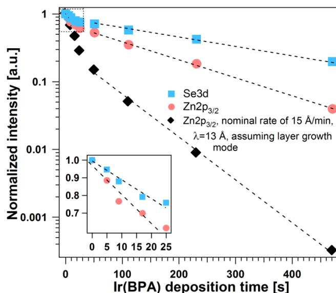
**Figure 5.6:** Normalized integrated Zn2p<sub>3/2</sub> and Se3d emission intensities versus Ir(BPA) deposition time. Below 25 s the damping increases linearly (shown in the inset), indicating growth of a monolayer. Above 25 s the damping is exponential, indicating layer-by-layer or island growth. In addition, the calculated damping of Zn2p<sub>3/2</sub> emission is shown for a layer-by-layer growth considering a nominal deposition rate of 15 Å/min and a photoelectron escape depth of 13 Å.
