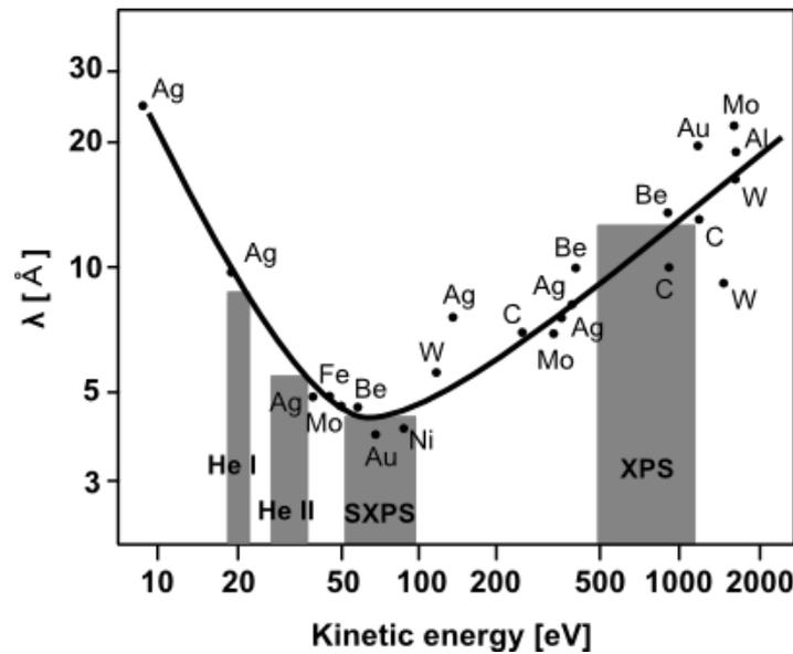
**Figure 3.1:** The inelastic mean free path  $\lambda$  of emitted photoelectrons as a function of their kinetic energies  $E_{kin}$ . Typical kinetic energy ranges resulting from specific photon sources are indicated.
