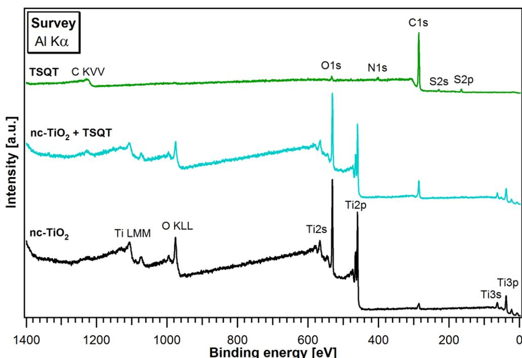
**Figure 9.8:** Survey spectra of pristine nc-TiO<sub>2</sub>, drop-casted TSQT on the nc-TiO<sub>2</sub>, and pristine TSQT. The C1s peak in the spectrum of the nc-TiO<sub>2</sub> indicates the presence of residual carbon contamination that was not fully eliminated by the cleaning procedure.
