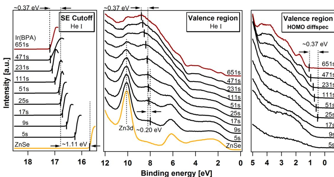
**Figure 5.7:** Secondary electron cutoff and valence region spectra during the stepwise deposition of Ir(BPA) on ZnSe. The Ir(BPA) deposition times are indicated. A distinct Ir(BPA) valence feature at  $\sim 8.80$  eV is marked in the valence spectra. During monolayer growth,  $\phi$  decreases strongly by about 1.11 eV while the dye features shift by 0.20 eV to lower binding energy. Then the SE and the dye features shift by an additional 0.37 eV.
