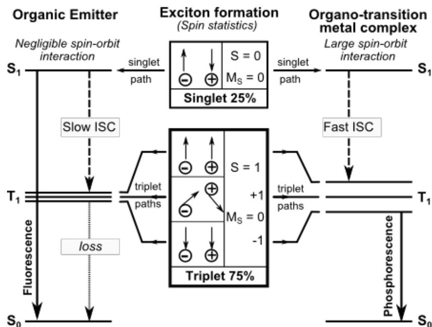
**Figure 2.14:** Singlet and triplet harvesting in the electroluminescence excitation processes for organic and organo-transition metal emitters. Modified from [96].
