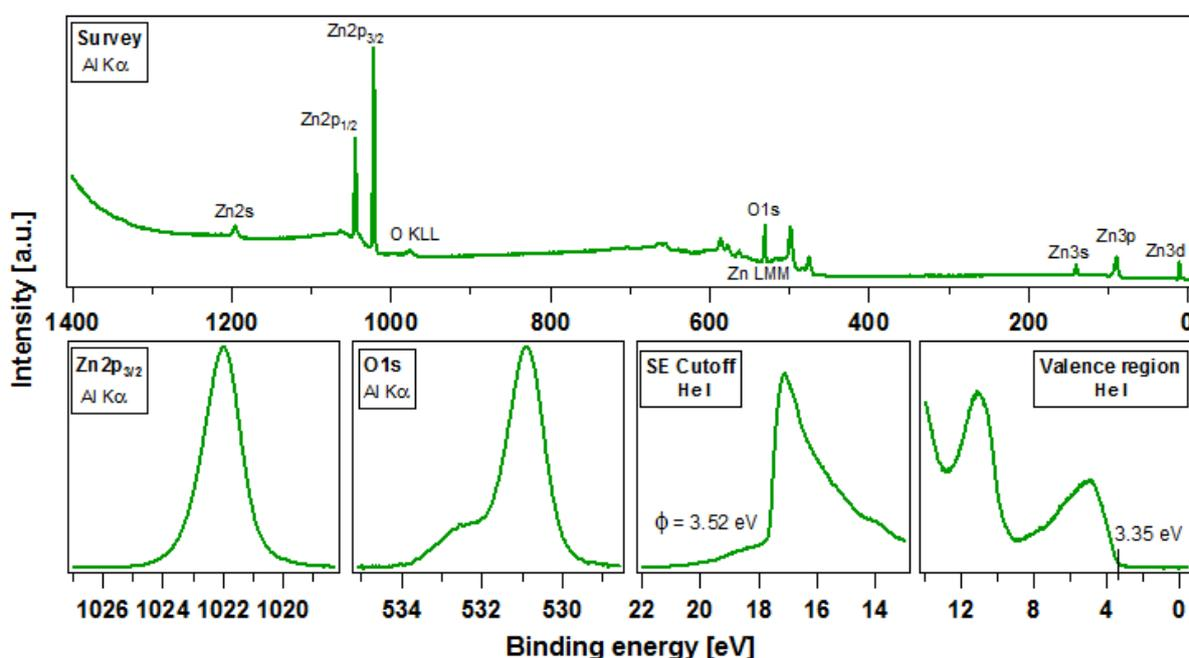
**Figure 8.6:** A survey spectrum showing all the peak photoemissions that are representative of the elemental composition of the as-deposited ZnO film on ITO glass substrate, together with the detailed spectra of Zn2p<sub>3/2</sub>, O1s, SE cutoff region and the valence band. From the SE cutoff,  $\phi$  is determined to be 3.52 eV. The VBM is located at 3.35 eV from the Fermi level.
