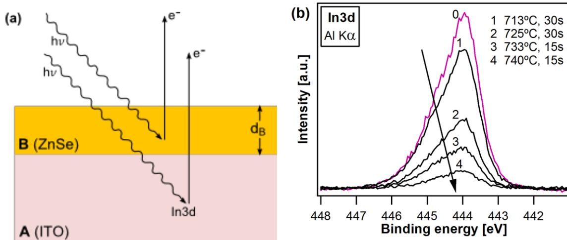
**Figure B.1:** (a) Schematic geometry for a layer model in obtaining layer thickness. The substrate is ITO on glass and the overlayer is ZnSe with a thickness of  $d_B$ . (b) Attenuation of the ITO In3d emission upon the step-wise deposition of ZnSe.
