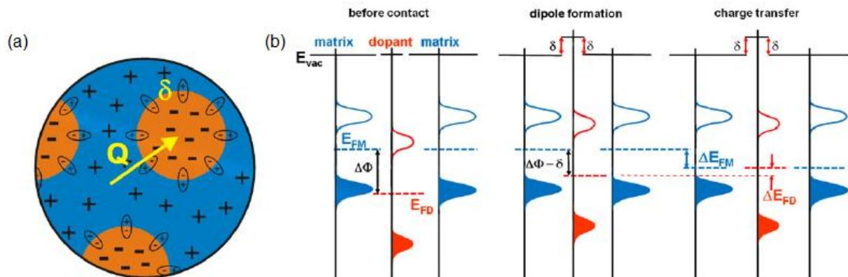
**Figure 2.23:** (a) Sketch of a composite material comprising of an organic matrix (in blue) and clusters of dopant molecules (in orange). p-type doping is also illustrated. (b) Development of the energy band diagram according to the internal interface charge transfer model. Taken from [146].
