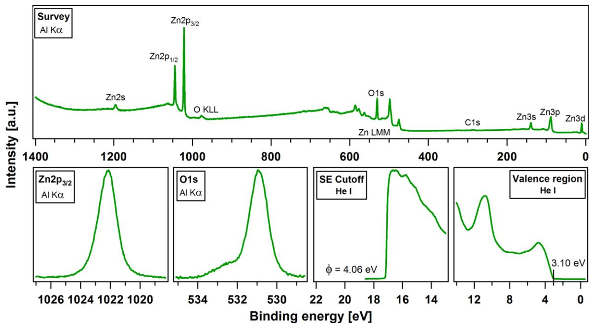
**Figure 8.7:** A survey spectrum showing all the peak photoemissions that are representative of the elemental composition of the annealed ZnO film deposited on ITO glass substrate, together with the detailed spectra of Zn2p<sub>3/2</sub>, O1s, SE cutoff region and the valence region. From the SE cutoff,  $\phi$  is determined to be 4.06 eV. The VBM is at 3.10 eV from the Fermi level.
