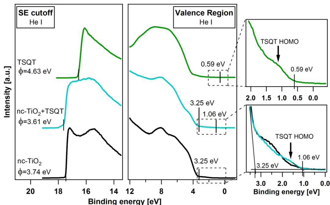
**Figure 9.10:** SE cutoff and valence region spectra of the pristine nc-TiO<sub>2</sub>, nc-TiO<sub>2</sub> + TSQT composite and pristine TSQT layers. The spectra on the right side are enlarged versions of the boxed regions in the valence region spectra.
