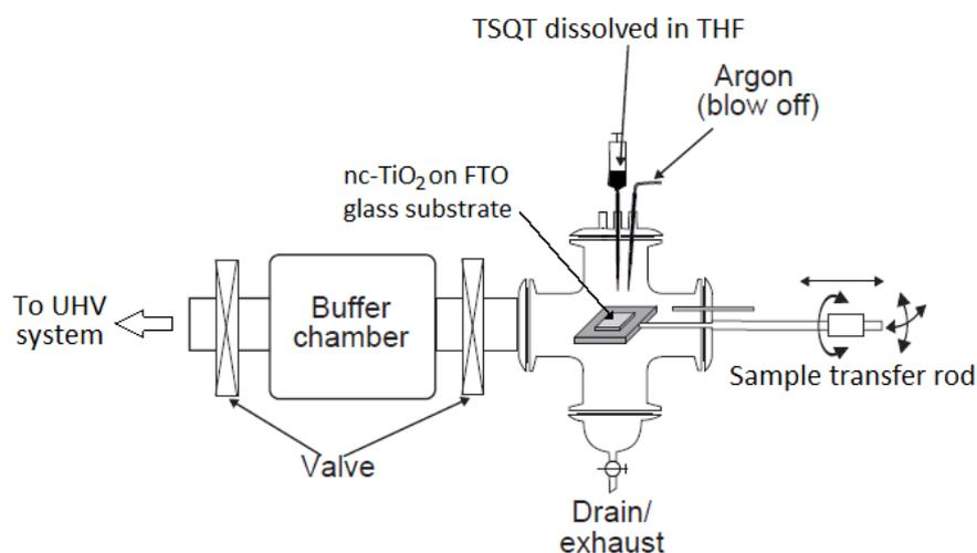
**Figure 9.6:** Glass cell for solution-based deposition of TSQT on nc-TiO<sub>2</sub>.
