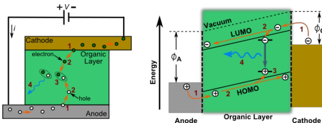
**Figure 2.3:** OLED basic working principle. An organic layer is sandwiched between a transparent conductive oxide as anode and a low-work function metal as cathode. Four steps of the light generation process in an OLED: (1) charge injection, (2) charge carrier transport, (3) exciton formation and (4) exciton recombination.
