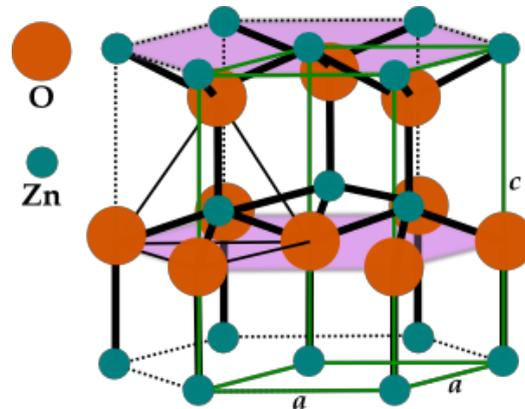
Figure 8.1: Hexagonal wurtzite structure of a ZnO crystal.
