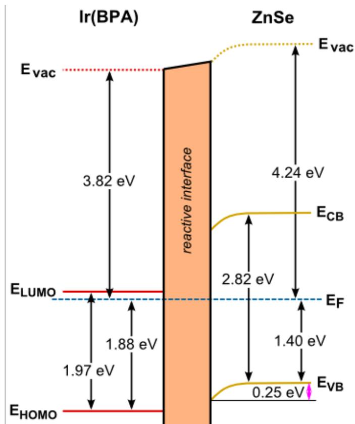
**Figure 5.15:** Energy band alignment for the Ir(BPA)/ZnSe heterojunction where only depositions up to 17 s is considered for the Ir(BPA) layer and depositions starting from 37 s is considered for the ZnSe layer. The deposition of ZnSe on top of Ir(BPA) leads to an interface region where the two materials are reactive (i.e. intercalation of Zn atoms into the immediate Ir(BPA) layer; formation of mixed phases of ZnSe, Se<sup>0</sup> and reduced Se; oxidation of Ir(BPA) molecules).
