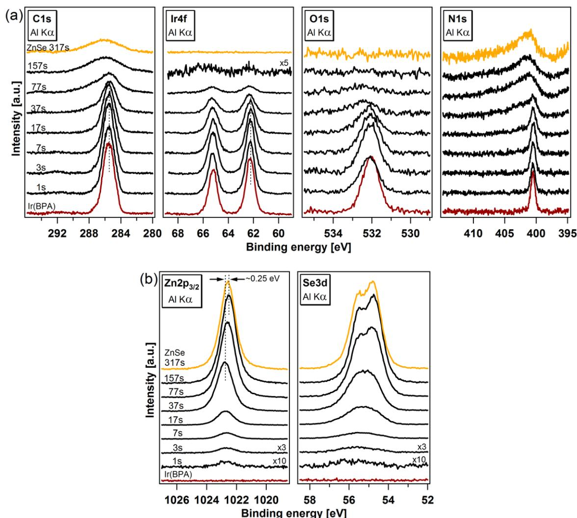
**Figure 5.12:** Ir(BPA) C1s, Ir4f, O1s and N1s emission spectra (a), ZnSe Zn2p<sub>3/2</sub> and Se3d emission spectra (b) during the stepwise deposition of ZnSe on an Ir(BPA) film. The ZnSe deposition times are indicated. While the dye's C1s and Ir4f binding energies remain constant with increasing overlayer coverage, the Zn2p<sub>3/2</sub> and Se3d emissions shift to lower binding energies approaching that of pristine ZnSe.
