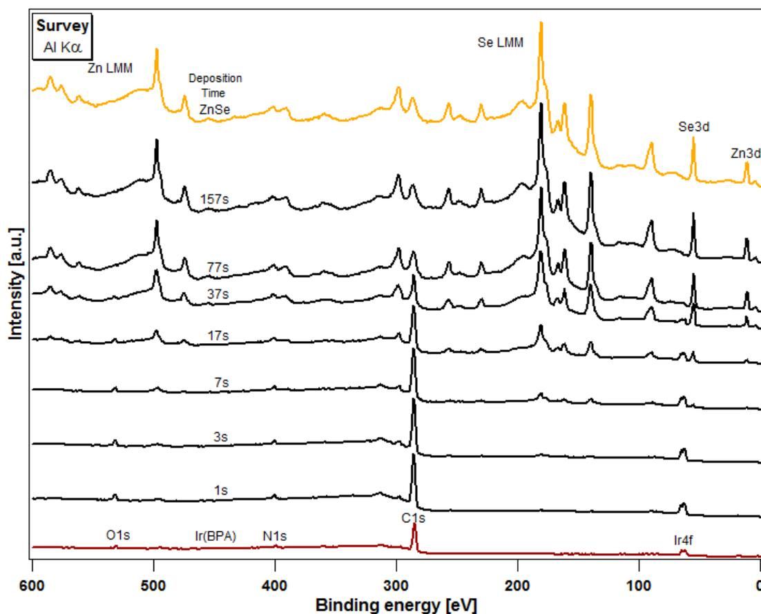
**Figure 5.10:** Survey spectra of Ir(BPA) and the step-wise deposited Ir(BPA) in the interface experiment for a ZnSe/Ir(BPA) bilayer. The total times for each of the Ir(BPA) deposition steps are indicated.
