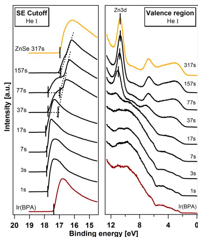
**Figure 5.11:** Photoemission spectra of the secondary electron cutoff and the valence region for ZnSe deposition onto the Ir(BPA) layer. The ZnSe deposition times are indicated. At the 37 s deposition step, the SE cutoff starts to exhibit a double edge structure and the valence region shows a sudden increase of Zn3d and the appearance of ZnSe valence features.
