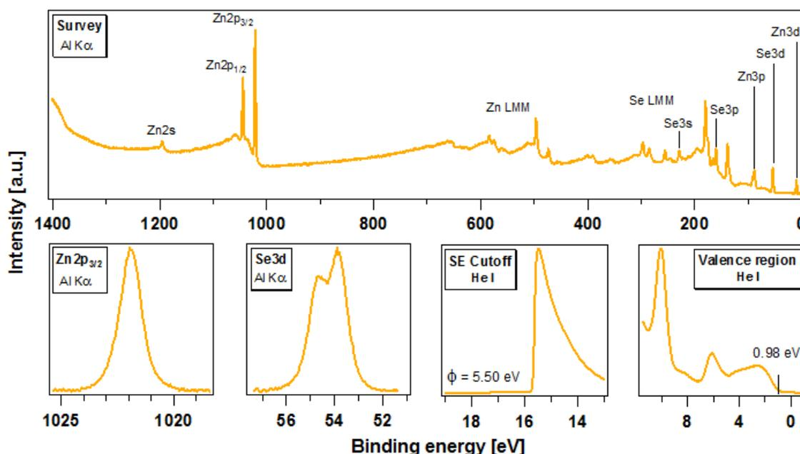
**Figure 5.1:** Survey spectrum, Zn $2p_{3/2}$  and Se3d detailed spectra, SE cutoff and valence region spectra of the ZnSe layer. No contamination is evident. The features found in the valence band spectrum are representative of that of ZnSe.
