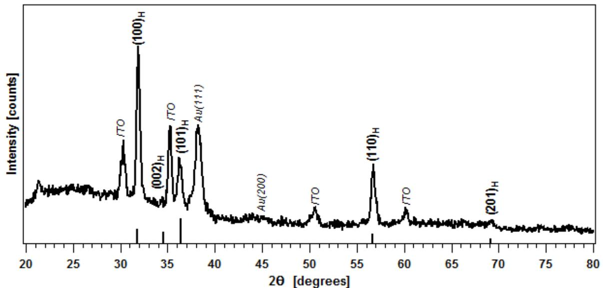
Figure 8.2: XRD spectra of a ZnO film deposited on ITO glass substrate along with bar markings on the x-axis for ZnO reflection peaks from the JCPDS<sup>55</sup> database.
