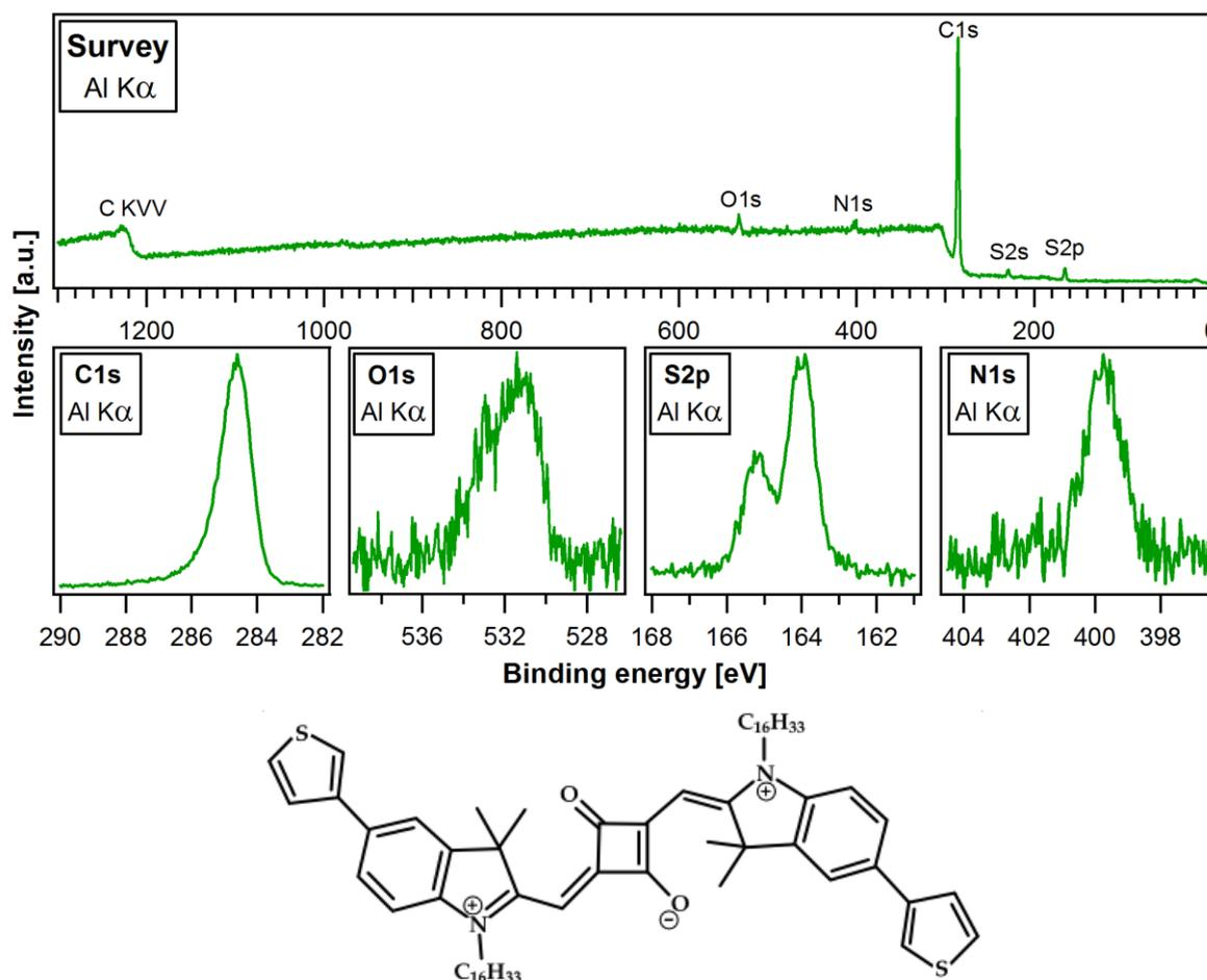
**Figure E.2:** Survey spectrum and detailed spectra of the C1s, O1s, S2p and N1s core line emissions from the pristine TSQT film drop-casted on an ITO glass substrate. The chemical structure of the dye is also shown.
