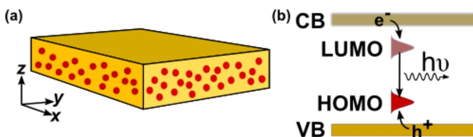
**Figure 1.5:** Schematic representation of the proposed bulk composite as an electroluminescent active layer for HLEDs comprising of an inorganic semiconductor matrix doped with organic small molecules (a) and the corresponding designated energy level diagram for direct electron/hole transfer from the inorganic wide bandgap semiconductor matrix to the dopants with subsequent radiative emission from the dopants (b).
