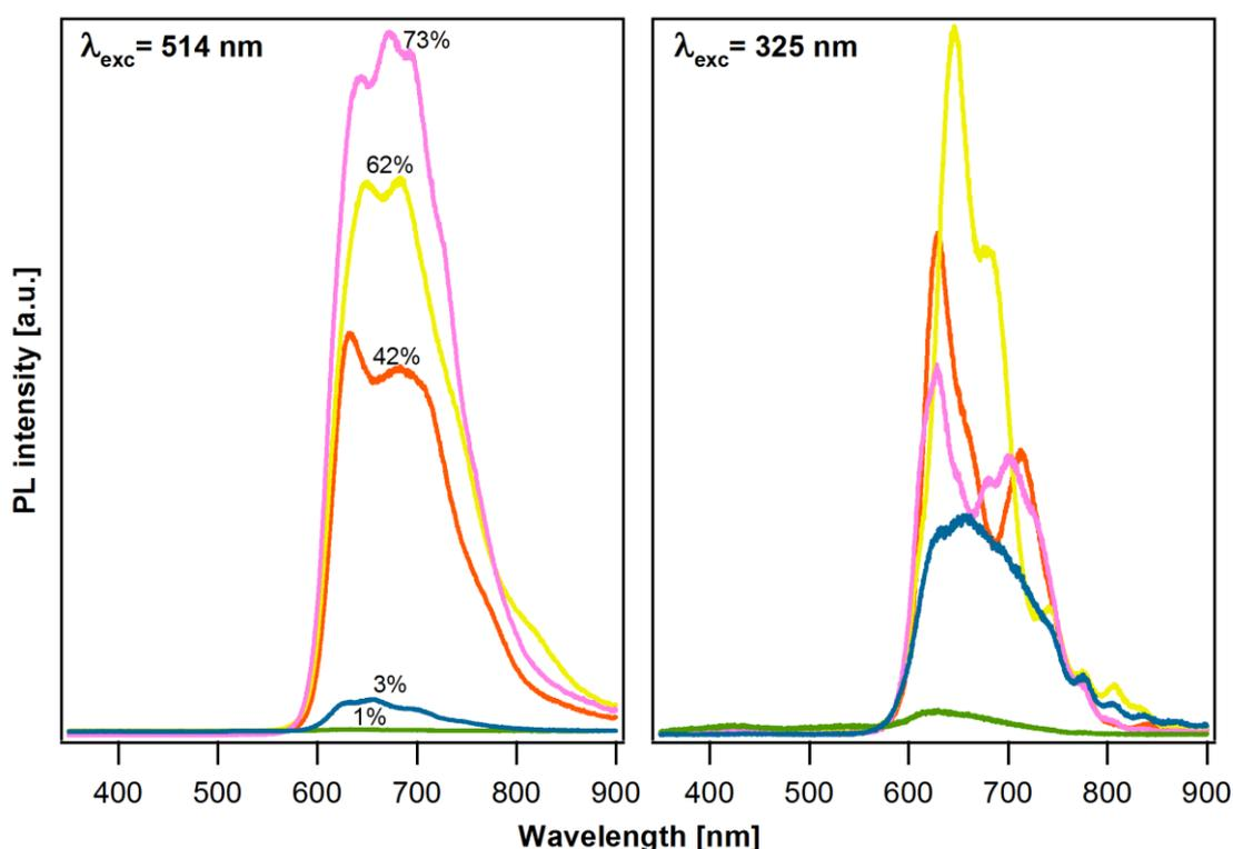
**Figure 6.14:** Superimposed PL spectra of the composites under the 514 nm and 325 nm laser excitation. Under the 325 nm UV laser excitation, the luminescence of the dye in the 1% and 3% composites is enhanced relative to the luminescence of the composites with the large dye content.
