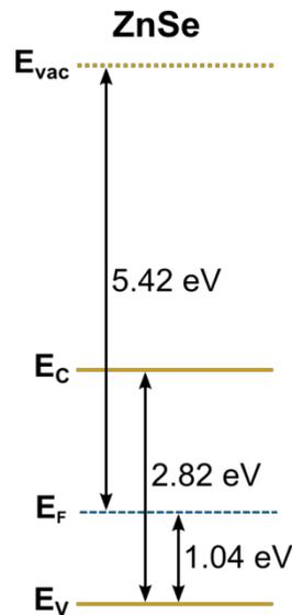
**Figure 4.3:** Energy levels of ZnSe as deduced from the UPS measurement:  $\phi = 5.42$  eV and VBM at 1.04 eV. The energy gap is taken from transmittance measurements (found in the succeeding sections).
