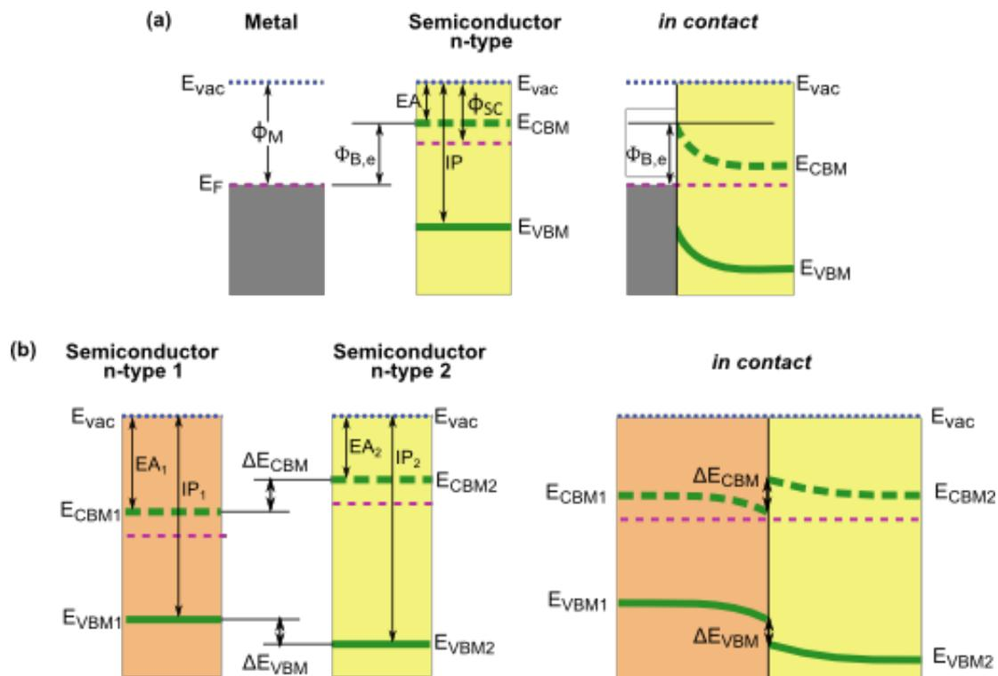
**Figure 2.20:** (a) Schottky-Mott model that describes the construction of the metal-semiconductor junction energy band diagram. (b) Anderson's rule that describes the construction of the heterojunction between two semiconductor materials.
