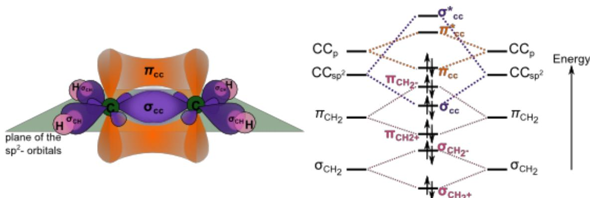
**Figure 2.6:** Orbital structure of ethylene ( $C_2H_4$ ). End-to-end overlap of  $sp^2$  orbitals results to a  $\sigma$  bond between the two carbon atoms, while side-to-side overlap of p orbitals result to a  $\pi$  bond.
