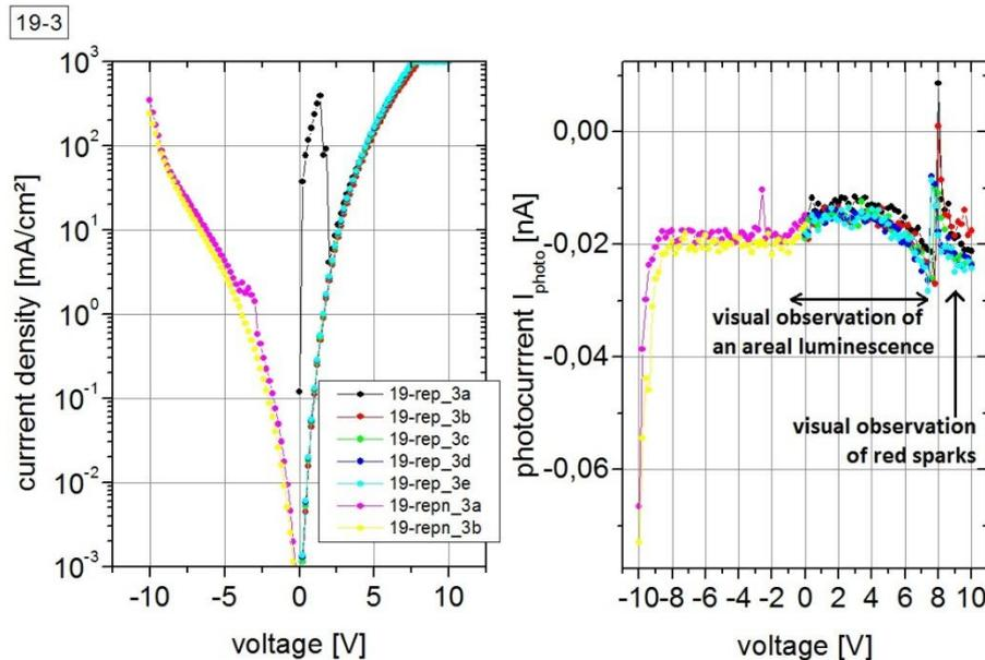
**Figure 7.8:** Current density versus applied (reverse and forward) voltage for Device 19-3. The photocurrents generated on a silicon photodiode against the applied voltage on the device are plotted here as well.
