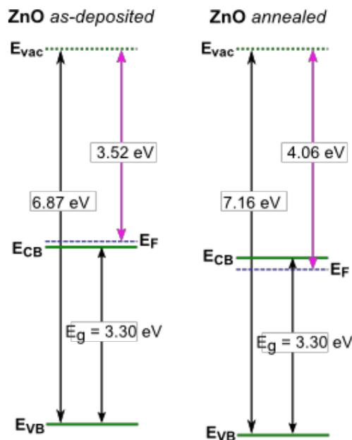
**Figure 8.8:** Energy levels of the as-deposited and annealed ZnO as deduced from the UPS measurements. The 3.30 eV energy gap is taken from the optical transmission measurement. The ionization potential and the work function of ZnO increased when annealed, approaching literature values.
