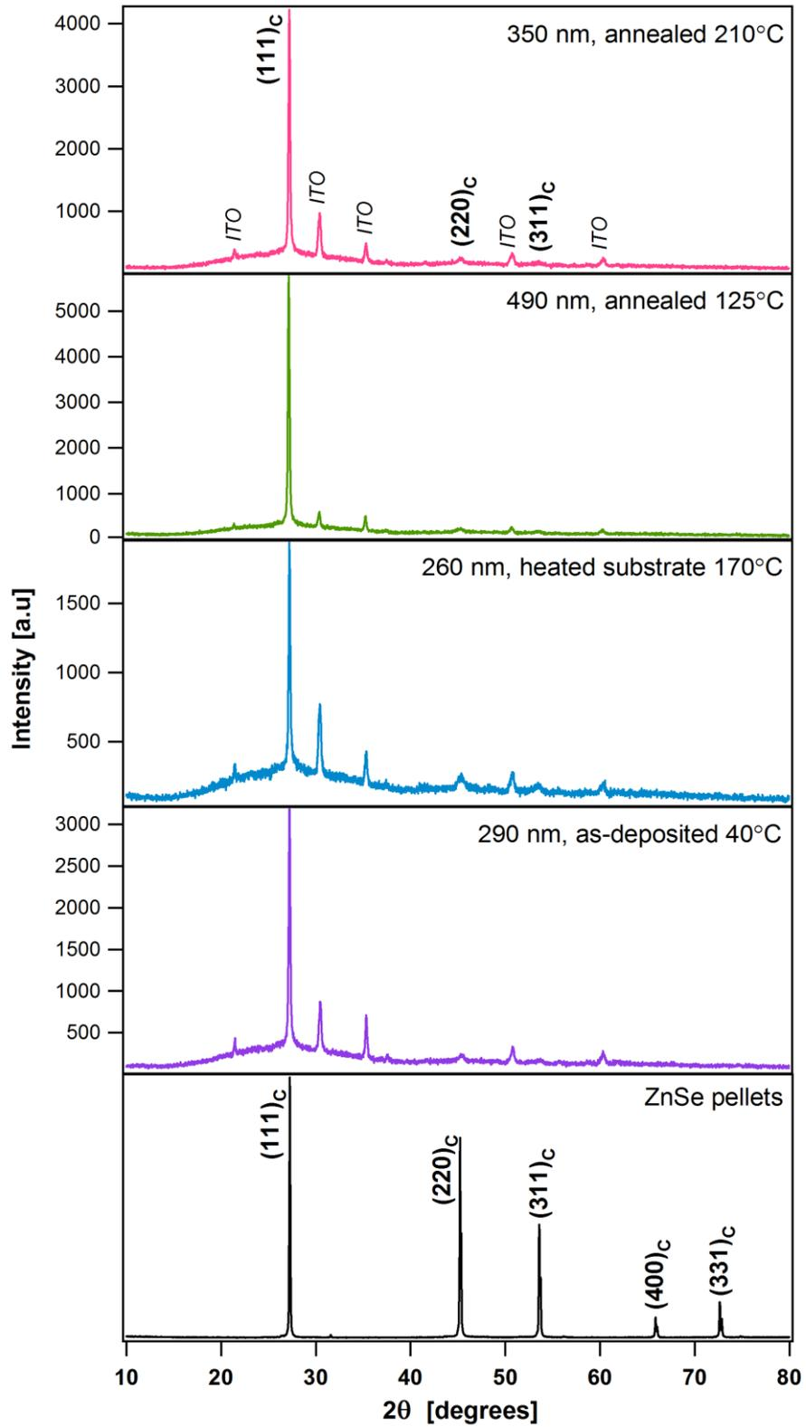
**Figure 4.8:** XRD patterns from as-deposited, heated-substrate and annealed ZnSe thin films together with the pattern from pulverized ZnSe pellets.
