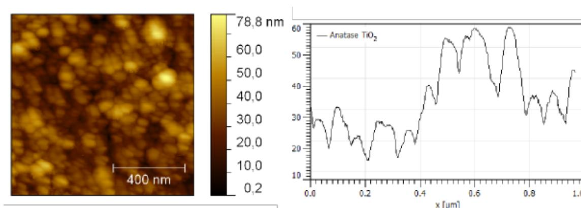
**Figure 9.3:** AFM image of the anatase nc-TiO<sub>2</sub> film with an average particle size of ~20 nm. The height profile reveals a surface that is not flat.
