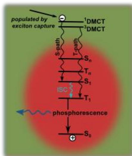
**Figure 2.16:** Alternative energy level scheme for the emitter dopant with its immediate surrounding matrix molecules.  $^1\text{DMCT}$  and  $^3\text{DMCT}$  represent dopant-to-matrix charge transfer states. Adapted from [113].
