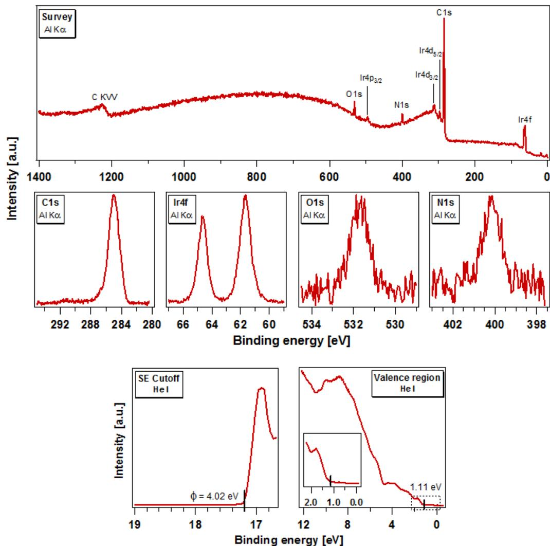
**Figure 5.2:** Survey spectrum, core levels (C1s, Ir4f, O1s, N1s) detailed spectra, SE cutoff and valence band spectra of the Ir(BPA) layer. The O1s and N1s emission spectra do not have good signal-to-noise ratio due to low atomic sensitivities.
