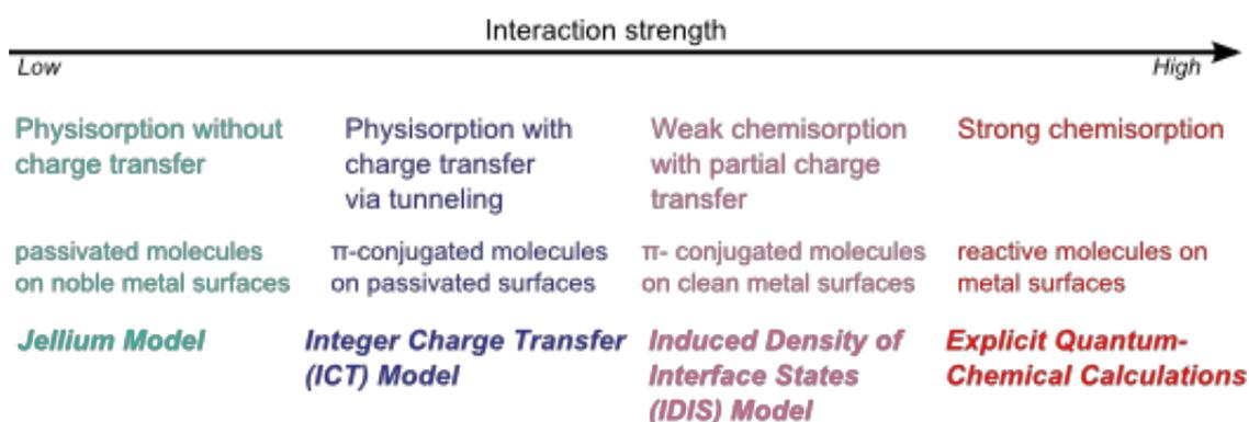
**Figure 2.18:** The different interaction regimes ranging from weak physisorption to strong chemisorption. (First row: interaction type, second row: example system, and third row: standard model). Adapted from [115].
