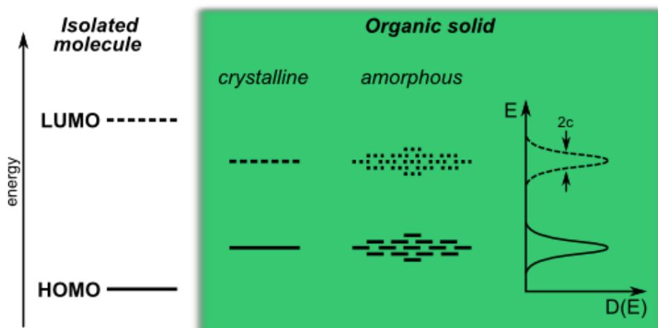
**Figure 2.9:** Energy level scheme for an amorphous organic solid showing a Gaussian density of states which is typically in the range of  $c = 80 - 120$  meV. The bandwidth in molecular crystals is less than 100 meV.[104]
