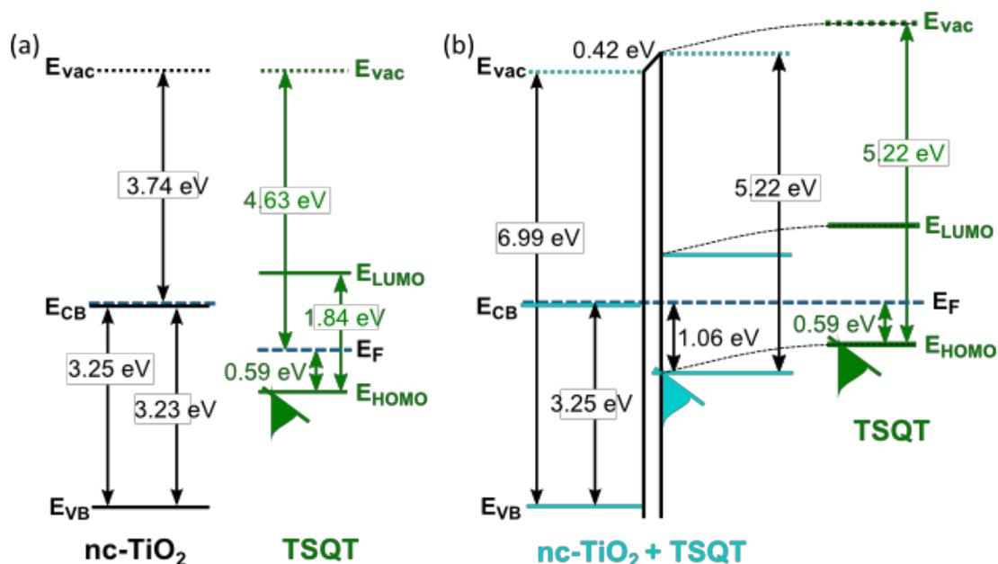
**Figure 9.11:** (a) Anderson lineup of the nc-TiO<sub>2</sub> and TSQT before contact. (b) Energy level alignment at the interfaces of the drop-casted TSQT guest molecules on the nc-TiO<sub>2</sub> matrix, together with the energy levels of the pristine TSQT. An extrapolated complete energy diagram for the nc-TiO<sub>2</sub>/TSQT interface would include a Fermi level pinning in the nc-TiO<sub>2</sub>, a band bending in the TSQT, and a large electron potential barrier at the interface.
