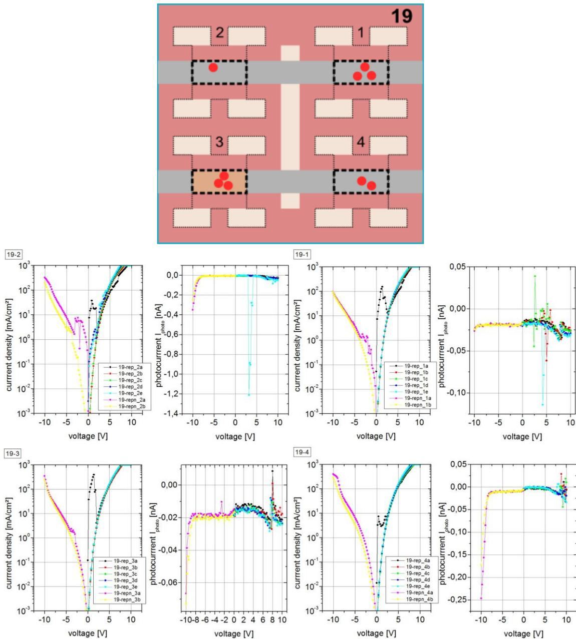
**Figure D.1:** Top-view schematic of Device 19 with its 4 devices (namely: 19-1, 19-2, 19-3 and 19-4). The current density versus applied voltage characteristics of the devices and the photocurrent generated on a silicon photodiode against the applied voltage on the devices are shown.
