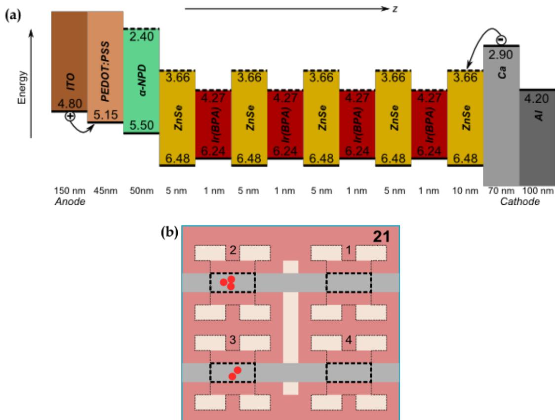
**Figure 7.9:** (a) Schematic diagram of Device 21 structure together with a suggested energy-band diagram. The active layer is composed of alternating 5 ZnSe and 4 Ir(BPA) layers. (b) Top-view schematic picture showing the 4 devices for this substrate. Two of the devices emitted several weak red sparks that lasted as long as the applied current did not finally burn up the devices.
