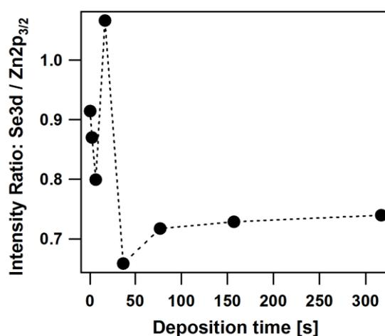
**Figure 5.13:** Photoelectron intensity ratios of the Se3d and Zn2p<sub>3/2</sub> emissions plotted as a function of the deposition time.
