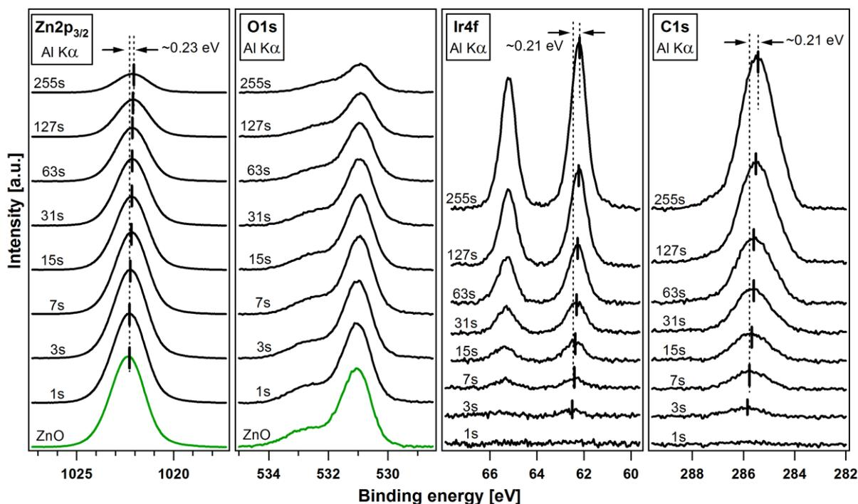
**Figure 8.11:** The Zn2p<sub>3/2</sub>, O1s, Ir4f and C1s core level emission spectra of the as-deposited ZnO film substrate and the Ir(BPA) dye deposited stepwise onto ZnO by thermal evaporation. All spectra were recorded with Al Kα excitation. The Ir(BPA) deposition times are indicated. The ZnO Zn2p<sub>3/2</sub> emission shifts by ~0.23 eV to lower binding energies, while the Ir(BPA) Ir4f and C1s emissions shift by ~0.21 eV to lower binding energies from the 7 s to 255 s deposition steps.
