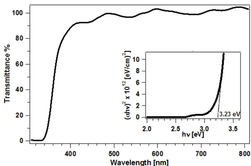
**Figure 9.4:** Optical transmission of the 2 μm thick anatase nc-TiO<sub>2</sub> film deposited on FTO glass substrate. Inset: An optical bandgap of 3.23 eV is derived from the plot,  $(\alpha h\nu)^2$  versus  $h\nu$ .
