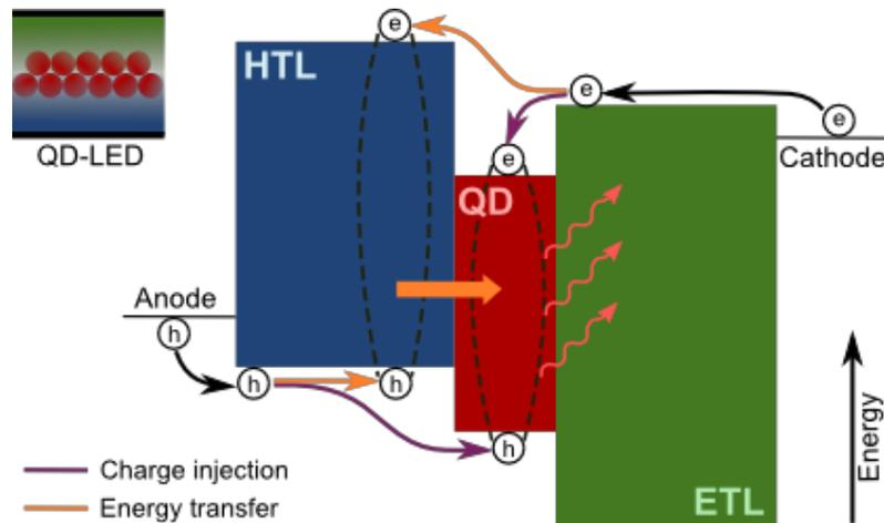
**Figure 1.3:** An energy band diagram of a typical QD-LED with organic electron and hole transport layers. Charge injection and energy transfer are outlined in the diagram as two possible mechanisms for QD excitation.
