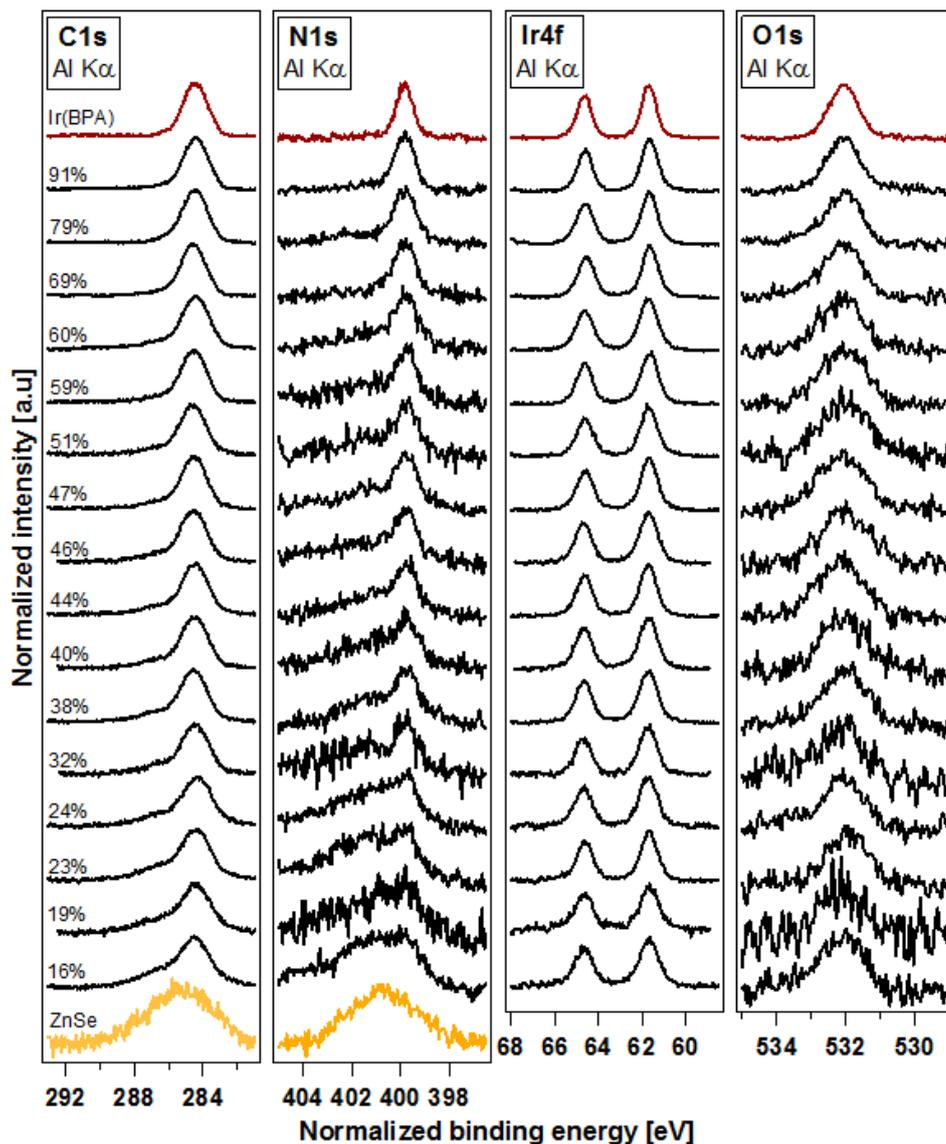
**Figure C.2:** Core line (C1s, N1s, Ir4f, O1s) emissions of the Ir(BPA) dye in several composites. The C1s and N1s emissions of the dye superimpose with broad Auger emissions coming from the ZnSe. The dye volume percentages are indicated.
