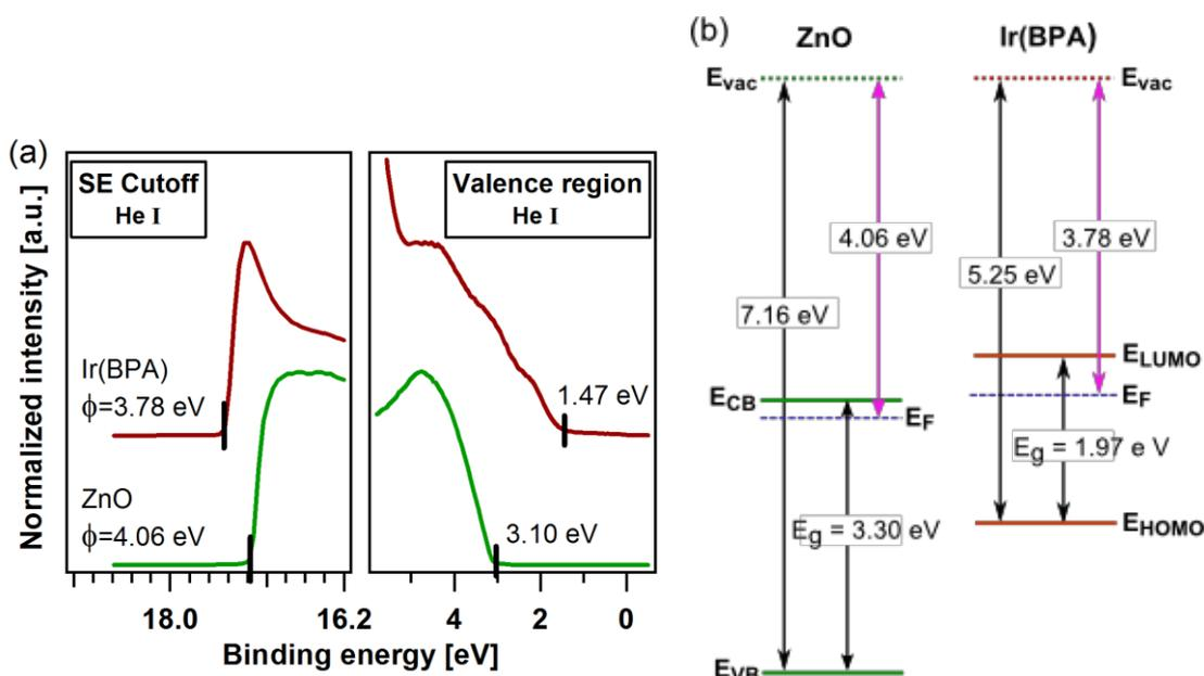
**Figure 8.15:** (a) Secondary electron cutoff and valence region spectra of the annealed ZnO film and fully-closed Ir(BPA) overlayer (a). The work functions ( $\phi$ ) and VBM/HOMO onset values are indicated. (b) An Anderson lineup of the energy levels of these two pristine materials before contact.
