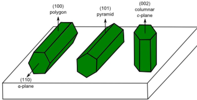
**Figure 8.4:** The hexagonal wurtzite microstructures of ZnO on a substrate together with their corresponding crystal growth orientations.
