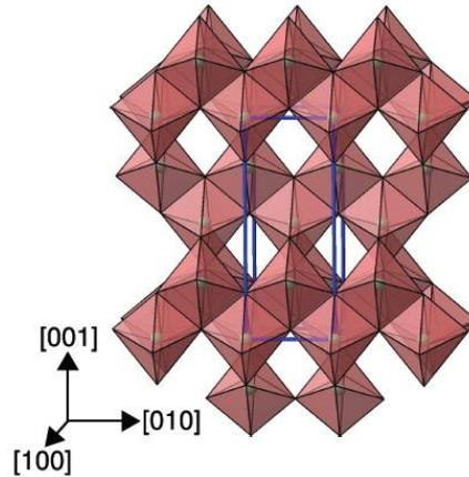
**Figure 9.1:**  $[\text{TiO}_6]^{2-}$  octahedra building block representation for the anatase phase of  $\text{TiO}_2$ .
