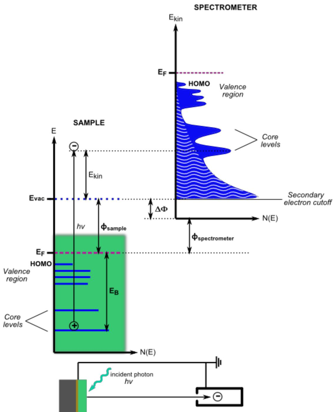
**Figure 3.2:** Schematic diagram of the energy levels in a sample and the corresponding kinetic energy  $E_{kin}$  distribution curve of photoelectrons as detected by the spectrometer. The number of photoelectrons increases strongly with decreasing  $E_{kin}$  and then drops drastically at  $E_{kin}=0$ . The  $E_{kin}$  distribution of the primary (represented by the solid blue curve) and secondary (represented by the curve with wave patterns) photoelectrons are superimposed.
