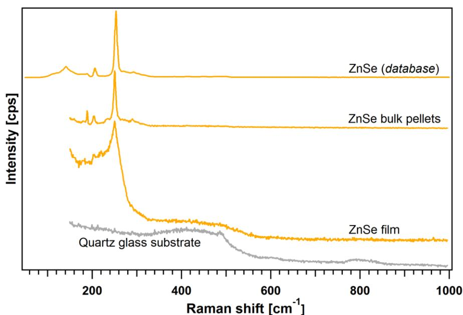
**Figure 6.2:** Raman spectra of ZnSe from a film deposited on a quartz glass substrate, the bulk source pellets and the database. The spectrum obtained for a bare quartz glass substrate is also included.
