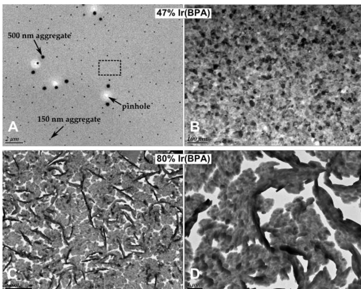
**Figure 6.5:** TEM images of ZnSe + Ir(BPA) two composite films with dye volume percentages of 47% (A, B) and 80% (C, D) under different magnifications. Apparently, the aggregation of the dye increases with increased amount of dye concentration in the composite film.
