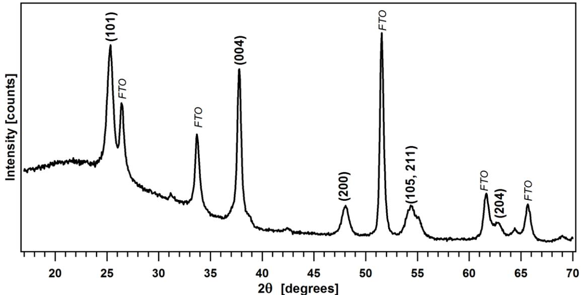
**Figure 9.2:** XRD spectrum of the  $\text{nc-TiO}_2$  film on FTO glass substrate showing reflections of the anatase form.
