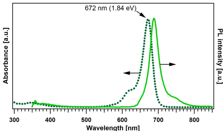
**Figure 9.7:** Room-temperature UV-Vis absorption and emission spectrum of TSQT molecules dispersed in tetrahydrofuran (THF). The emission spectrum is a mirror image of the absorption spectrum. The absorption of the molecule peaks at 672 nm (1.84 eV), while the PL peaks at 688 nm (1.80 eV).
