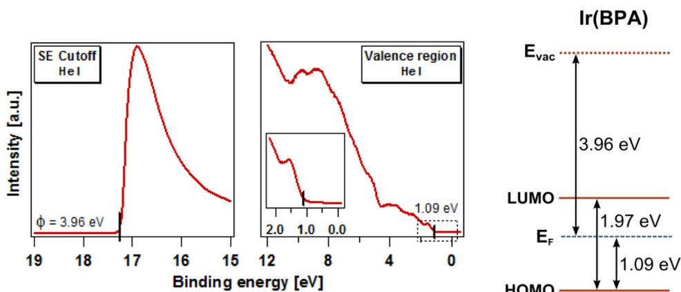
**Figure 4.18:** The SE cutoff where  $\phi$  is determined to be 3.96 eV and the valence region where the HOMO is at 1.09 eV from the Fermi level. The inset shows in greater detail the HOMO onset of the dye. Energy levels of Ir(BPA) as deduced from the UPS measurement. The energy gap of 1.97 eV is taken from the optical measurement.
