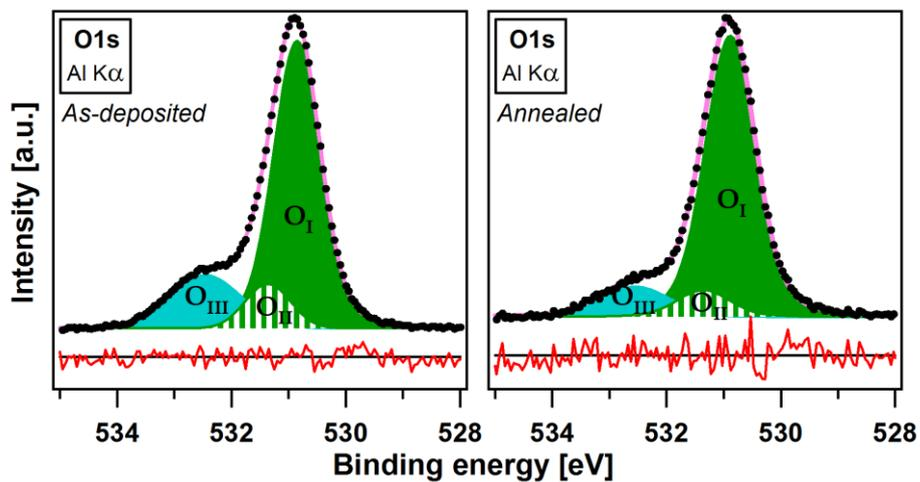
**Figure 8.9:** Spectral fits of the O1s emissions of the as-deposited and annealed ZnO films showing three oxygen species. The photoemission contributions of the higher binding energy O<sub>II</sub> and O<sub>III</sub> species are reduced upon annealing.
