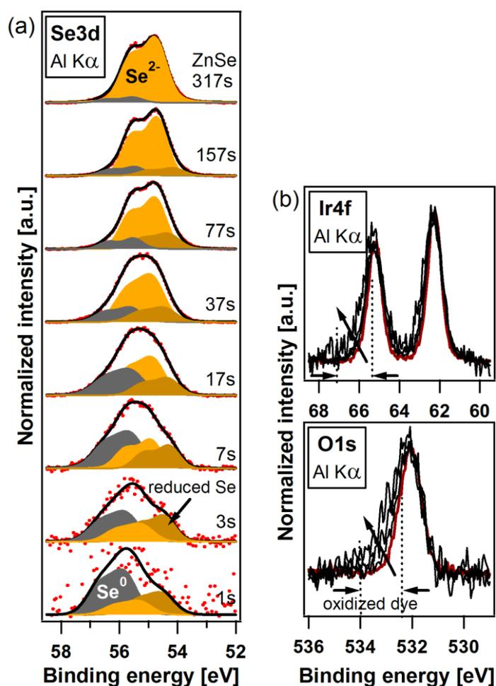
**Figure 5.14:** Peak fitted Se3d photoemission spectra (a). Good fitting is obtained with three contributions assigned to elemental Se<sup>0</sup>, Se<sup>2-</sup> in ZnSe and a more reduced component. (b) Normalized Ir4f and O1s emissions for 0 s, 17 s, 37 s and 77 s ZnSe evaporation show formation of high binding energy components.
