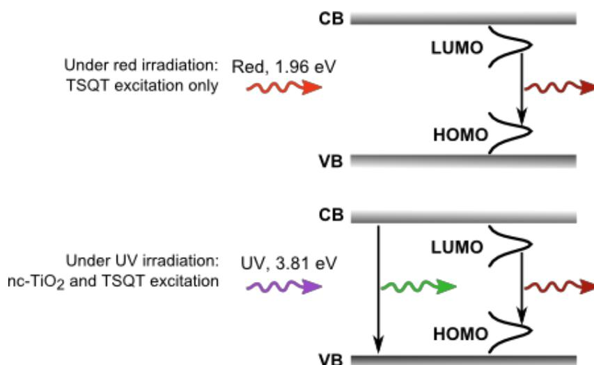
**Figure 9.13:** PL measurement technique employed in this study. Using a red laser for excitation, only the TSQT molecules in the composites are excited; thereby, only the emission of TSQT would then be observed. Under UV laser irradiation, the porous nc-TiO<sub>2</sub> matrix is excited. At this high energy excitation, the absorption of TSQT is very low while that of the nc-TiO<sub>2</sub> is high.
