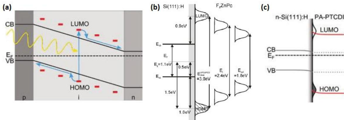
**Figure 1.4:** Electronic structure of the bulk composite absorber in a *p-i-n* device structure (a). Energy band diagrams of the Si(111):H/ $F_8ZnPc$  interface (b) and *n*-Si(111):H/PA-PTCDI interface (c) as determined from PES measurements. The figures are taken from [74, 75]
