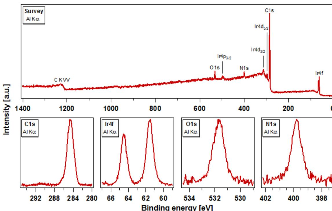
**Figure 4.17:** Survey spectrum showing all the peak photoemissions that are representative of the elemental composition of an Ir(BPA) film deposited on ITO glass substrate. Detailed spectra of the C1s, Ir4f, O1s and N1s emissions confirm the stability of the dye during the deposition through the absence of chemically shifted dye emissions.
