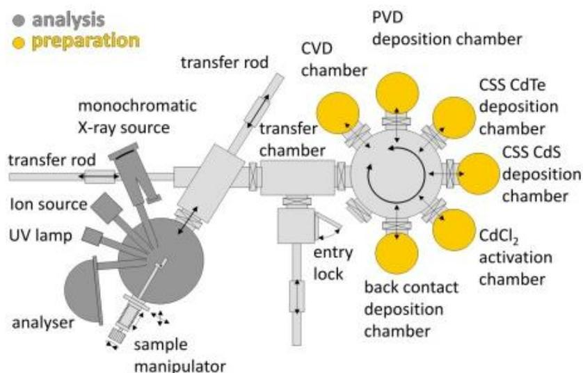
**Figure 3.5:** Layout of the DAISY-SOL in Darmstadt. Different dedicated deposition chambers are all attached to a single distribution chamber that is connected to the analysis chamber for *in-situ* XPS and UPS measurements. Taken from the Surface Science website.<sup>42</sup>
