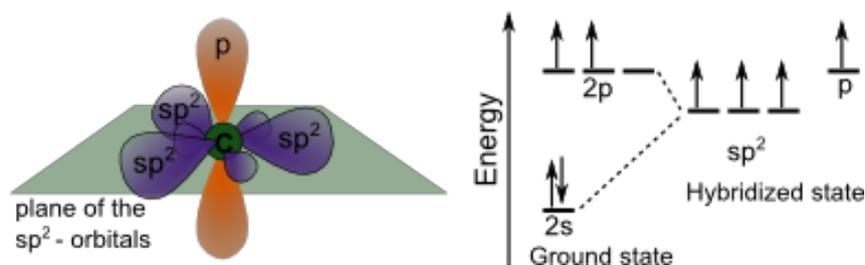
**Figure 2.5:**  $sp^2$  hybridization of carbon. The combination of one  $s$  and two  $p$  orbitals from the same valence shell gives a set of three  $sp^2$  hybridized orbitals that have equivalent energy levels but are  $120^\circ$  spatially apart on a single plane. The remaining  $p$  orbital lies perpendicular to this plane.
