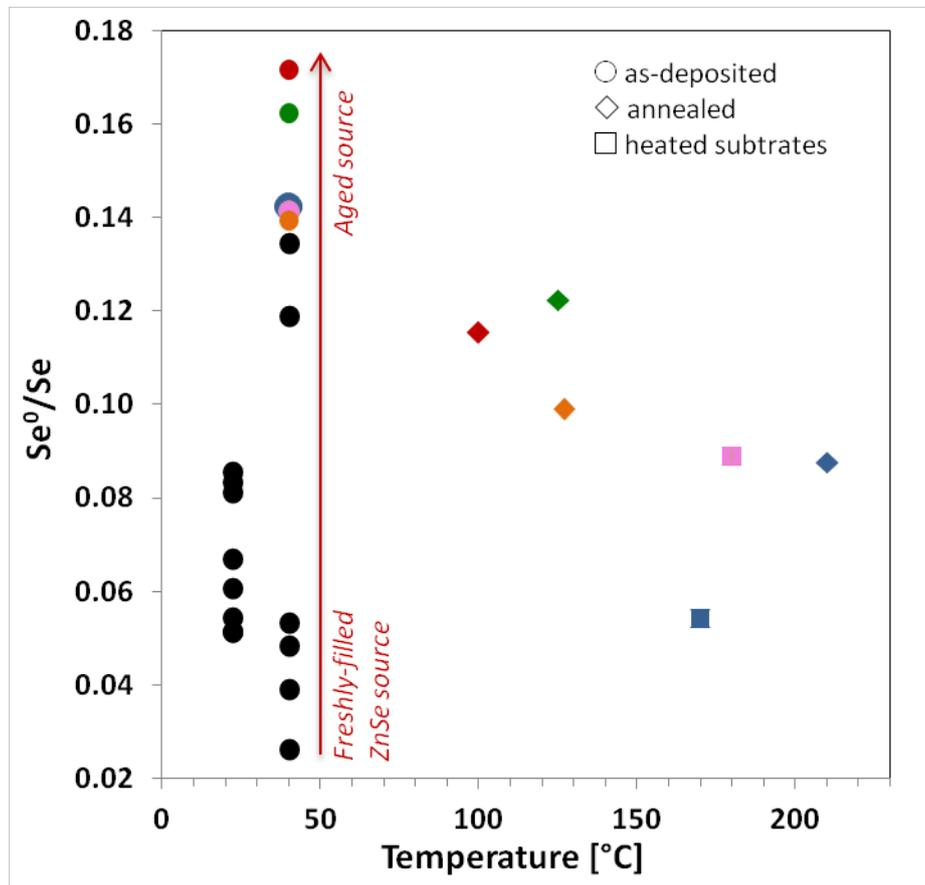
**Figure 4.5:**  $\text{Se}^0$ -to-Se ratio as a function of deposition temperature. The colors of the data points indicate the same batch of samples in the case of the heated substrate treatment and the same samples in the case of the post-deposition annealed treatment. Meanwhile, the shapes indicate the heat treatment performed on the samples. All heat treatments resulted to a reduced  $\text{Se}^0$ . The deposition on a heated substrate exhibited the largest reduction of  $\text{Se}^0$ .
