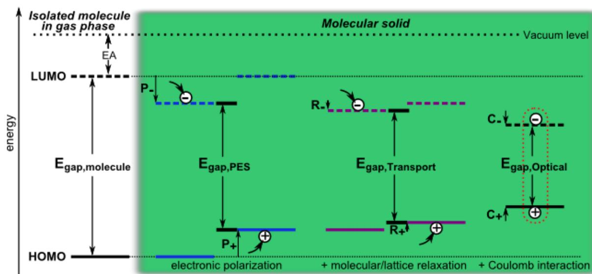
**Figure 2.8:** Energy levels of an isolated molecule and a molecular solid. EA denote electron affinity in the gas phase. Different energy gaps for the solid are probed by different measurement techniques. Figure adapted from [103-106].
