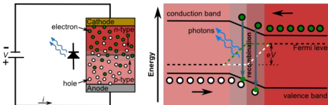
**Figure 2.2:** LED basic working principle. A LED operated with a forward bias leads to current flow, thereby injecting minority carriers into the region of the majority carriers. Photons are emitted during the recombination of electrons and holes.
