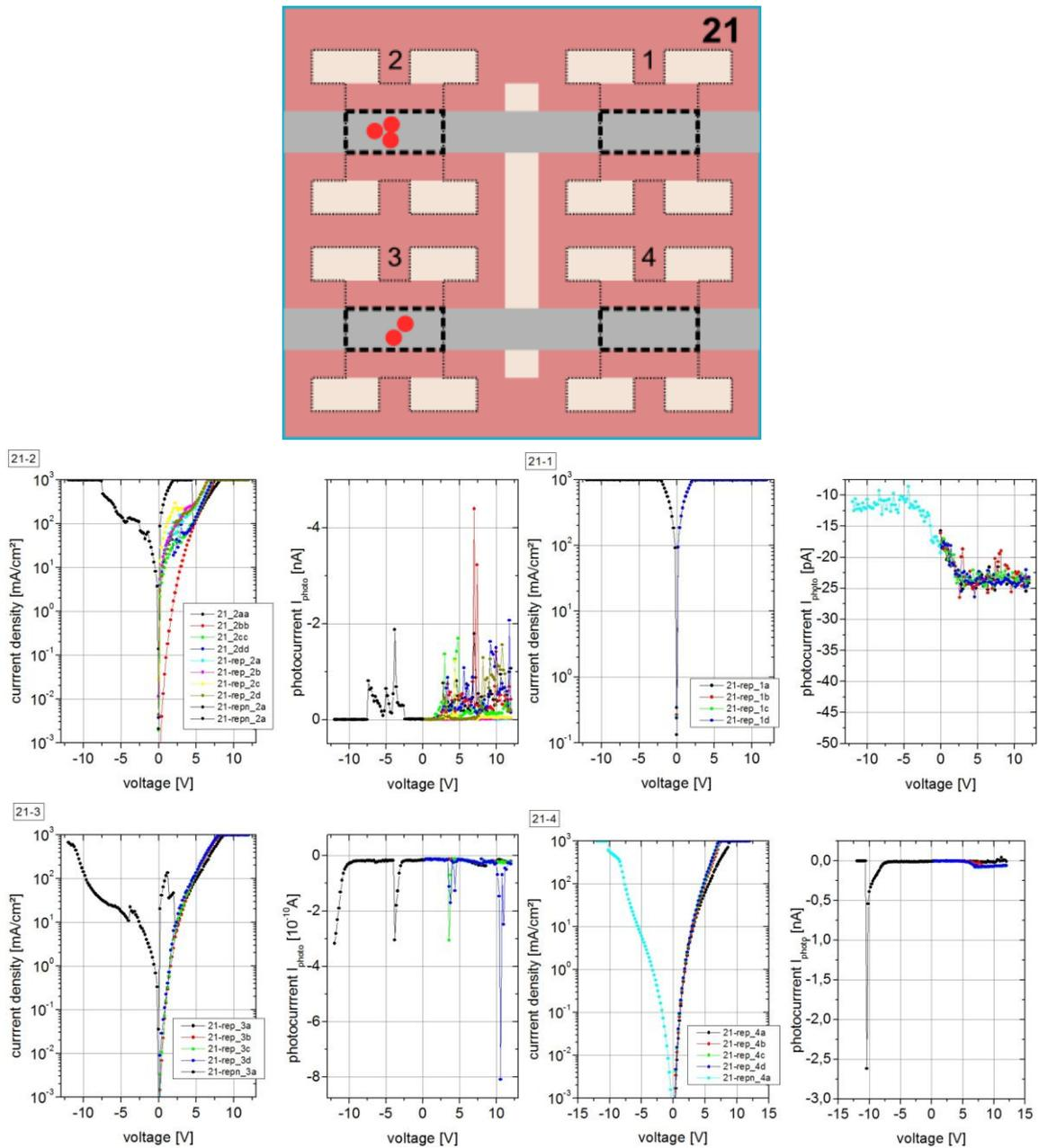
**Figure D.2:** Top-view schematic of Device 21 with its 4 devices (namely: 21-1, 21-2, 21-3 and 21-4). The current density versus applied voltage characteristics of the devices and the photocurrent generated on a silicon photodiode against the applied voltage on the devices are shown.
