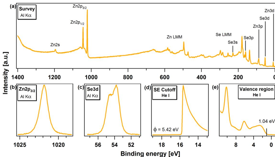
**Figure 4.2:** (a) A survey spectrum showing all the peak photoemissions that are representative of the elemental composition of a ZnSe film deposited on ITO glass substrate. Detailed spectra of (b) Zn2p<sub>3/2</sub> and (c) Se3d emissions. (d) The SE cutoff where  $\phi$  is determined to be 5.42 eV. (e) The valence region where the VBM is at 1.04 eV from the Fermi level.
