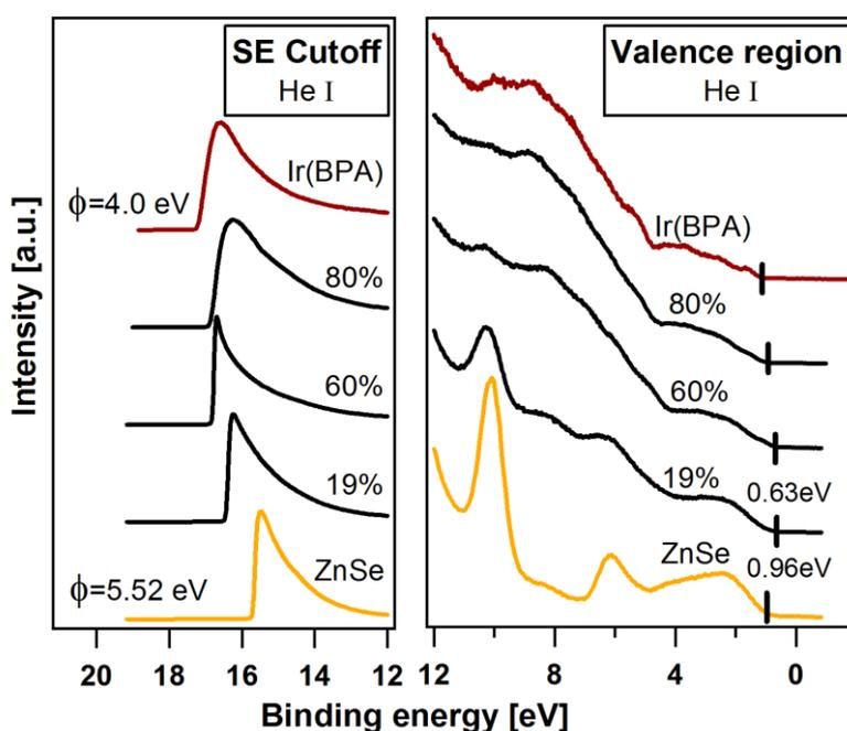
**Figure 5.18:** Secondary electron cutoff and valence band spectra of the composites. The values of  $\phi$  and HOMO/VBM onsets of ZnSe and 19% composite are indicated. The HOMO onset is shifted to a lower binding energy position as compared to that of pristine Ir(BPA).
