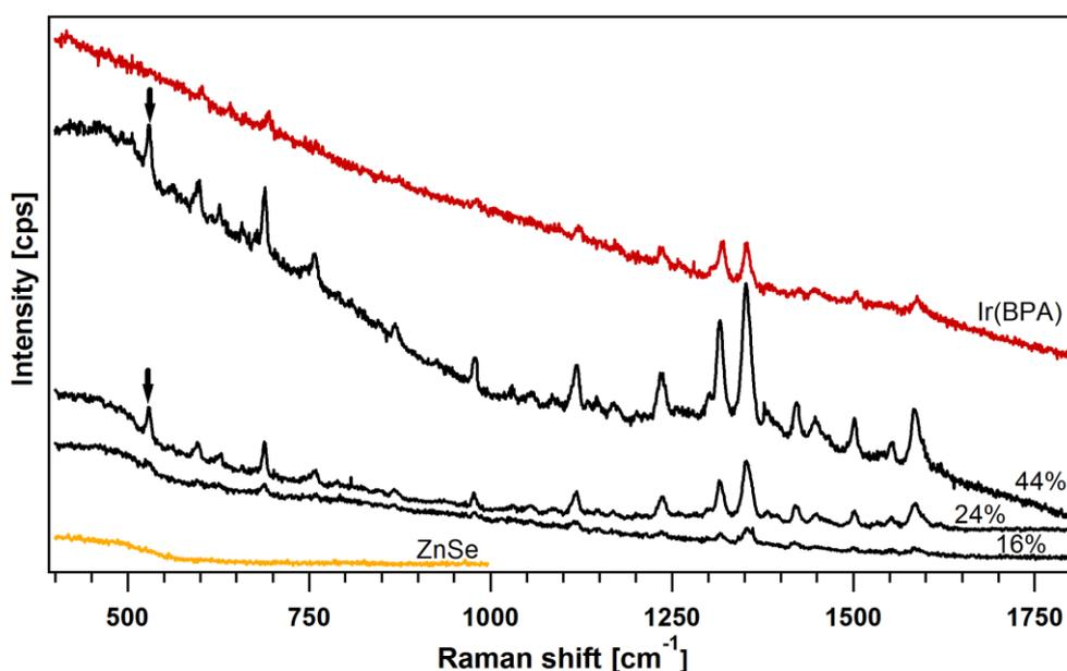
**Figure 6.1:** Raman spectra of ZnSe + Ir(BPA) composite films deposited on quartz glass substrates together with pristine ZnSe film and Ir(BPA) powder. The dye volume percentages are indicated. The vibrational modes of the dye molecules are also present in the composites. Arrows point at an additional vibrational mode at  $529.5 \text{ cm}^{-1}$  that is unique to the composites.
