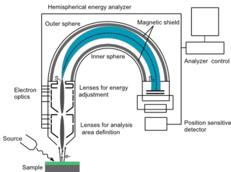
**Figure 3.3:** The working principle of a state-of-the-art photoelectron spectrometer with a hemispherical analyzer (HSA). Photoelectrons are generated through the irradiation of the sample with a monochromated electromagnetic radiation. They are directed to the detector above the sample, passing through the HSA which selects the kinetic energy of the detected electrons. The photoelectrons are eventually detected by a position sensitive detector. Adapted from a website.<sup>40</sup>
