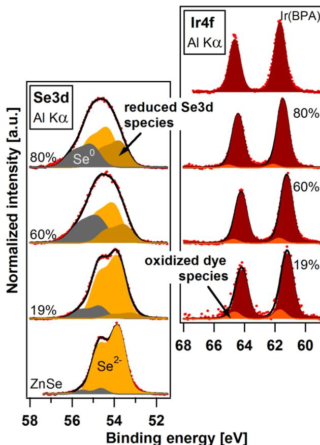
**Figure 5.17:** Curve fitting analysis for Se3d and Ir4f core level emission spectra. Se3d fit reveals the presence of three species contributing to the emission:  $Se^{2-}$ ,  $Se^0$  and reduced Se. Ir4f fit shows presence of oxidized dye species.
