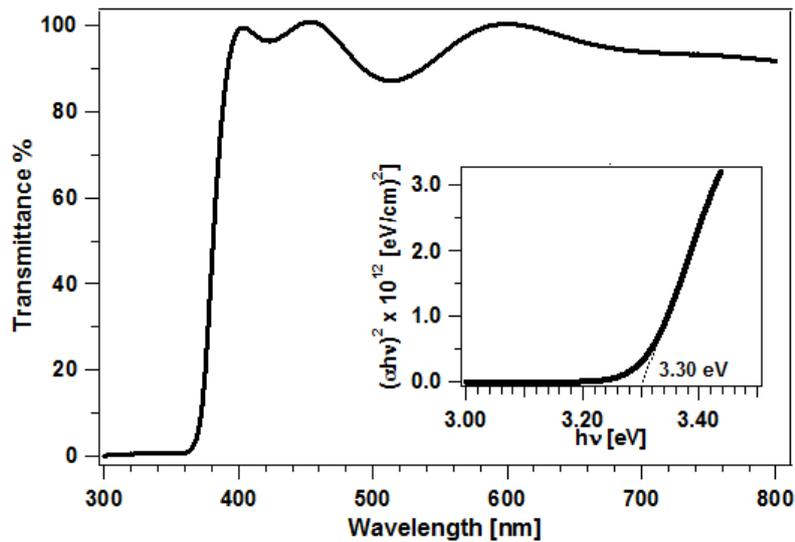
**Figure 8.5:** Transmission spectrum of the ZnO film deposited on an ITO glass substrate that exhibits a sharp optical absorption edge. Inset: An optical bandgap of 3.30 eV is derived from the plot of  $(\alpha h\nu)^2$  versus  $h\nu$  of the ZnO film.
