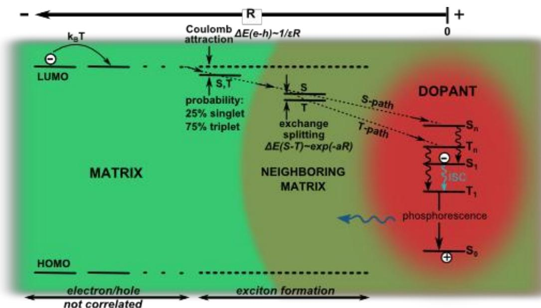
**Figure 2.15:** Dynamics of exciton formation in an organic matrix doped with emitter molecules. (R: electron-hole separation, a: constant depending on the respective matrix and dopant material). Adapted from [113].
