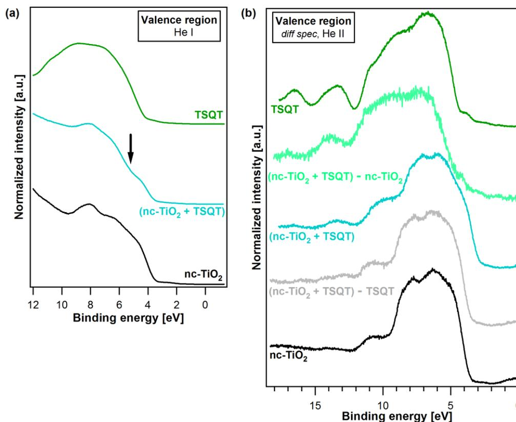
**Figure E.4:** Valence region emission spectra from the pristine nc-TiO<sub>2</sub> and TSQT layers and the nc-TiO<sub>2</sub> + TSQT composite under (a) He I and (b) He II photoexcitations. The gray and light green curves in (b) give the difference spectra of the He II valence region.
