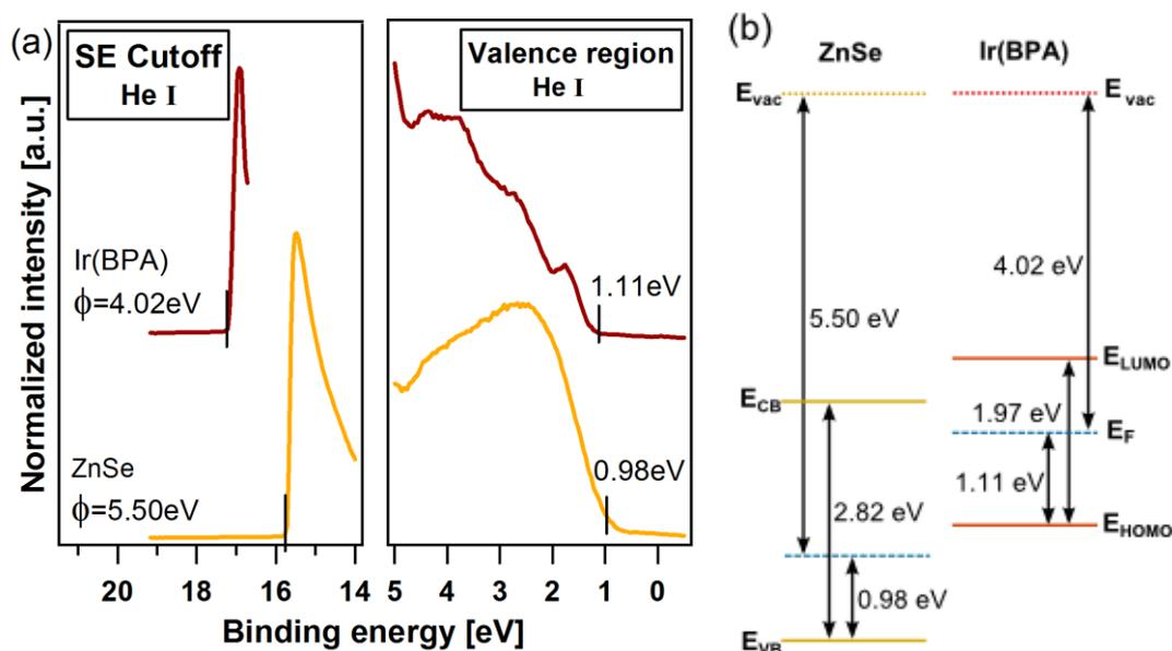
**Figure 5.3:** (a) SE cutoff and valence region spectra of pristine ZnSe and pristine Ir(BPA). The work function ( $\phi$ ) and VBM/HOMO onset values are indicated. (b) A schematic diagram of the relative energy levels of ZnSe and Ir(BPA). Aligning the vacuum levels of the two materials before contact reveals that the energy level alignment is not as needed for carrier injection as described in Figure 1.5.
