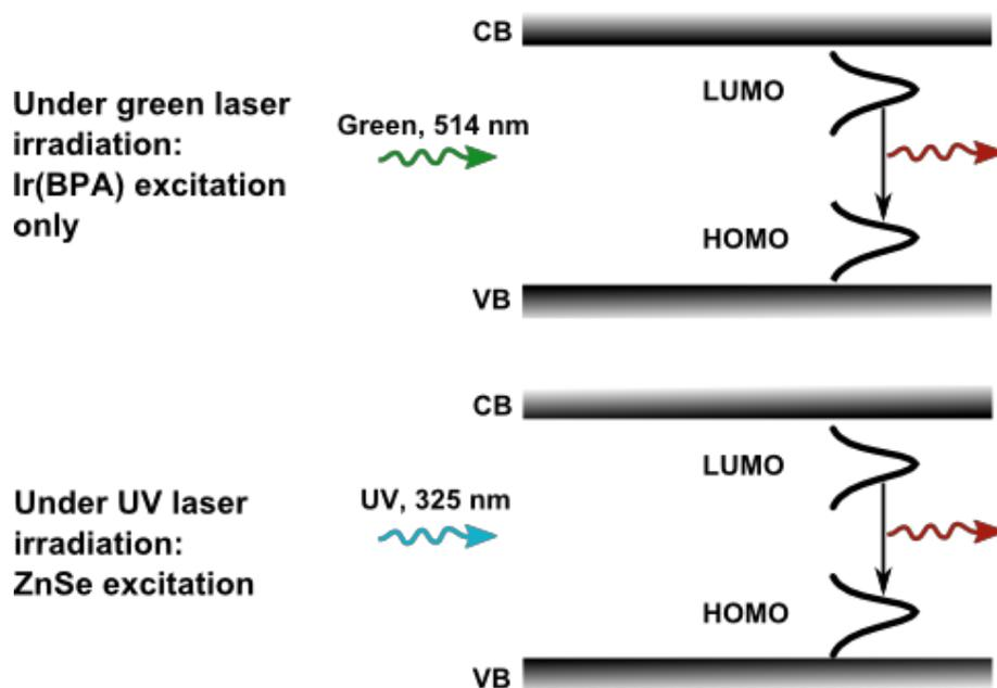
**Figure 6.11:** Photoluminescence measurement technique employed in this study. Using a green laser for excitation, only the Ir(BPA) molecules in the composites are excited; thereby, only the emission of Ir(BPA) would then be observed. Under UV laser irradiation, the ZnSe matrix can be excited. If the dye does not absorb in the UV region, then any emission coming from the dye can be accounted to a Förster energy transfer from ZnSe to the dye.
