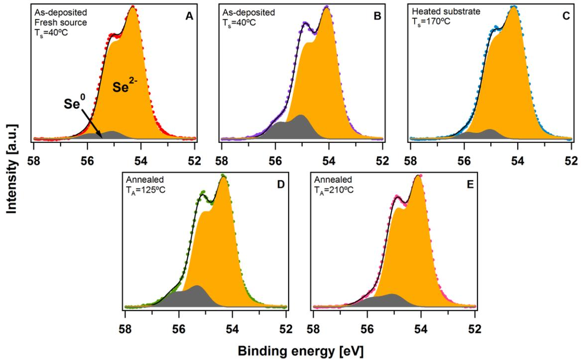
**Figure 4.4:** Spectral fits of the Se3d emission (A: As-grown film deposited from freshly-filled source, B: As-grown film deposited from aged source, C: Film deposited on heated substrate from aged source, C-D: Annealed as-grown films deposited from aged source).
