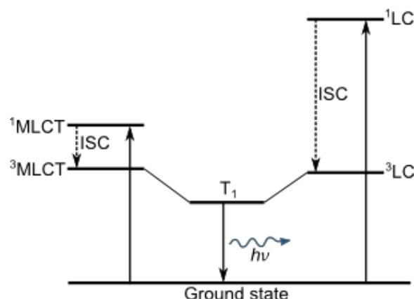
**Figure 4.14:** Narrow energetic distance and overlap between  $^3\text{MLCT}$  and  $^3\text{LC}$  states result in a mixed lowest excited triplet state  $T_1$ . Adapted from [255].
