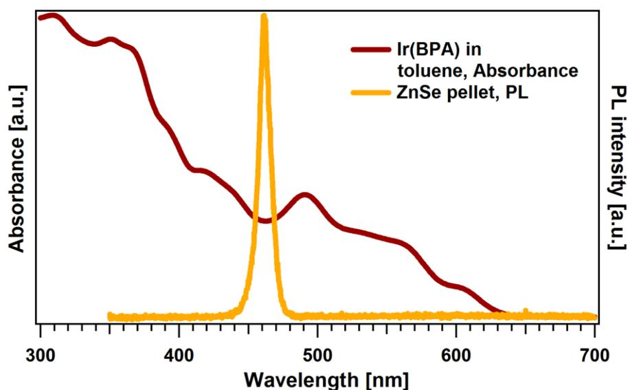
**Figure 6.10:** Photoluminescence spectrum of a ZnSe pellet shown together with the absorption spectrum of Ir(BPA) molecules dispersed in toluene to demonstrate the total spectral overlap, which indicates the likelihood of resonant exciton energy transfer from ZnSe to Ir(BPA) molecules.
