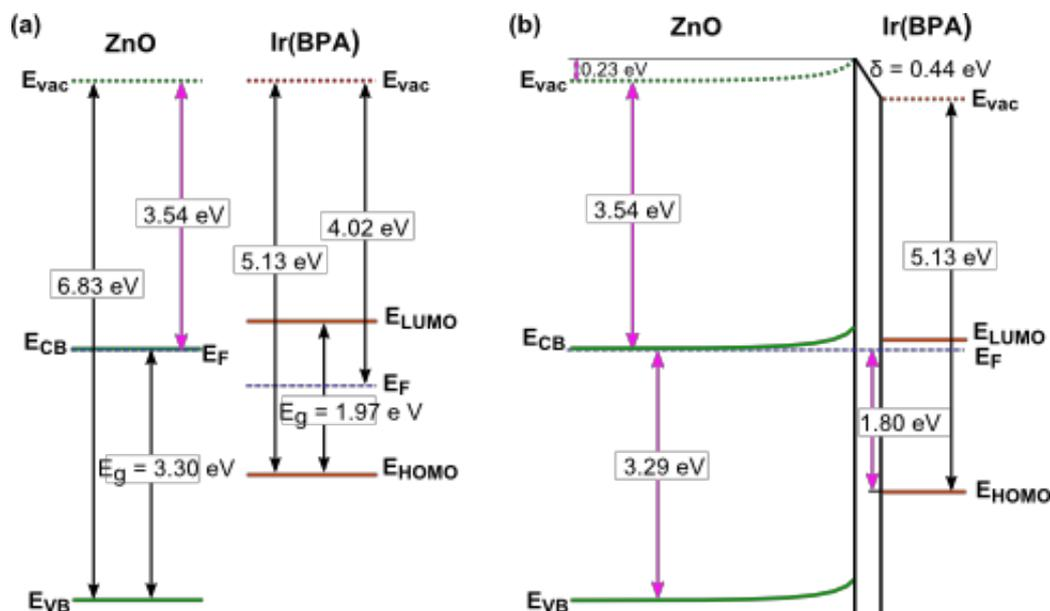
**Figure 8.14:** (a) Anderson lineup of the energy levels of the pristine as-deposited ZnO (left) and pristine Ir(BPA) (right) (adapted from Figure 5.3 b) before contact. (b) Interface band diagram of the as-deposited ZnO/Ir(BPA) bilayer that includes an interface dipole of 0.44 eV and ZnO band bending of 0.23 eV. The energy levels for Ir(BPA) drawn in the diagram is representative only of the formed dye monolayer (i.e. at the 7 s deposition step).
