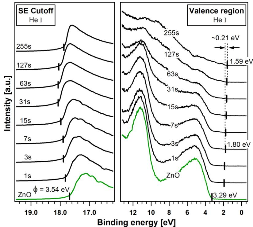
**Figure 8.13:** Secondary electron cutoff and valence region spectra during the step-wise deposition of Ir(BPA) on an as-deposited ZnO film. The Ir(BPA) deposition times are indicated. The HOMO<sub>onset</sub> of Ir(BPA) shifts from 1.80 eV at the 7 s deposition step to 1.59 eV by the last deposition step.
