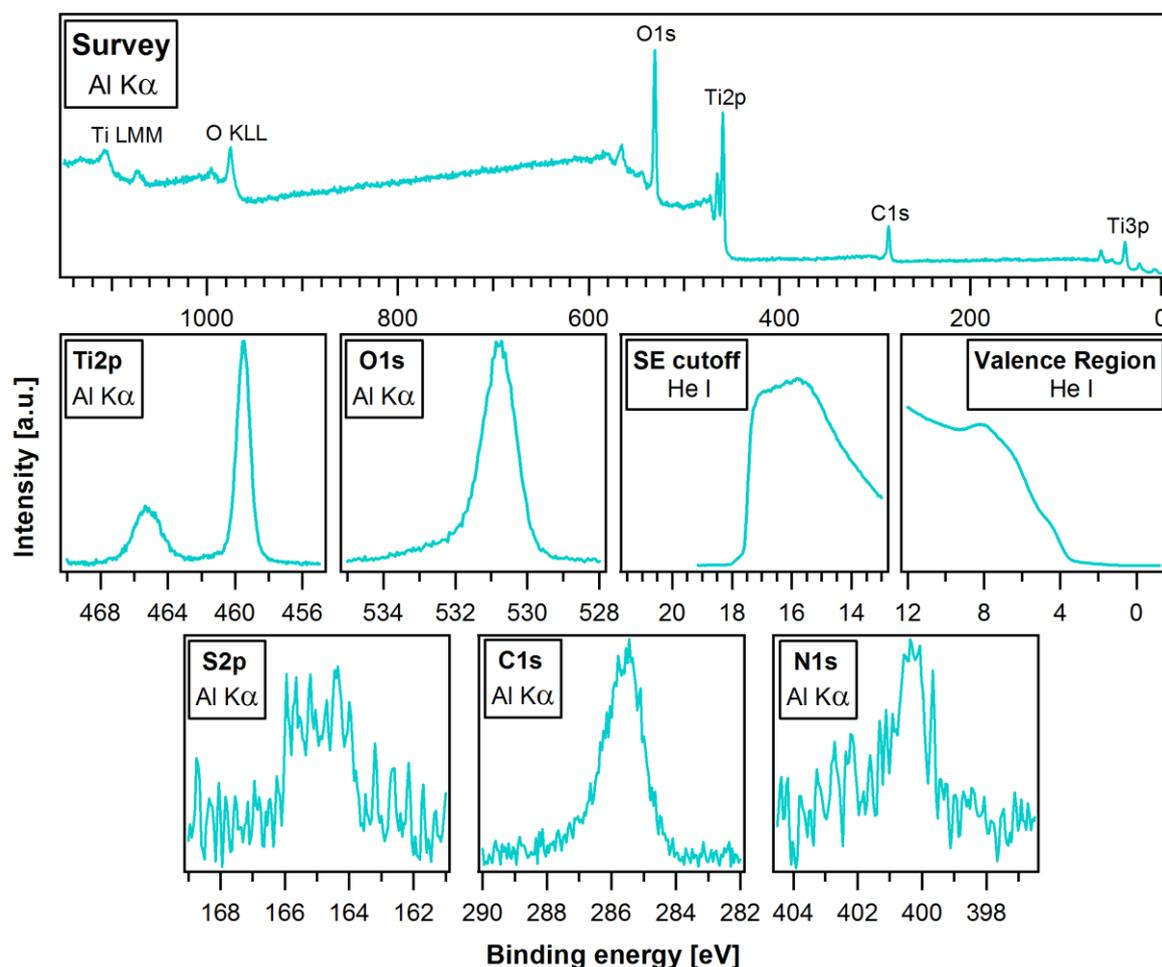
**Figure E.3:** Survey spectrum and detailed spectra of the Ti2p, O1s, S2p, C1s and N1s core line emissions from the nc-TiO<sub>2</sub> + TSQT composite, together with the spectra for the SE cutoff and valence region.
