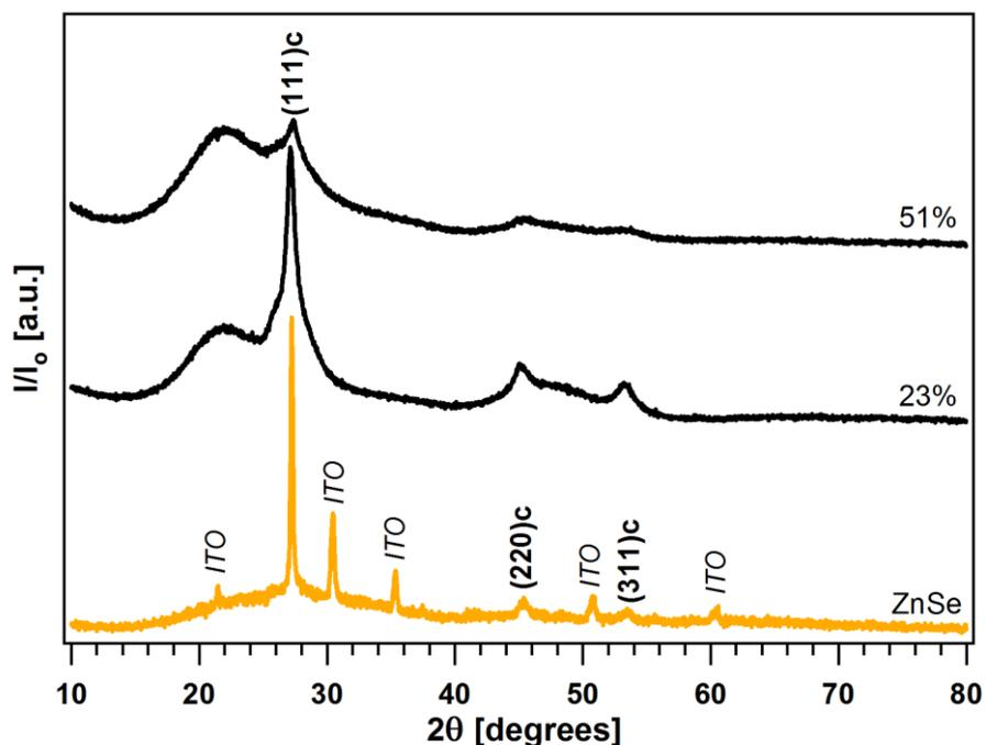
**Figure 6.4:** X-ray diffraction patterns of ZnSe film deposited on ITO on glass substrate at room temperature.
