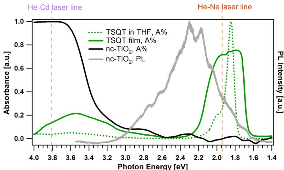
**Figure 9.12:** PL spectrum of the nc-TiO<sub>2</sub> layer (gray curve) shown together with the absorption spectra of TSQT molecules dispersed in THF and spin-coated on a quartz glass substrate (green curves) to demonstrate the spectral overlap, which indicates the likelihood of resonant exciton energy transfer from nc-TiO<sub>2</sub> to TSQT.
