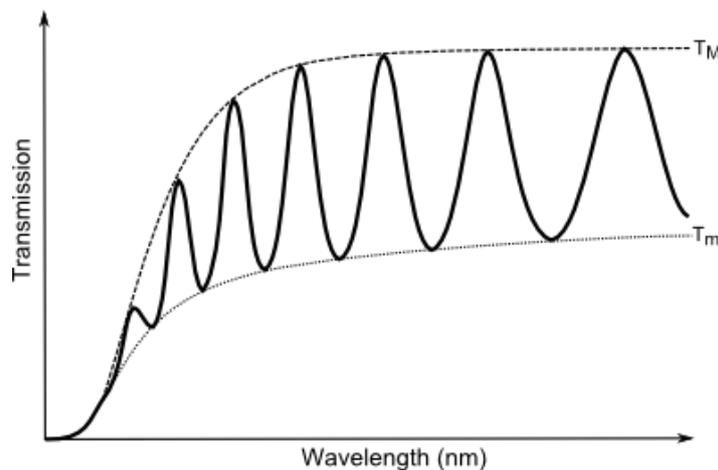
**Figure 3.9:** A sample transmission spectrum to illustrate the interference fringes that can be found from uniform thin films grown on transparent substrates.  $T_M$  and  $T_m$ , which are continuous functions of the wavelength, represent the envelopes for the maxima and minima of the interference fringes.
