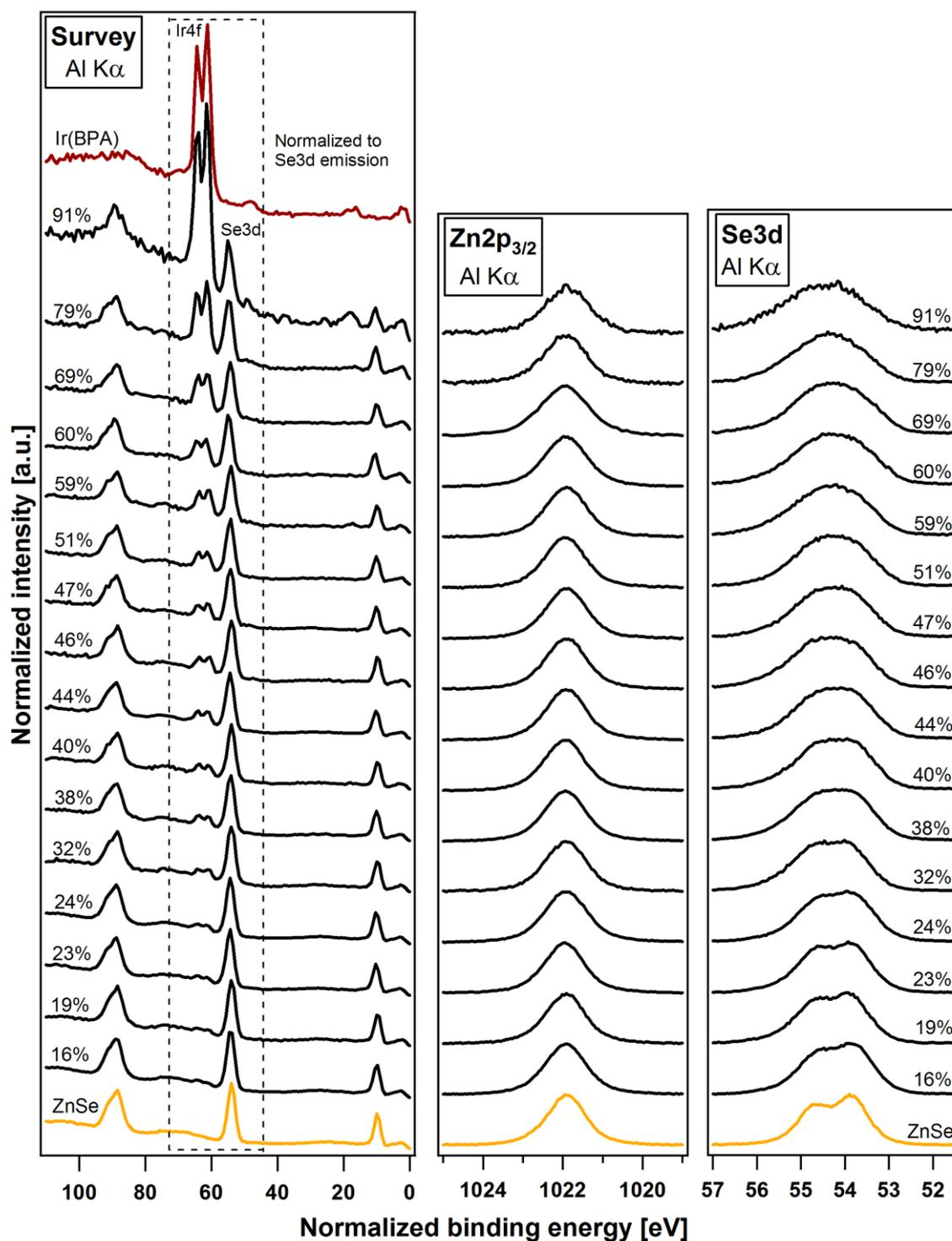
**Figure C.1:** Survey spectra, Zn2p<sub>3/2</sub> and Se3d detailed spectra of several composites. The survey spectra are normalized to the peak of the Se3d emission in order to obtain a rough visualization of the dye to ZnSe+Se ratio. The dye volume percentages are indicated.
