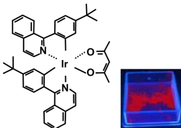
**Figure 4.15:** Molecular structure of Ir(BPA). The central metal atom, iridium, is coordinated by conjugated organic ligands. Photograph: Ir(BPA) powder under UV lamp illumination displaying a bright red luminescence even at RT and ambient atmosphere.
