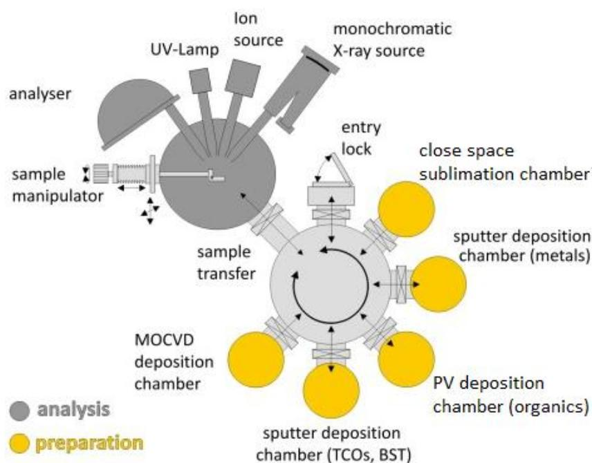
**Figure 3.4:** Layout of the DAISY-MAT in Darmstadt. Different dedicated deposition chambers are all attached to a single distribution chamber that is connected to the analysis chamber for *in-situ* XPS and UPS measurements. Adapted from the Surface Science website.<sup>41</sup>
