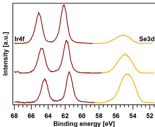
**Figure 6.7:** Ir4f and Se3d emissions of the 80% composite measured at different parts of the sample. Variations in the intensity ratio of the Ir4f and Se3d emissions confirms the inhomogeneity observed in the ZnSe and Ir(BPA) distribution from the TEM images.
