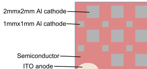
**Figure 7.1:** Top-view schematic picture of a sandwich-type electrode geometry for devices: the bottom-most is a glass substrate covered entirely with unpatterned ITO layer as the anode, the various semiconductor films are on top of the ITO layer, and the top-most is comprised of 8 2mm x 2mm and 6 1mm x 1mm aluminum cathode pads. This, in total, yields 14 devices with identical cross-sectional structures.
