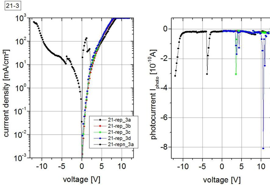
**Figure 7.10:** Current density versus applied (reverse and forward) voltage for Device 21-3. The photocurrent generated on a silicon photodiode against the applied voltage on the device are plotted here as well.
