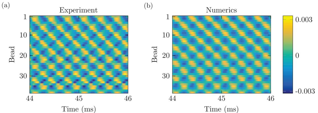
Figure 3.22: Velocity of each particle for a driven frequency at 3 kHz when the steady state is achieved for (a) experimental and (b) numerical results.
