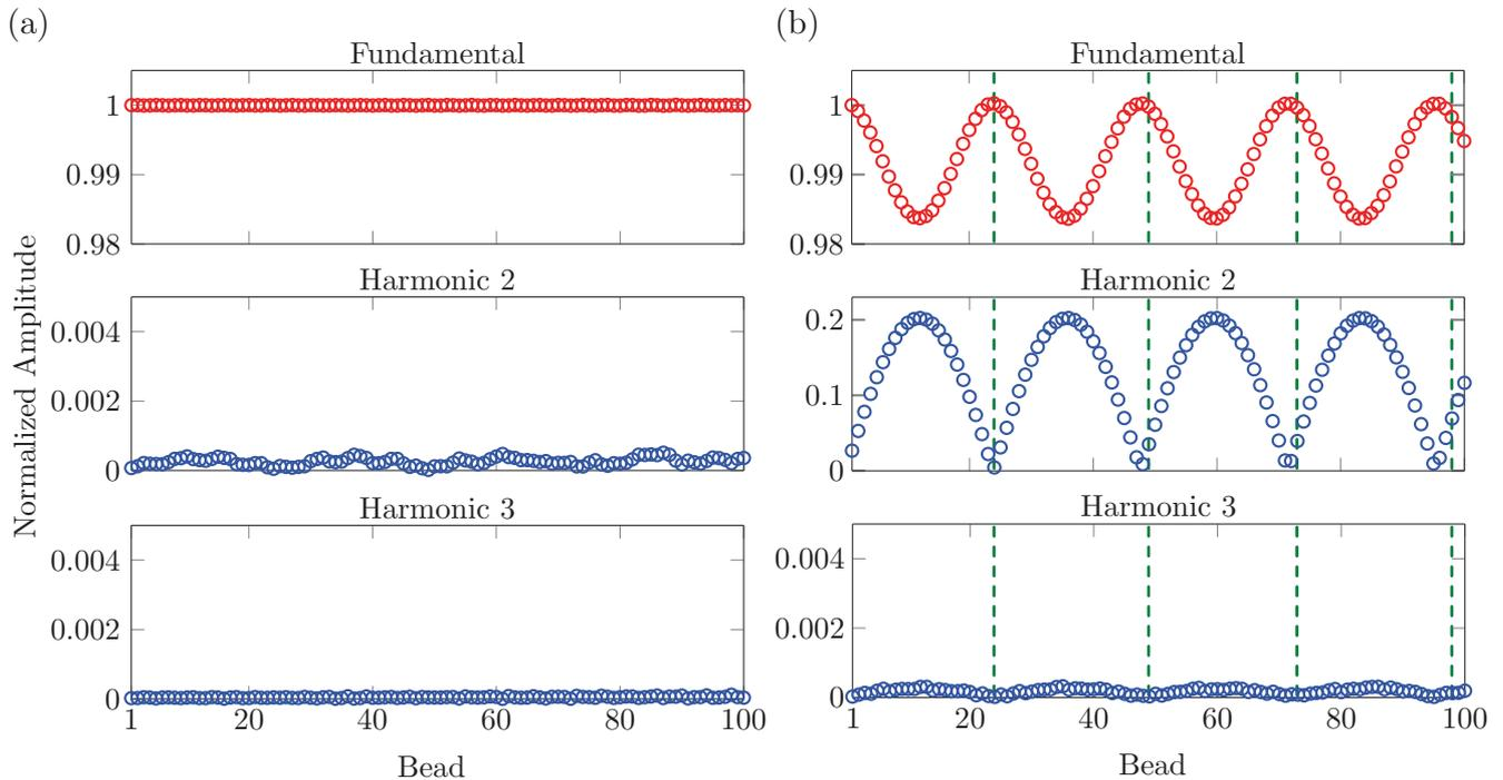
Figure 3.14: Normalized amplitude of the fundamental, second and third harmonics considering lossless propagation for displacement amplitudes (a)  $\delta/\delta_0 = 3 \cdot 10^{-4}$  and (b)  $\delta/\delta_0 = 0.19$ , for both cases  $f_1/f_c = 0.42$ . Green dashed line are analytical predictions of the disappearance of the second harmonic contribution from Eq. (3.8).
