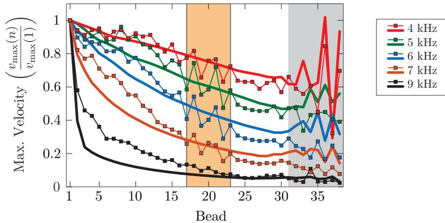
Figure 3.4: Maximum of the wave packet velocity as a function of beads for different carrier frequencies. Thick lines correspond to numerical results with  $\tau = 1.9$  ms and  $F_0 = 2.25$  N, and thin lines with markers are experimental results. The grey/orange zones correspond to the presence of reflected wave.
