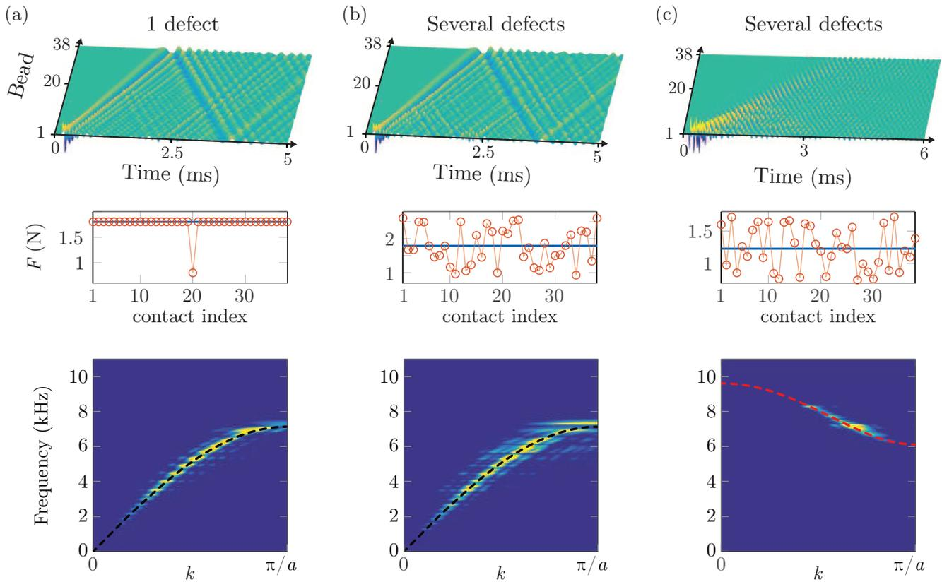
Figure 2.28: Numerical results for (a) the  $L$  branch with  $F_0 = 1.8$  N and  $\tau = 2.4$  ms, defect at bead 20 with  $F_0 = 0.8$  N (b) with several defects  $F = 1.8 \pm 0.9$  N and  $\tau = 2.4$  ms (c)  $TR$  branch with  $F = 1.23 \pm 0.5$  N and  $\tau' = 0.8$  ms. The blue line corresponds to the mean value of  $F_0$ . The dashed lines correspond to the analytical dispersion curve using a constant  $F_0$ .
