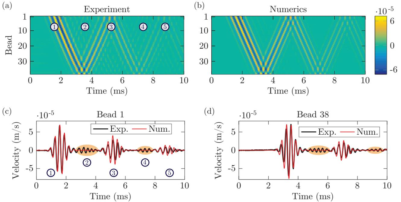
Figure 3.2: (a) Experimental spatio-temporal diagram of the velocity of the particles during the propagation of a wave packet with a central frequency of 3 kHz. (b) Numerical spatio-temporal diagram with  $F_0 = 2.25$  N and  $\tau = 1.9$  ms. Velocity as a function of time for (c) the first bead and (d) the last bead of the chain.
