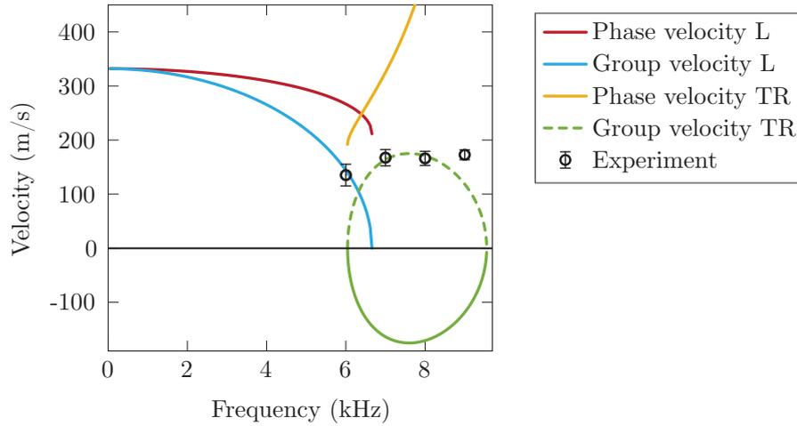
Figure 3.10: Analytical phase and group velocities for the  $L$  and  $TR$  branches. The dashed line correspond to the absolute value of the analytical group velocity in  $TR$  branch, markers correspond to the experimental results.
