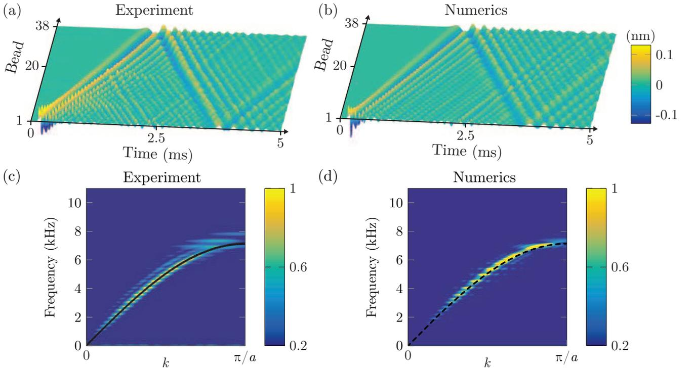
Figure 2.24: (a) Experimental and (b) numerical (from Eq. (2.42)) results for the longitudinal wave propagation as function of time for a chain of 38 beads. (c) Experimental and (d) numerical dispersion curves with  $F_0 = 1.8$  N and  $\tau = 2.4$  ms. Analytical dispersion curves are superimposed.
