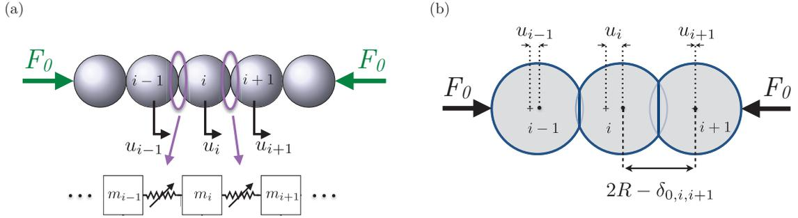
Figure 1.7: (a) Schematics of the one-dimensional granular chain, a mass-nonlinear spring lattice. (b) Schematics of the statically compressed granular chain by a static force  $F_0$ . The crosses represent the initial positions of the particle centers in a statically compressed chain while the black circles denote the current positions [11].
