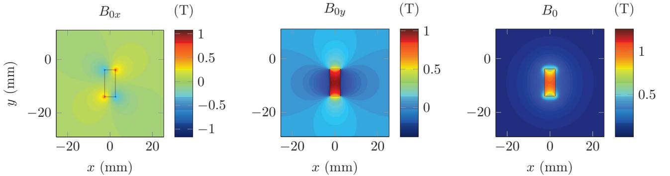
Figure A.3: 2D finite element simulation of the magnetic field of one permanent magnet for the  $x$  and  $y$  components, left and center panels respectively, and the density of magnetic field (right panel).
