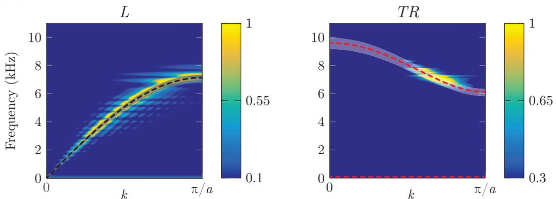
Figure 2.27: Numerical dispersion curves for the longitudinal branch (left) and (right) for the transverse-rotational branches after 100 simulations varying the precompressional force  $F_0 \pm 0.3$  N. The analytical dispersion curves are superimposed considering  $F_0$  (dashed lines)  $\pm 0.3$  N (shadow zones).
