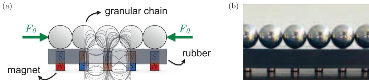
Figure 2.10: (a) Schematic diagram of the granular chain on top of permanent magnets within a rubber. Forces and magnetic flux lines induced by the magnetic field have been superimposed. (b) Photography of the experimental setup for the "free" chain configuration.
