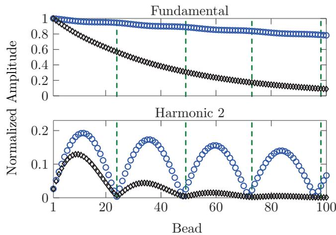
Figure 3.15: Normalized amplitude of the fundamental and second harmonic considering lossy propagation for displacement amplitudes  $\delta/\delta_0 = 0.19$  and  $f_1/f_c = 0.42$ . Blue circles correspond to a dissipative term  $\tau = 10$  ms and black diamonds to  $\tau = 1$  ms. Green dashed line are analytical prediction of the disappearance of the second harmonic contribution from Eq. (3.8).
