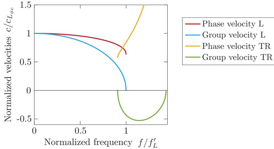
Figure 3.7: Analytical phase and group velocities for the  $L$  and  $TR$  branches normalized by the maximum of the longitudinal phase velocity  $c_{L\phi c}$ . The frequency is normalized by the longitudinal cutoff frequency  $f'_L$ .
