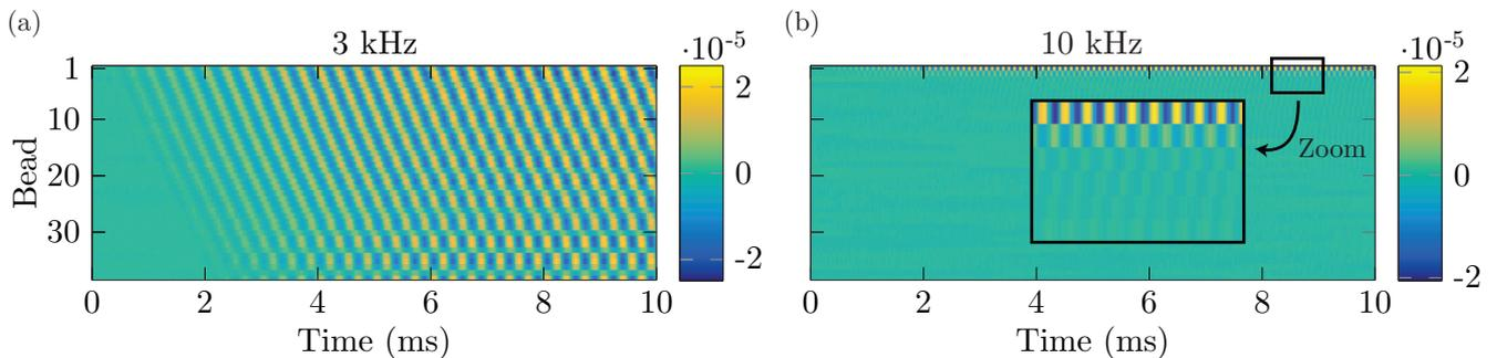
Figure 3.5: Experimental velocity of each particle as function of time for harmonic wave frequency (a) inside and (b) outside the propagating band.
