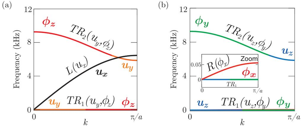
Figure 2.4: Dispersion curves for the infinite free granular chain considering the static force  $F_0 = 1$  N and  $\tilde{K}_N = \tilde{K}_S = \tilde{K}_T = 0$  for (a) modes polarized in the sagittal plane and (b) modes polarized in the horizontal plane.
