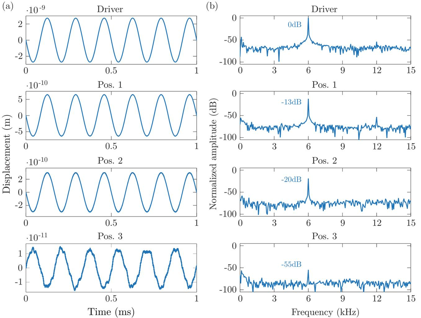
Figure 3.26: Experimental results for a driven frequency at  $\Omega_{T2} < \Omega = 0.91 < 1$  and linear amplitude of excitation in (a) temporal and (b) frequency domains.
