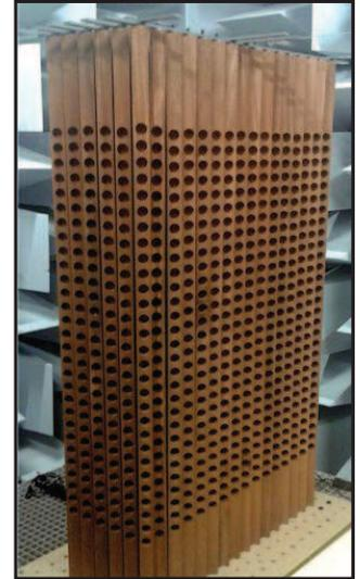
Figure 1.1: Example of a 3D phononic crystal made of square-rod rigid scatterers incorporating a periodic arrangement of quarter wavelength resonators [26].
