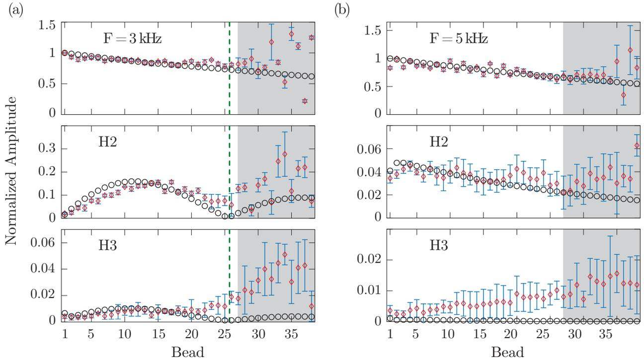
Figure 3.18: Experimental and numerical harmonic generation for a driving frequency at (a) 3 kHz:  $f_1/f_c = 0.41$  and (b) 5 kHz:  $f_1/f_c = 0.69$ . Black circles correspond to numerics and red diamonds to experiment, respectively. Green dashed line is given from Eq. (3.8). Grey zones correspond to the experimental presence of reflection during the analysis.
