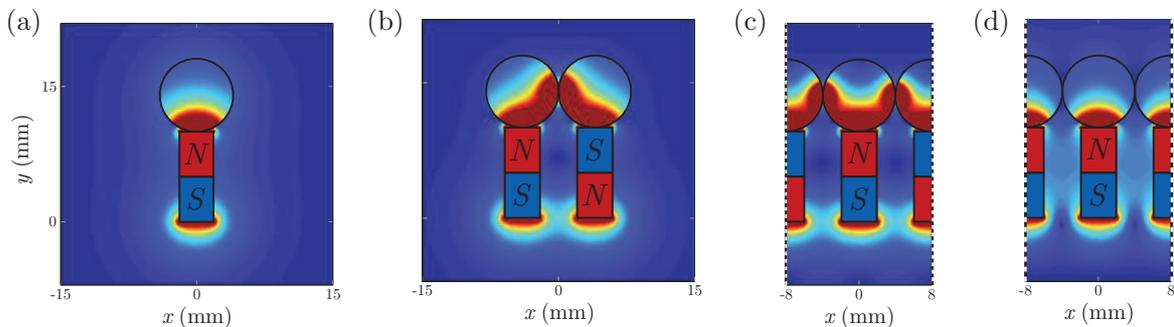
Figure 1.17: Simulated magnetic field created by (a) one magnet, (b) two magnets with poles alternatively oriented. (c) Simulated magnetic field using periodic conditions for alternatively and (d) identically orientations of the poles. The colormap is saturated to see clearly the magnetization into the beads. Red to blue color means high to low density of magnetic field respectively.
