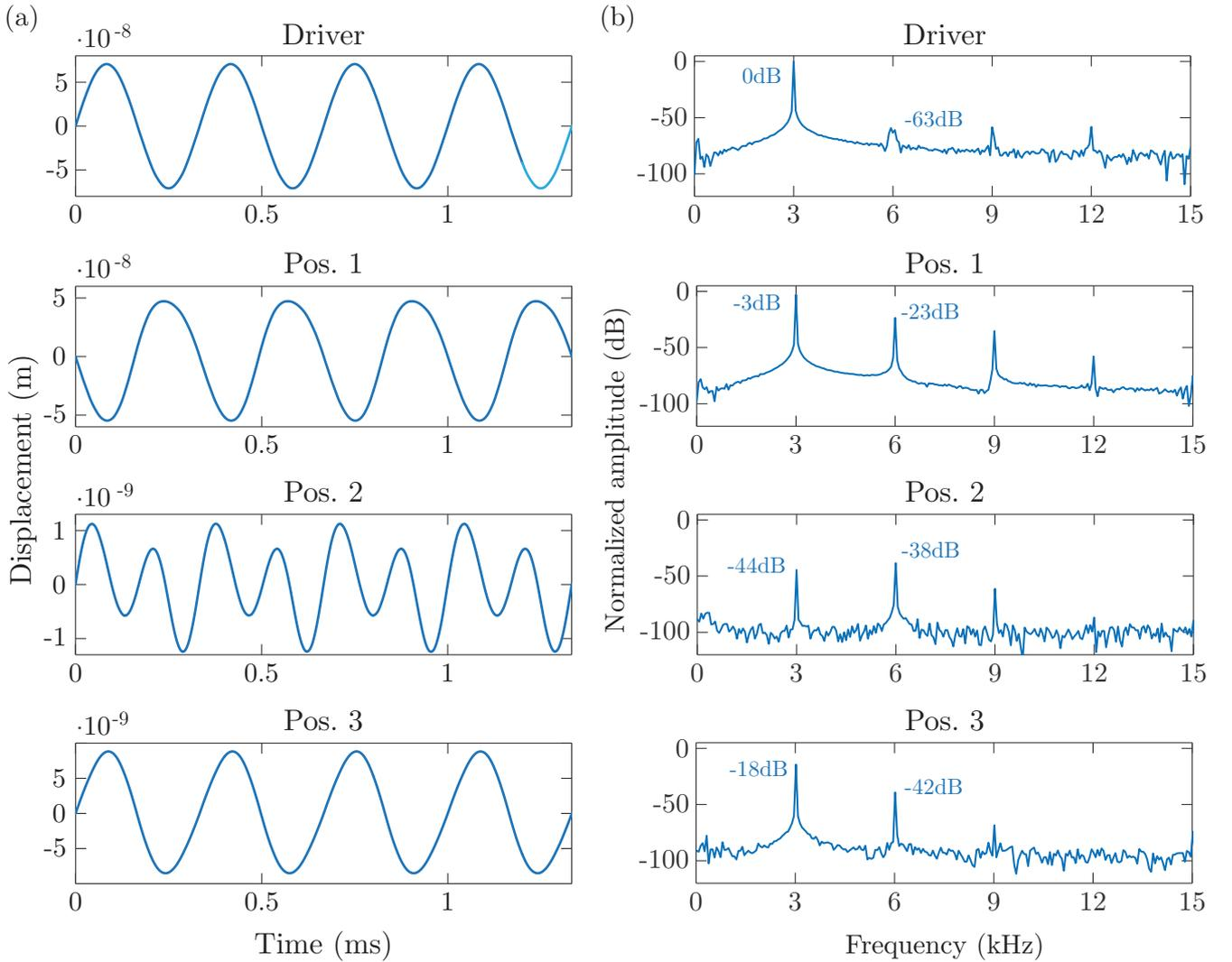
Figure 3.27: Experimental results for a driven frequency at  $\Omega = 0.455 < \Omega_{T2}$  and nonlinear amplitude of excitation ( $\delta/\delta_0 = 0.32$ ) in (a) temporal and (b) frequency domains.
