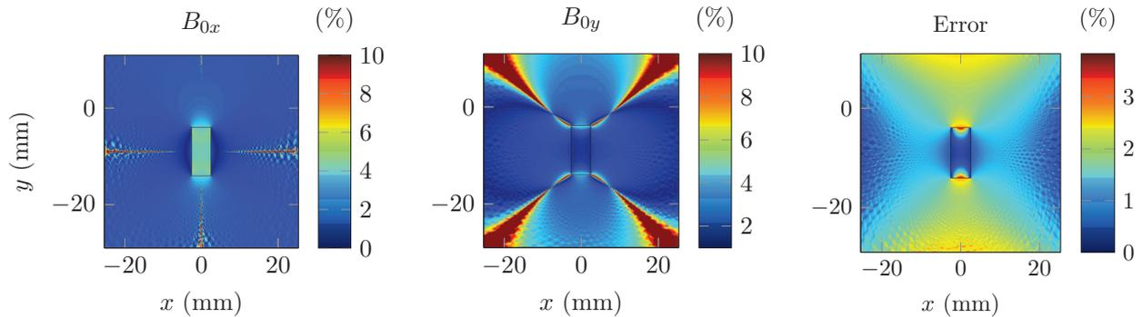
Figure A.4: Error between the analytical model and the finite element simulation magnetic field for one magnet.
