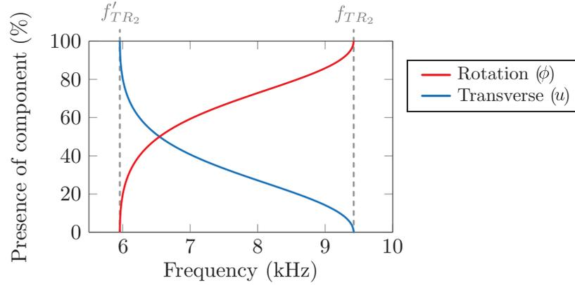
Figure 2.6: Relative amplitude (in percentage) of transverse ( $u$ ) and rotation ( $\phi$ ) in the  $TR_2$  branch as a function of the frequency. Dashed line corresponds to the lower and higher cutoff frequencies for the  $TR_2$  branch.
