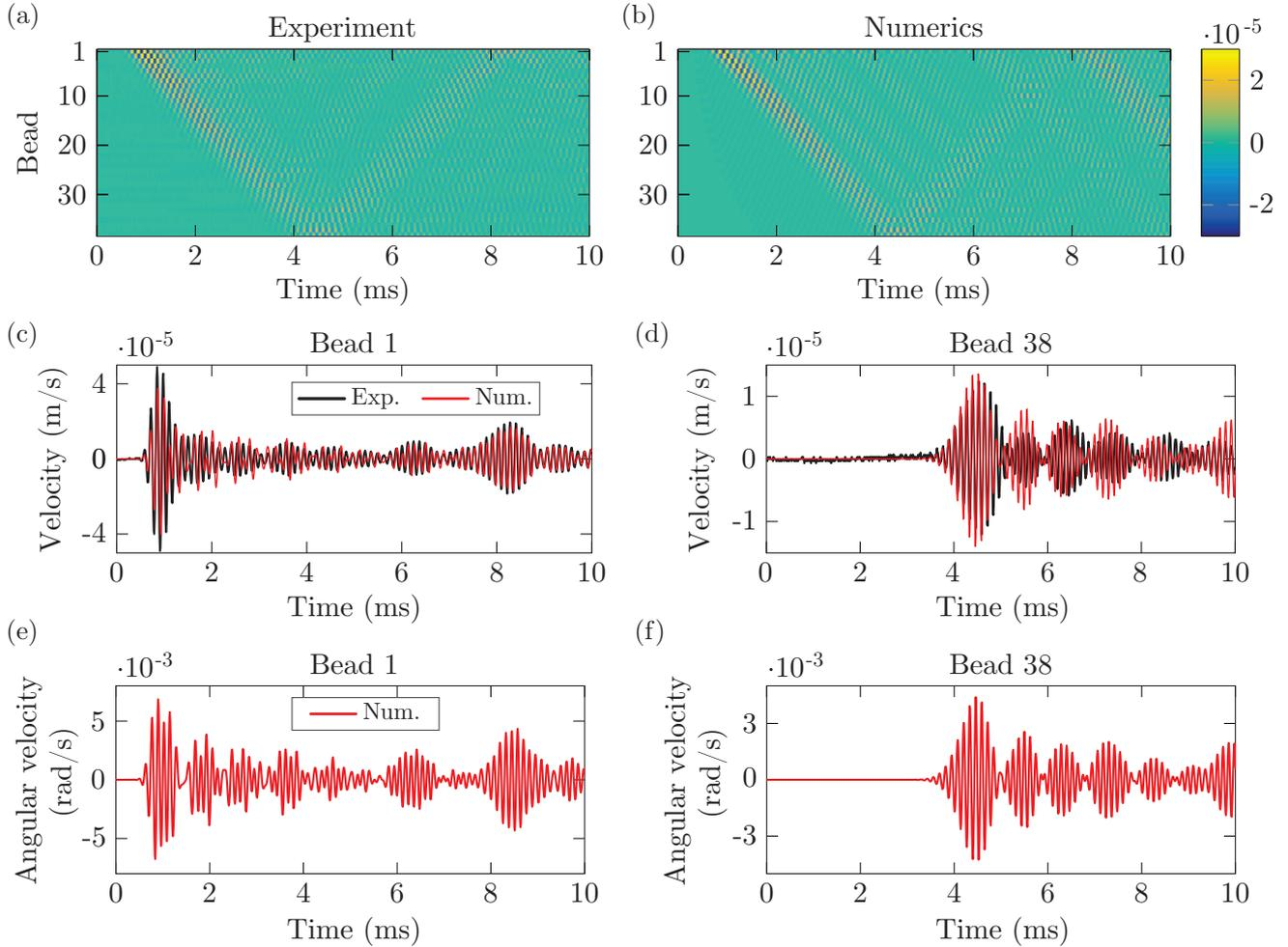
Figure 3.9: (a) Experimental velocity measured for each particle driving with a wave packet with a central frequency of 7 kHz, (b) transverse part from numerics with  $F_0 = 1.2$  N and  $\tau = 1$  ms. Transverse velocity as a function of time for (c) the first bead and (d) the last bead of the chain. Angular velocity from numerical simulation for (e) the first and (f) the last bead of the chain.
