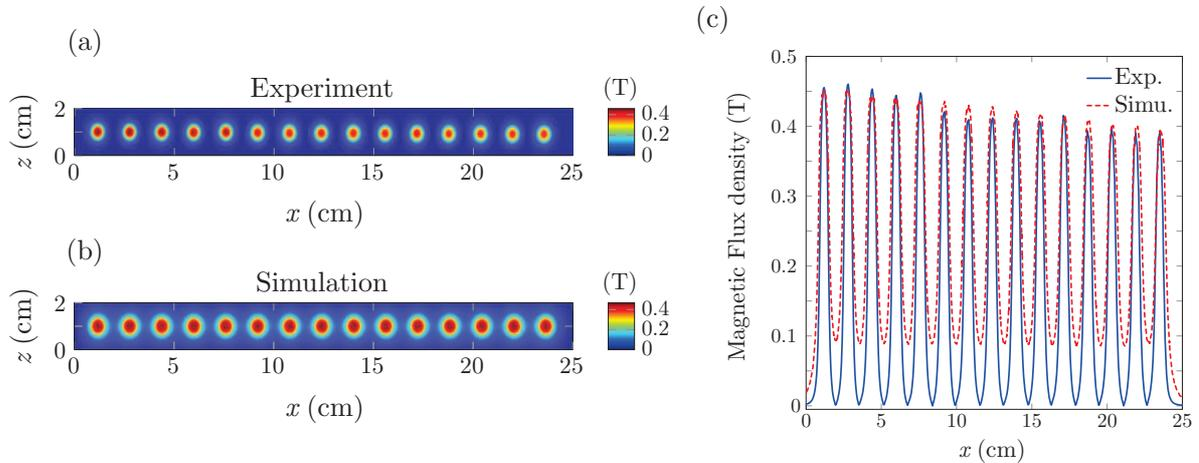
Figure 1.16: Magnetic field created by a chain of 15 magnets from (a) experiments and (b) simulations. (c) Magnetic field on the line  $z = 1$  cm from experiments (solid line) and simulations (dashed line).
