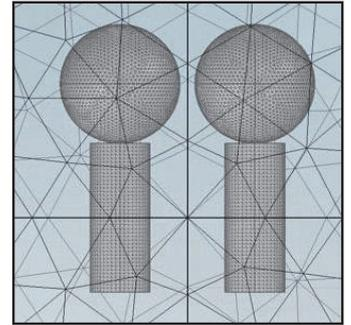
Figure 1.18: Simulated mesh in FEM, non contact case.
