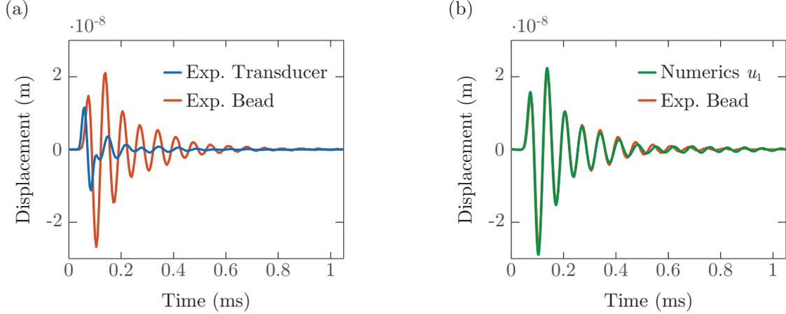
Figure 2.18: (a) Experimental signal measured on the transducer (blue) and on the bead (red) for a pulse excitation. (b) Numerical displacement (green) solving Eq.(2.39) with  $K_g = 1.49 \cdot 10^8$  N/m,  $\tau_g = 0.17$  ms and experimental signal measured on the bead (red).
