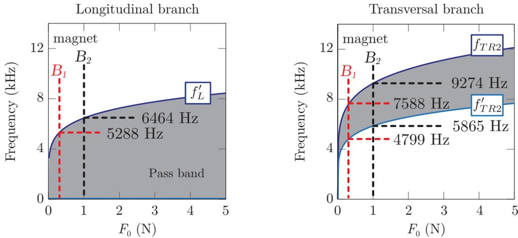
Figure 2.12: Cutoff frequencies for the  $L$  (left) and  $TR$  (right) branches as function of the normal force  $F_0$ . Experimentally estimated forces are  $F_0 = 0.3$  N (dashed red) and  $F_0 = 1$  N (dashed black) for permanent magnets of  $B_1$  and  $B_2$  remanent magnetization, respectively, both placed a distance 10 mm from the center of the beads. Grey zones correspond to pass bands. The torsional cutoff frequency is not shown.
