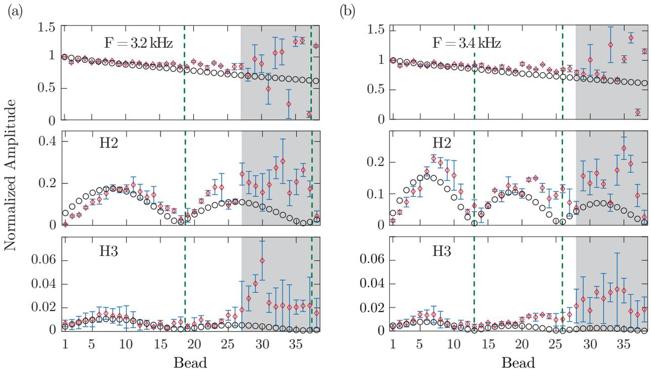
Figure 3.20: Experimental and numerical harmonic generation for a driving frequency of (a) 3.2 kHz:  $f_1/f_c = 0.44$  and (b) 3.4 kHz:  $f_1/f_c = 0.47$ . Black circles correspond to numerics and red diamonds to experiment, respectively. Green dashed line from Eq. (3.8). Grey zones correspond to the experimental presence of reflection during the analysis.
