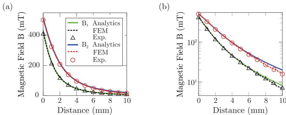
Figure 1.14: Magnetic flux density as a function of the distance from the upper surface of magnets for  $B_1 = 1.32$  T and  $B_2 = 1.37$  T from Eq. (1.30) (solid line), from 3D finite element simulations (dashed line) and experiments (marks) (a) in linear scale and (b) in log scale.
