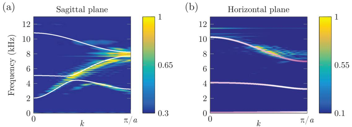
Figure B.3: Experimental dispersion curves for a chain of 26 beads for modes polarized in (a) sagittal and (b) horizontal planes. The theoretical existence of translational motion  $u_z$  is superimposed on panel (b) in color scale (white to magenta). Theoretical dispersion curves are plotted using  $F_0 = 2.1$  N ( $K_N$ ),  $F'_0 = 1.8$  N ( $K_S, K_T$ ),  $F = 10$  N ( $\tilde{K}_N, \tilde{K}_T$ ),  $F = 0.1$  N ( $\tilde{K}_S$ ).
