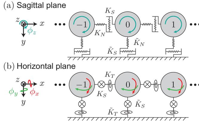
Figure 2.1: Representation of the infinite granular chain coupled with a rigid substrate. Displacement and rotation motions are separated in (a) the sagittal plane (displacements along  $x$  and  $y$ , rotation relative to  $z$ -axis) and (b) the horizontal plane (rotations relative to  $x$  and  $y$ -axes, displacement along  $z$ ).
