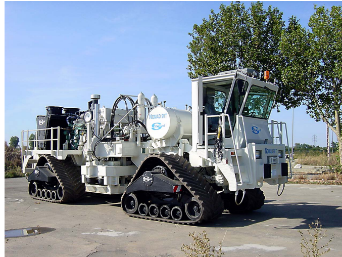
Figure 3.2: Seismic vibrator. This truck emits the sweep into the Earth in the frequency range: (5-250) Hz (courtesy: CGG).
