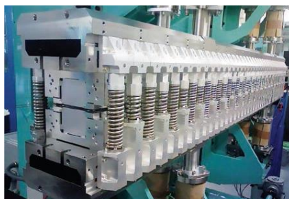
Figure II.24. Wiggler WS 50 of PSICHE beamline at synchrotron SOLEIL.
