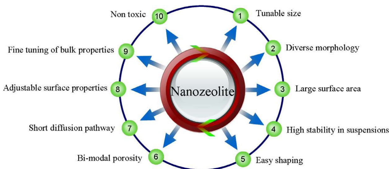
Figure 2 Properties of nanosized zeolites (reprinted from [57])
