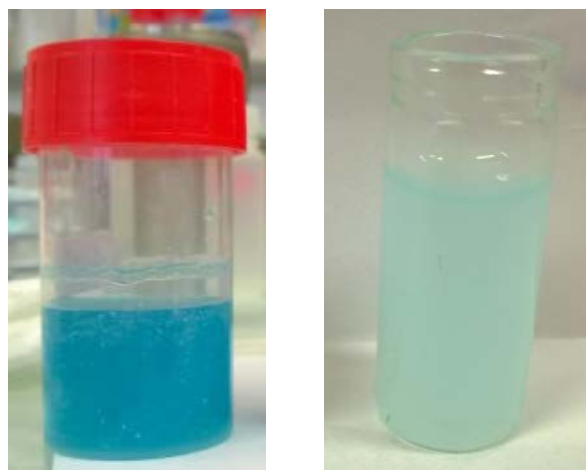
Figure 1 The image of the synthesis gel after 60 h of aging (left) and after hydrothermal crystallization (right)
