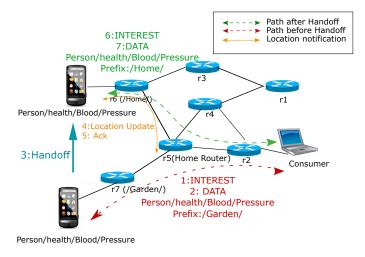
Figure 3.4: Locator/identifier separation approach
