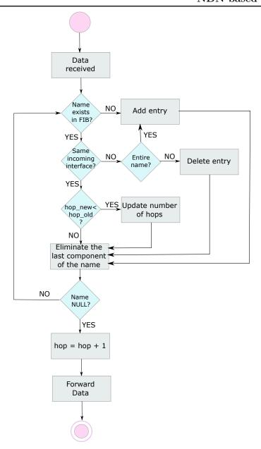
Figure 6.2: AFIRM algorithm: FIBs construction phase
