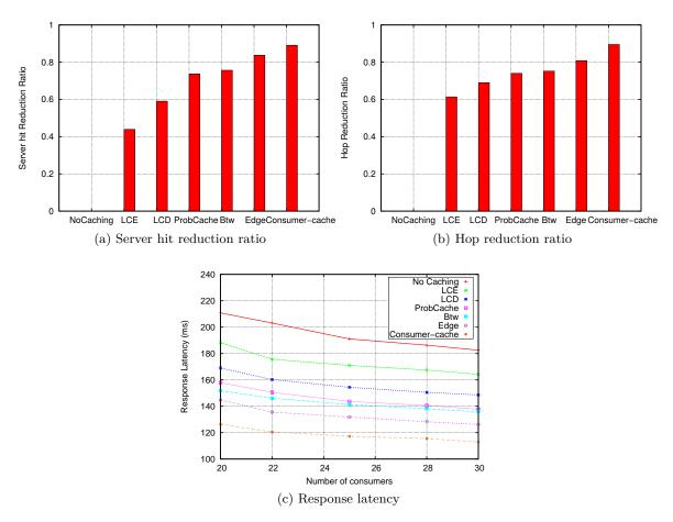
Figure 7.4: System performances for in-network caching
