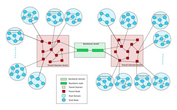
Figure 7.1: Transit-Stub topology model
