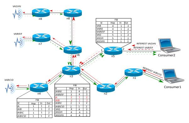
Figure 6.4: AFIRM example: FIBs construction phase
