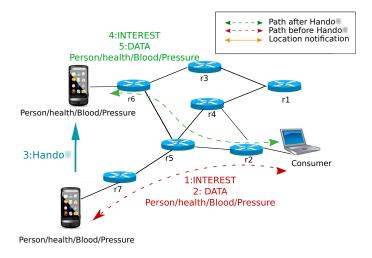
Figure 3.5: Routing-based approach
