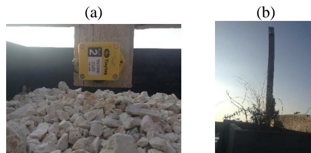
Figure 2-8: Waterproof and temperature sensor at the heights of: (a) 5 cm (b) 110 cm
