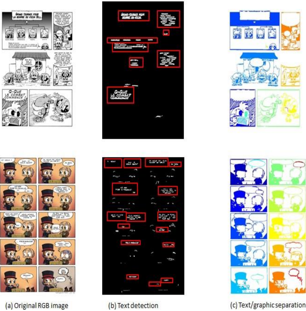
Figure 24: Text/graphic separation in the case of black text written in speech balloon with white background. (a) RGB processed comics. (b) Text detection results. The red rectangles illustrate detected texts. (c) Final results of text extraction from graphics
