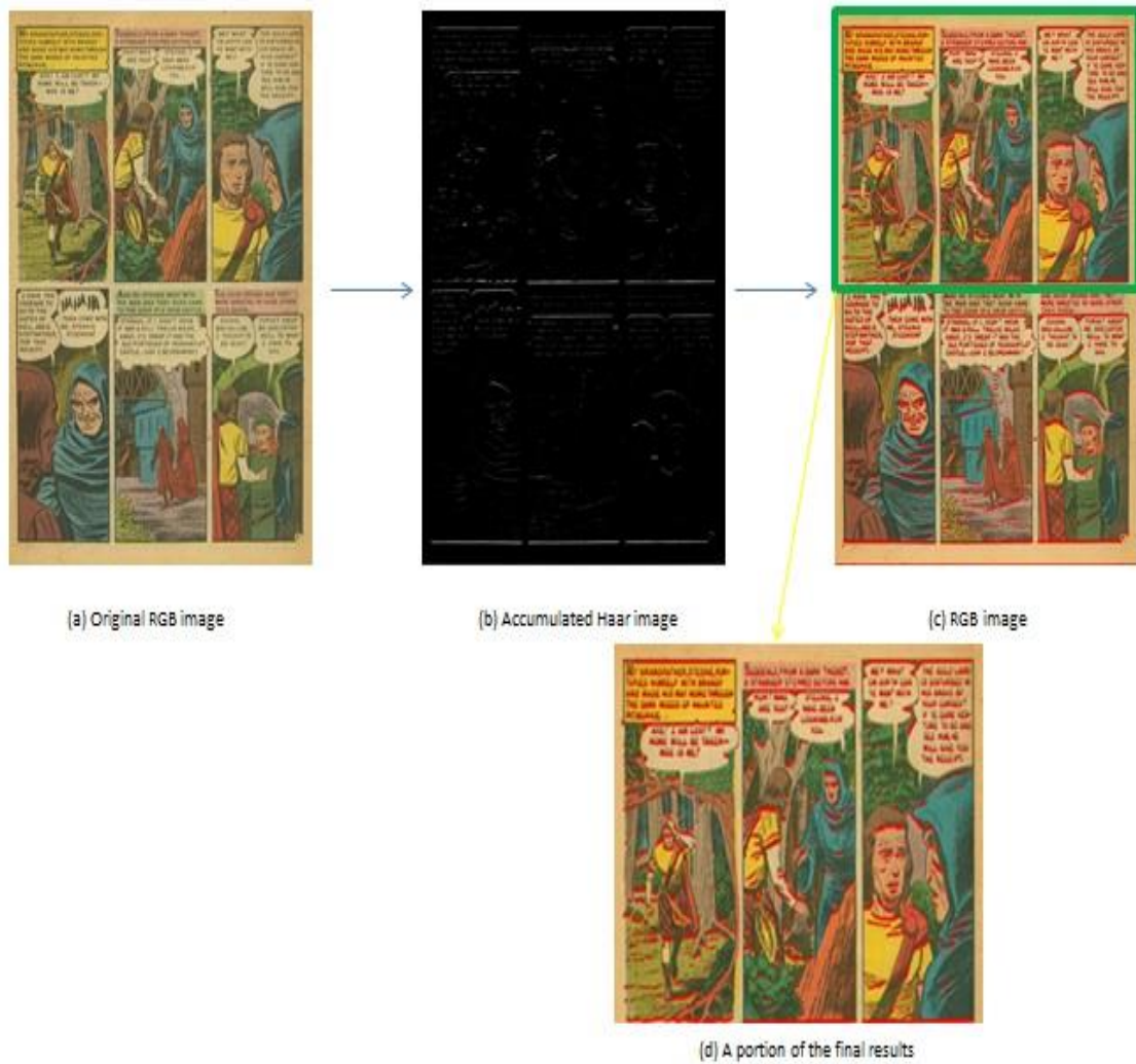
Figure 21: The text detection process based on asymmetric Haar-like features in digitized comics. (a) The RGB input comic image where text is written in black within speech balloons with various background colors. (b) The accumulated grey image resulting from applying two asymmetric Haar-like filters (Figure 19(b)) on the input comic. (c) The result image where text areas are represented by horizontal red shapes. (d) A zoomed portion of the final image.
