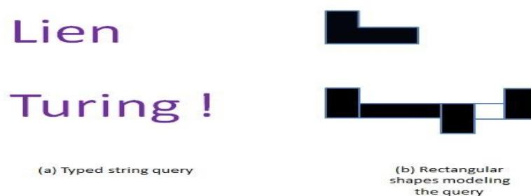
Figure 49: Modeling strings by rectangular shapes. (a) The user typed string (b) Black rectangles characterize the written letters, and the white one characterizes the blank space.
