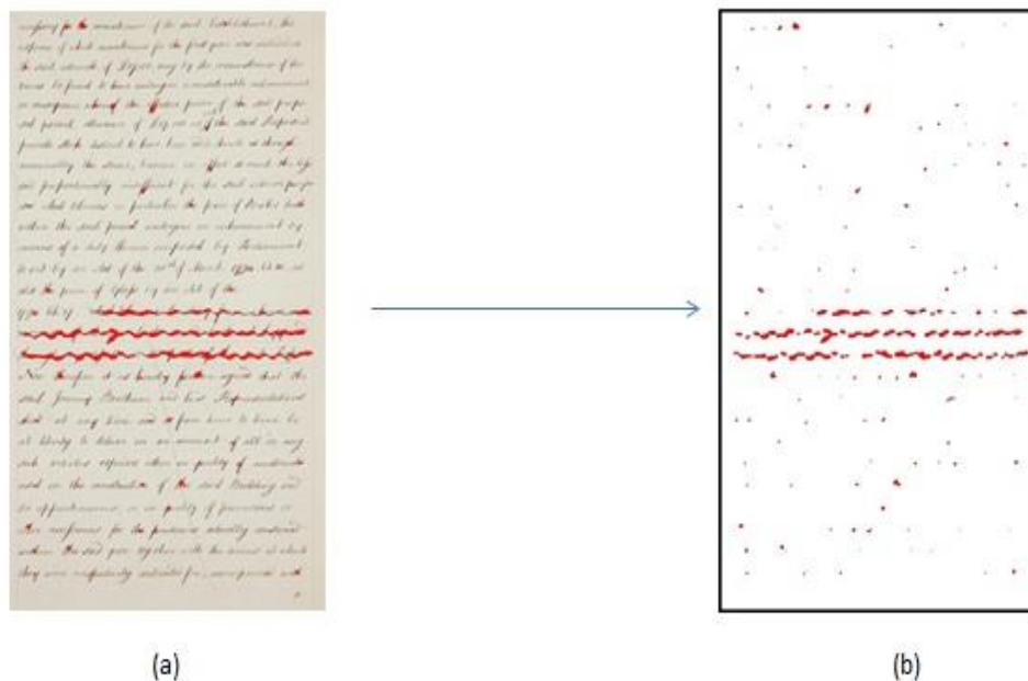
Figure 76: An example of a document page from Bentham Dataset where some text lines are crossed out. (a) The crossed text lines respond too much to the applied GHF. (b) We highlight only the red responses without textual components. For the Applied GHF, we used the first one in figure 75(b).
