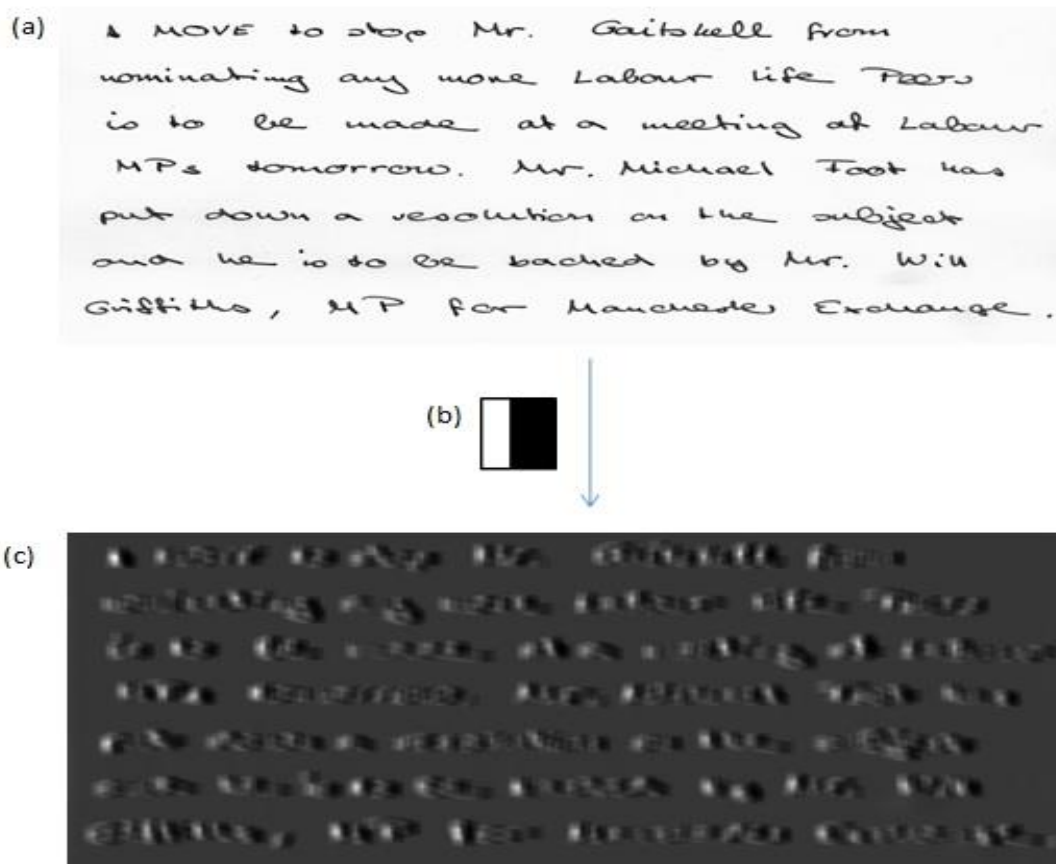
Figure 59: The transformed grey image obtained by applying an asymmetric GHF (b) on the manuscript document image (a). (b) The applied pattern permits detecting zones of interests beginning by an uppercase letter or a lowercase letter with an ascender. (c) The transformed grey image. The potential responses are highlighted in white within this image. They vote for the presence of the shape in that spatial area.
