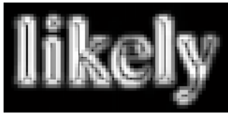
Figure 5.5.6: Color distance map produced by Smooth Watercolor. The pixel intensity represents the distance value.
