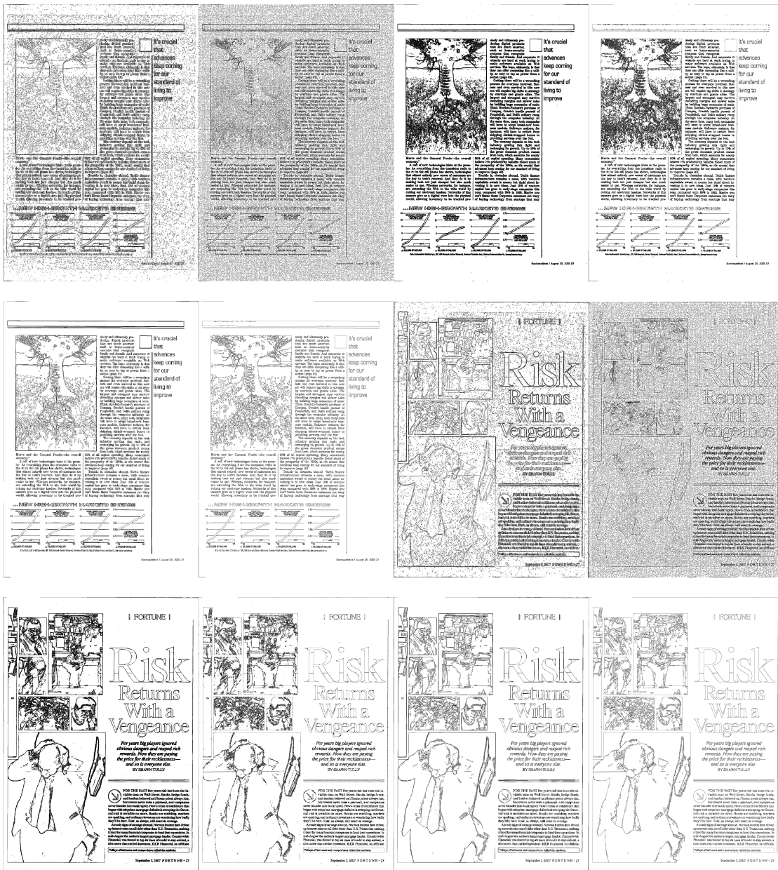
Figure 5.6.4: Results of the algorithms on two document images. Order for each series, line-wise from the top left image: FH, QS, WC, SWC, WCP, SWCP. The images produced by QS look gray because of the many region boundaries.
