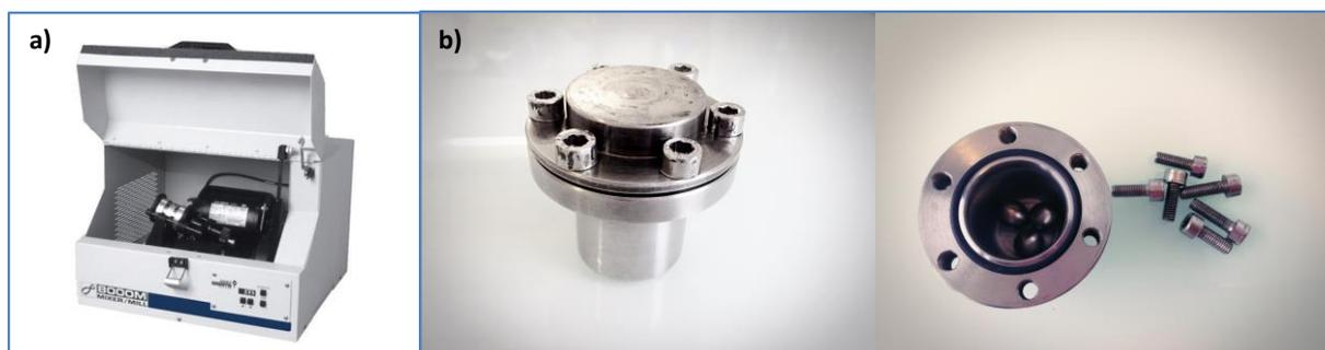
**Figure A.2:** (a) *SPEX 8000 Mixer/Mill®* (b) stainless steel ball-mill cylindrical cell with stainless-steel balls to be launched on the mixer.
