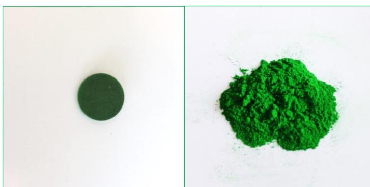
**Figure II.15:** The photo of pellet synthesized and the resulting ground powder of  $\text{Li}_2\text{Cu}_2\text{O}(\text{SO}_4)_2$ .
