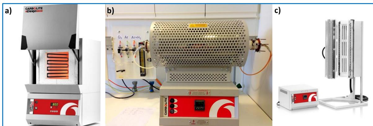
**Figure A.3:** (a) *CFW* laboratory chamber furnace (b) *EHC* compact horizontal tube furnace (c) *VST / TVS* Vertical Split Tube Furnace
