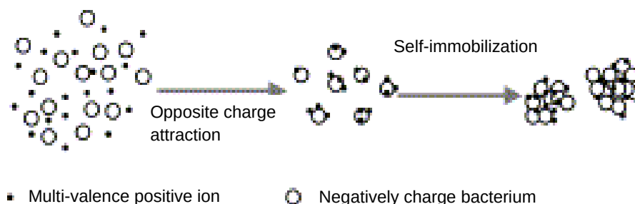
Figure 6: Schematic presents multi-valence positive ion-bonding model (Liu et al, 2003a).
