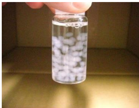
Figure 21 Image of gel beads formed by dropping polysaccharide solutions at a concentration of 0.5 wt% into alkaline and acid solutions of YbCl_3 \cdot 3H_2O .
