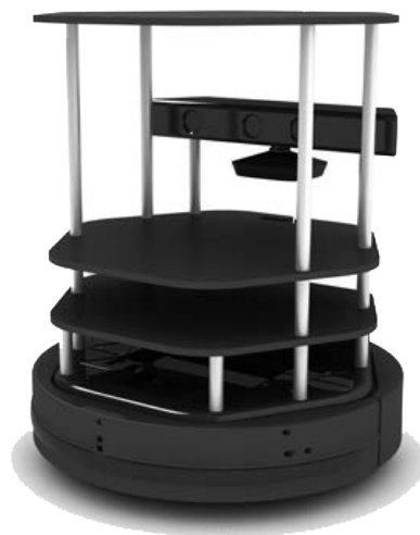
Figure 3.2: Turtlebot equipped with a Kinect sensor ( http://www.turtlebot.com ).
