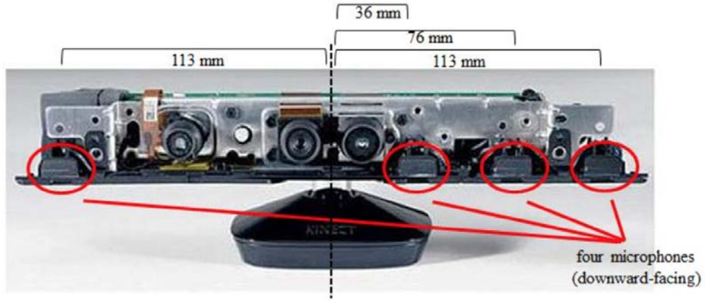
Figure 3.3: Linear array of 4 microphones inside the Kinect sensor ( https://www.microsoft.com ).
