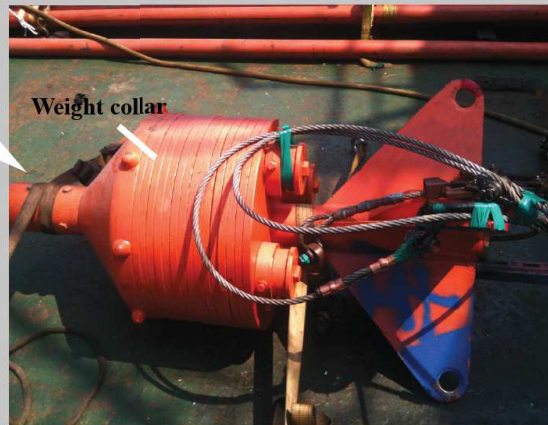
Orange peel closing system prevents the sample from exit.
