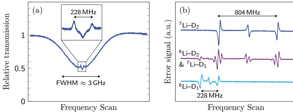
**Figure 6.11:** Doppler-free saturated absorption spectroscopy of the lithium D-lines. (a) Sample scan over the entire <sup>6</sup>Li D<sub>1</sub> Doppler-broadened absorption peak. The inset shows the sub-Doppler features. Similar spectra are obtained for all lithium D lines. (b) Error signals of all lithium D line transitions, generated by phase modulation spectroscopy. These signals provide an excellent reference for frequency-locking of the laser.
