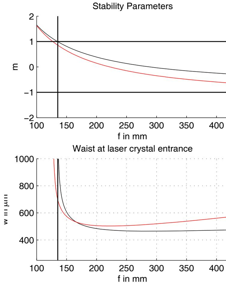
**Figure 5.11:** The stability diagram (upper panel, see Equation (5.14)) and the mode sizes (lower panel) in the laser crystal as a function of the thermal lens focal length  $f_{\text{th}}$ . The black (red) lines denote the horizontal (vertical) direction. The vertical line indicates the limit of cavity stability. The resonator remains stable down to  $f_{\text{th},\text{min}} = 135 \text{ mm}$ .
