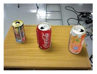
Figure 2.8: The model of the object is superposed on the actual image and flickered to trigger an SSVEP from the user.
