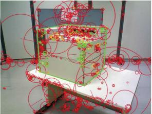
(a) Recognition result for a single object in the robot's field-of-view. The circles represent the SIFT features. Green circles represent match with the cookbook of the object, yellow circles represent partial matches and red circles represent non-matching features.
