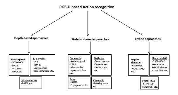
FIGURE 2.6: Overview of RGB-D based human action descriptors divided into three main groups: depth-based, skeleton-based and hybrid descriptors
