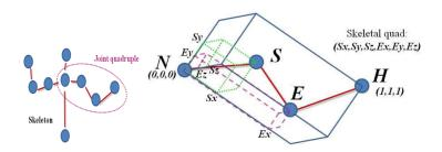
FIGURE 2.13: Skeletal quad representation calculated based on 4 joints introduced in [30]
