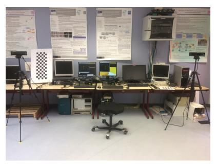
FIGURE 6.2: The RGB-D cameras positioning during the dataset acquisition: it can be noted the presnece of two RGB-D cameras (Kinect 2) with different viewpoints
