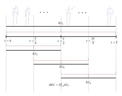
FIGURE 5.3: Computation of the Hierarchical Kinematic Covariance (HKC) descriptor as in [45]: T corresponds to the skeleton sequence length and  $KC_1$ ,  $KC_2$ ,  $KC_3$  and  $KC_4$  are the covariance matrices calculated from each corresponding range.
