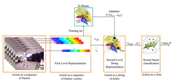
FIGURE 2.8: Overview of the method proposed in [12] where the notion of "actlet" is introduced: Feature vectors are first extracted from images. Then, each feature vector  $V_t$  is associated to a high level representation  $s_t$  thanks to the alphabet C learned during the training phase. Finally, the action is recognized using a kernel-based classification
