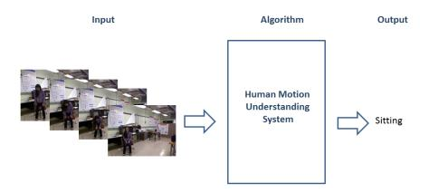
FIGURE 2.1: An example of a human motion understanding system: In this example, the input data represents an RGB video (a sequence of RGB images) where we can observe someone sitting. Therefore, using these input data, the system is able to recognize the observed action and returns as output its label "sitting".
