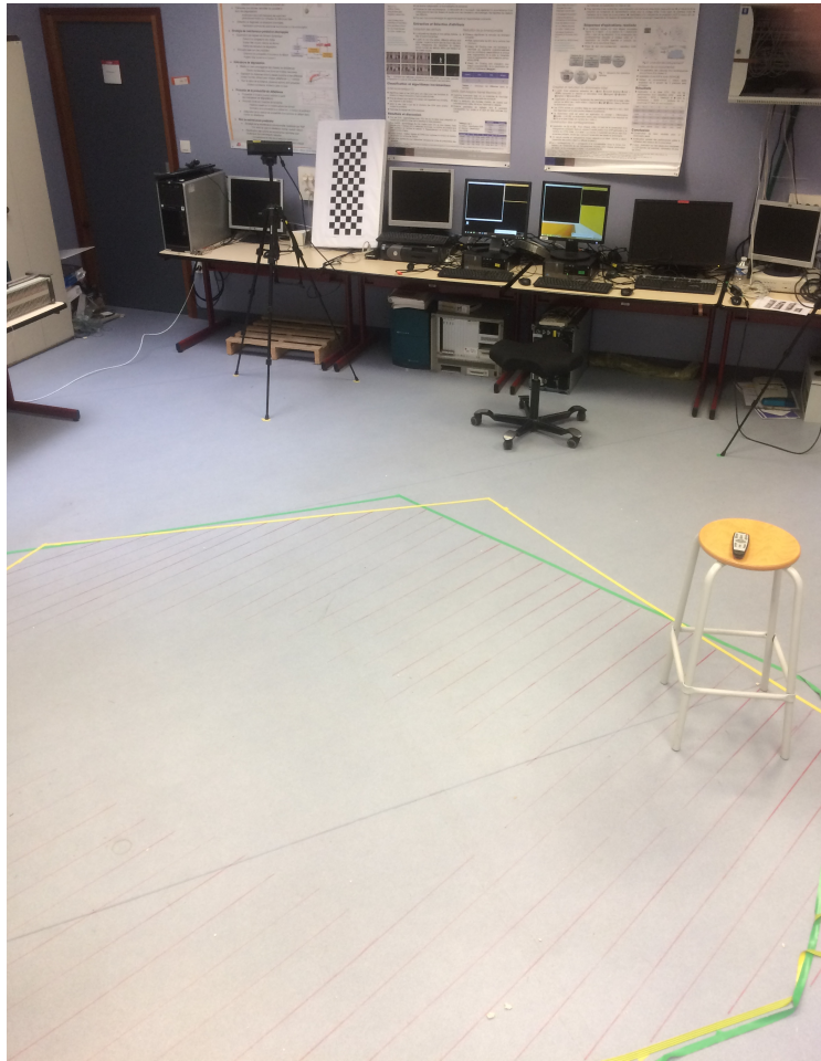
FIGURE 6.1: The experimental conditions of the dataset acquisition: the green surface represents the limits of the scene observed by the first camera, while the yellow surface represents the limits of the scene observed by the second camera.
