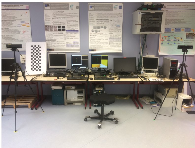
FIGURE 6.2: The RGB-D cameras positioning during the dataset acquisition: it can be noted the presence of two RGB-D cameras (Kinect 2) with different viewpoints
