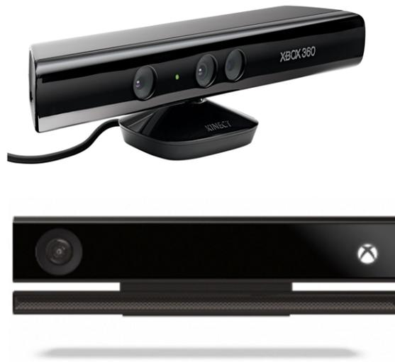
FIGURE 2.4: Examples of RGB-D cameras: Kinect 1 (on the top) and Kinect 2 (in the bottom)
