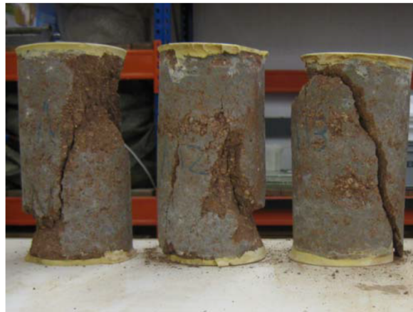
FIGURE 1.23: Specimens after triaxial tests [CWHM12]
