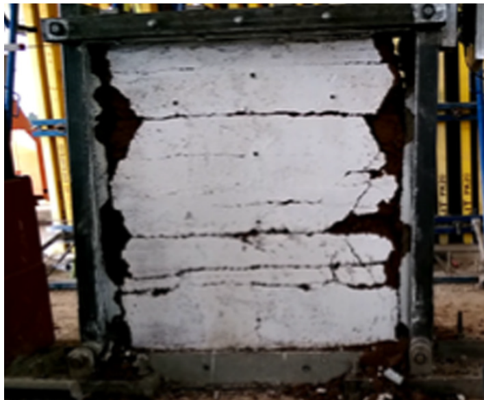
FIGURE 1.40: Crack pattern after pushover test for unstabilised rammed earth [AEY17]
