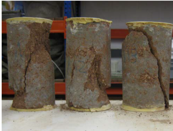
FIGURE 1.23: Specimens after triaxial tests [CWHM12]
