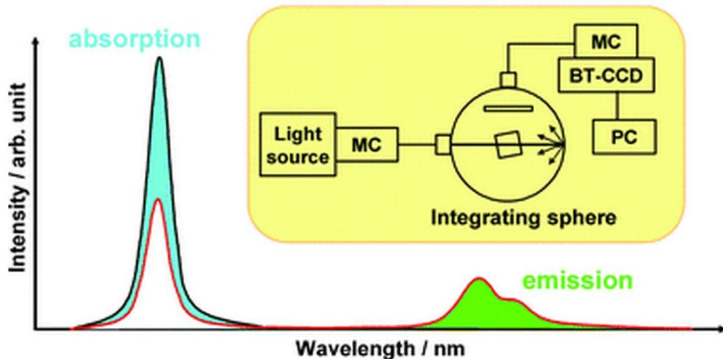
**Figure 7.3.** Schematic representation of an integrating sphere (IS) for measuring absolute luminescence quantum yields. MC stands for monochromator, and BT-CCD is a back thinned CCD. The number of photons absorbed is proportional to the difference of the integrated excitation light profiles, while the number of photons emitted is proportional to the area under its fluorescence spectrum.<sup>3</sup>
