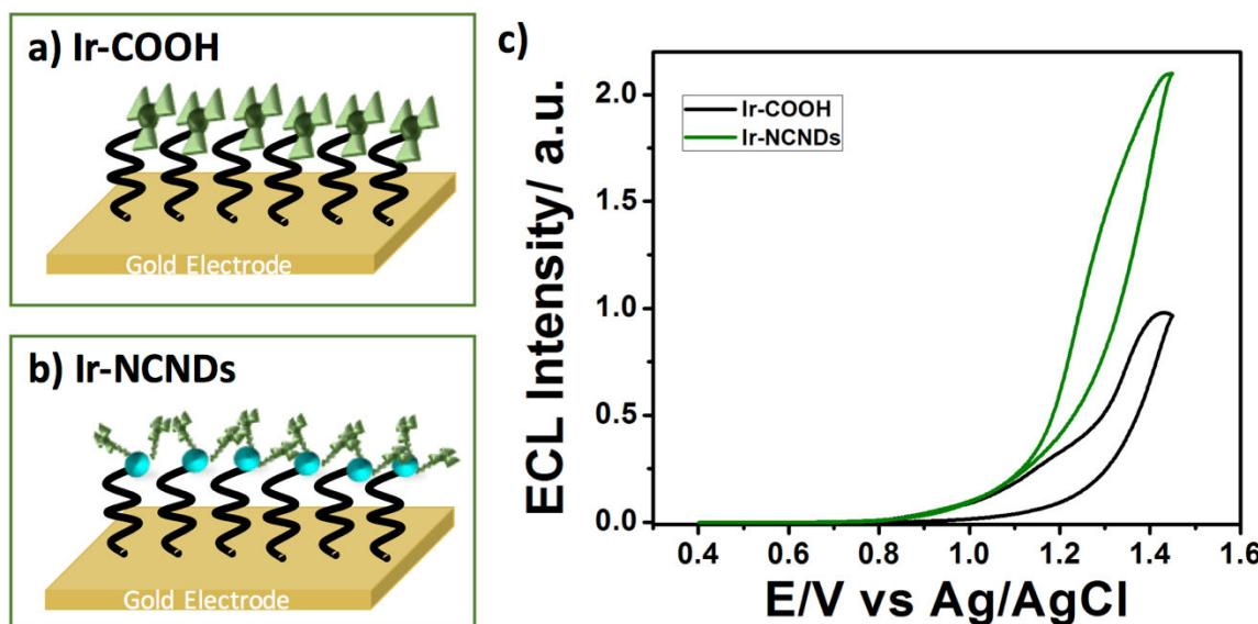
**Figure 5.17.** Schematic representation of a) Ir-COOH and b) Ir-NCNDs immobilization onto gold electrodes; c) ECL Intensities recorded during a CV in PBS/ Triton X 100/ TPrA 10 mM of Ir-NCNDs (green trace) and Ir-COOH (black traces) after immobilization. Scan rate 0.05 V s<sup>-1</sup>.
