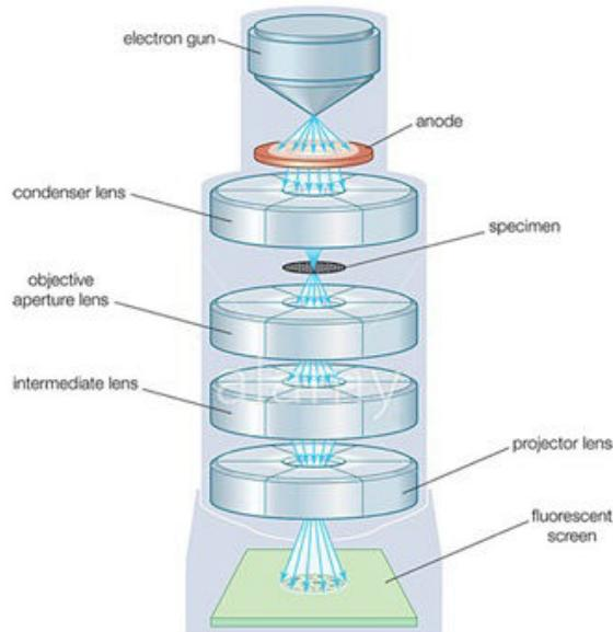
*Figure 7.7. Schematic representation of a TEM setup.*
