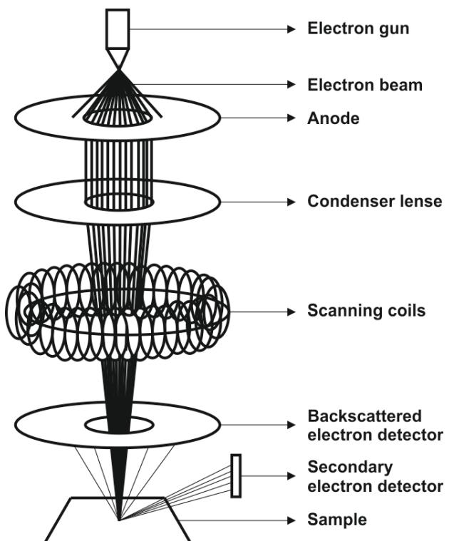
Figure 7.5 Schematic representation of a SEM setup.
