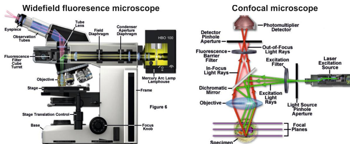
**Figure 7.6.** Simplified setup of a widefield fluorescence microscope (left) and schematic representation of a Laser Scanning Confocal Microscope (right) adapted from [www.zeiss.com](http://www.zeiss.com).
