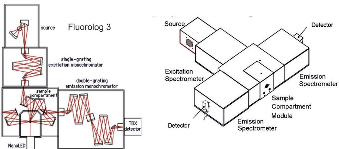
**Figure 7.2.** Schematic representation of the fluorescence spectrophotometer Fluorolog 3 model FL3-12 from Horiba Scientific (source: [www.horiba.com](http://www.horiba.com)).
