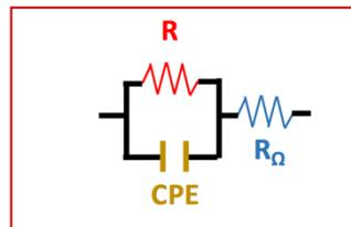
**Figure 6.11.** Equivalent circuit model representing the cTnI immunoassays.
