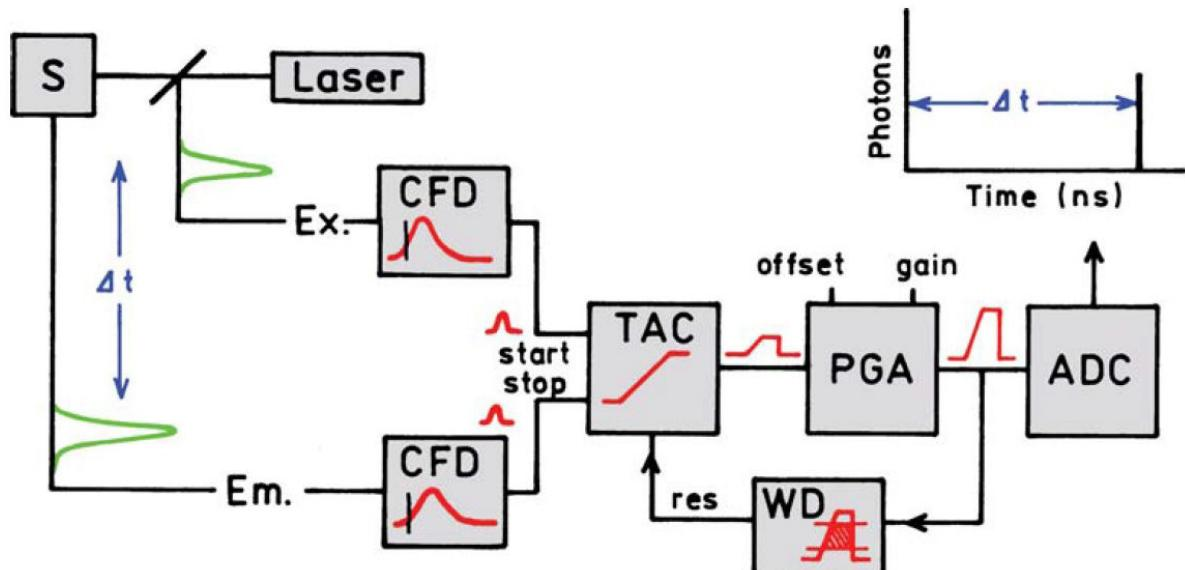
Figure 7.4. Electronic schematic for TCSPC.<sup>4</sup>
