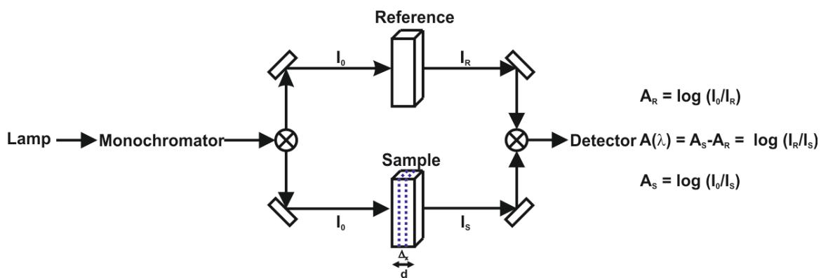
**Figure 7.1.** Schematic description of a double beam spectrophotometer.
