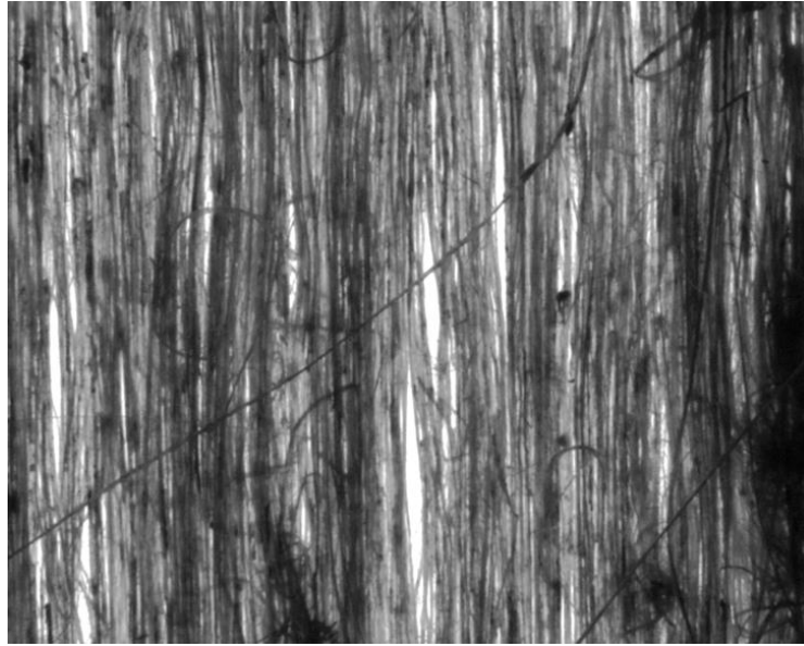
Fig. 2.7 Typical unidirectional ply of flax (without matrix). Some of the fibers (elementary fibers or bundle of fibers) are not aligned in the longitudinal direction (UD70).
