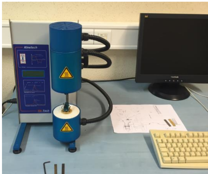
Fig. 2.14 Kinetech apparatus for glass transition measurement
