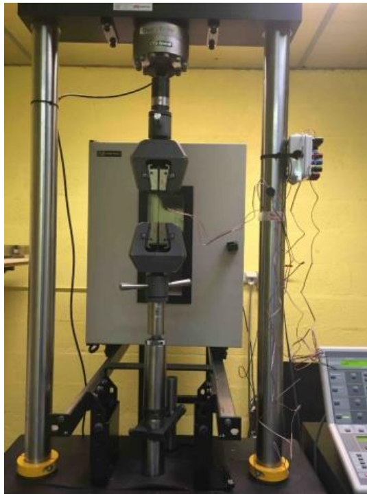
Fig. 2.12 Instron servo-hydraulic machine
