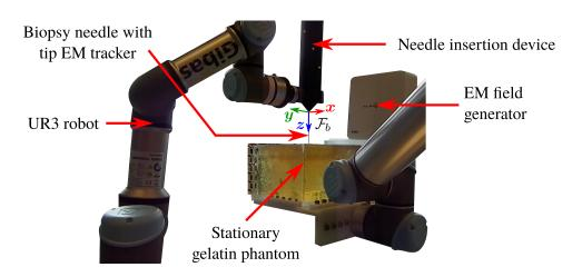
Figure 2.8: Picture of the setup used to acquire the trajectory of the tip of a real needle inserted in a gelatin phantom. The frame attached to the needle base is denoted by  $\{\mathcal{F}_b\}$ .
