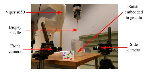
Figure 4.9: Picture of the setup used to test the performances of the different safety tasks.
