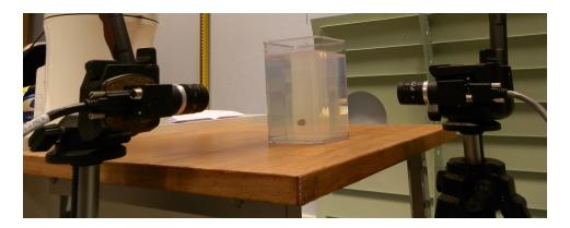
Figure 1.7: Picture of the stereo camera system and one gelatin phantom used for the experiments.
