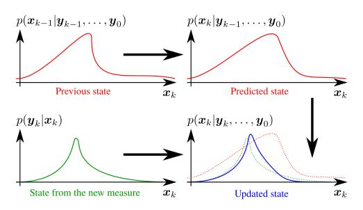
Figure 3.13: Illustration of the principle of Bayesian filtering
