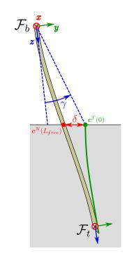
Figure 4.5: Illustration of the geometric features used for the safety task functions. Note that the representation is here limited to a 2D case, however in the general case the angle  $\gamma$  is defined in the plane containing the needle base axis  $\boldsymbol{z}$  and the initial insertion point  $\boldsymbol{c}^{T}(0)$ .
