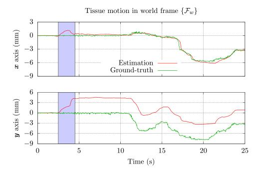
Figure 3.30: Example of tissue motions estimated using the update method 4 with the position feedback obtained from cameras. At the beginning of the insertion (blue zone from t = 2.5s to t = 4.5s), the needle base is moved laterally such that a tearing occurs at the surface of the gelatin. This creates an offset in the estimation of the motions of the tissues.
