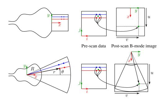
Figure 3.4: Illustration of 2D post-scan conversion for linear (top) and convex (bottom) transducers.
