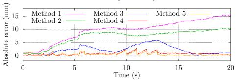
Simulated needle tip absolute position error
