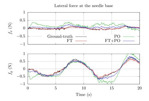
Figure 3.21: Example of forces measured and estimated using three different combinations of feedback for the update algorithm: force and torque feedback (FT, red), tip position and orientation feedback (PO, green) and feedback from all sources (FT+PO, blue).
