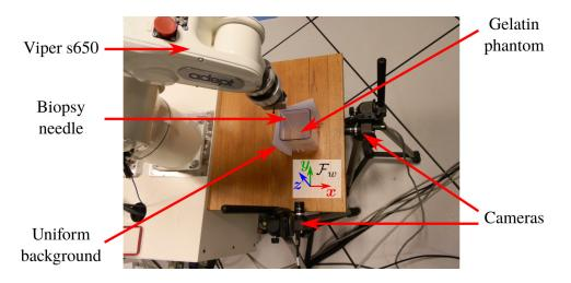
Figure 3.24: Experimental setup used to validate the performances of the tissue motion estimation algorithm when using the visual feedback provided by two cameras to detect the position of the needle body.
