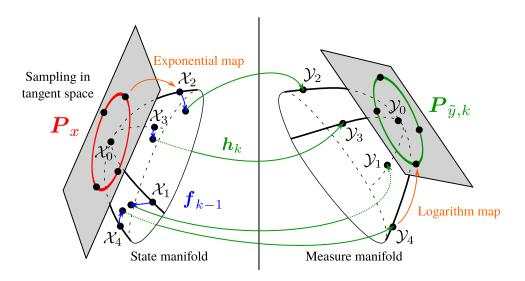
Figure 3.16: Illustration of the unscented Kalman filter on manifolds.
