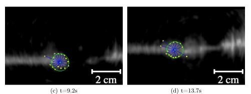
Figure 5.11: Target tracking in ultrasound images during a needle insertion in a gelatin phantom. The needle can be seen coming from the right.
