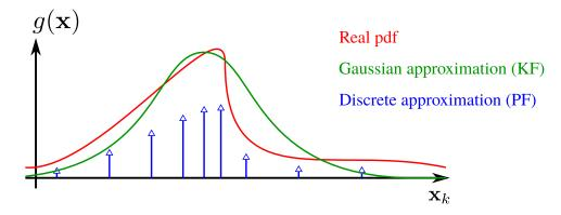
Figure 3.14: Illustration of the pdf approximations used by Kalman filters (KF) and particle filters (PF).
