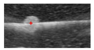
Figure 5.12: Slice extracted from a 3D ultrasound volume acquired at the end of an insertion in the gelatin phantom. The needle is coming from the right and the needle tip is shown with a red cross. The line on the left corresponds to a wooden stick used to maintain the spherical target during the conception of the phantom.
