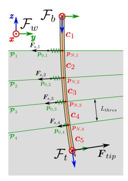
Figure 2.5: Illustration of the mechanical 3D model of needle-tissue interaction using virtual springs and a reaction force at the tip.
