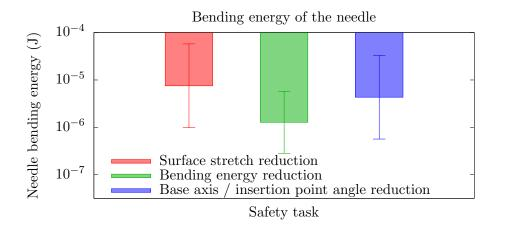
Figure 4.16: Mean value of the energy of bending stored in the needle. The mean is taken over time and across the five experiments for each kind of safety task.
