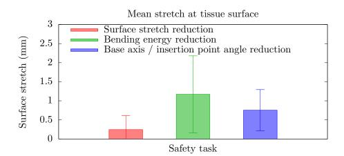
Figure 4.14: Mean value of the distance between the needle and the initial position of the insertion point at the tissue surface. The mean is taken over time and across the five experiments for each kind of safety task.
