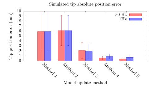
Figure 3.25: Mean over time and across five experiments of the absolute error between the real and modeled tip position obtained for the different update methods and two different update rates.
