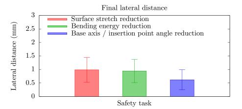
Figure 4.12: Mean value of the final distance between the needle tip axis and the target. The mean is taken across the five experiments for each kind of safety task.
