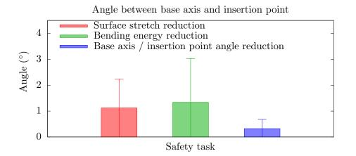
Figure 4.18: Mean value of the angle between the needle base axis and the initial position of the insertion point at the tissue surface. The mean is taken over time and across the five experiments for each kind of safety task.
