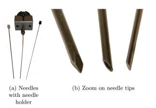
Figure 1.6: Picture of the needles used for the experiments. From left to right: Greene biopsy stylet, Chiba biopsy needle, Chiba biopsy stylet.
