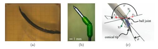
Figure 1.4: Example of special designs of the needle tip: (a) multi-segment needle (taken from [KFRyB11]), (b) one degree of freedom active pre-bent tip (taken from [AGL<sup>+</sup>16]) and (c) two degrees of freedom active prebent tip (taken from [RvdBvdDM15]).
