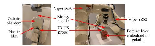
Figure 4.21: Pictures of the experimental setup used for the validation of the framework with 3D ultrasound (US) imaging. The whole setup is depicted on the picture on the right using the phantom with porcine liver embedded in gelatin. A zoom on the interface between the US probe and the gelatin phantom is shown on the left.
