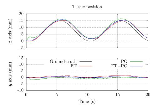
Figure 3.23: Example of tissue motions measured and estimated using three different combinations of feedback for the update algorithm: force and torque feedback (FT, red), tip position and orientation feedback (PO, green) and feedback from all sources (FT+PO, blue).
