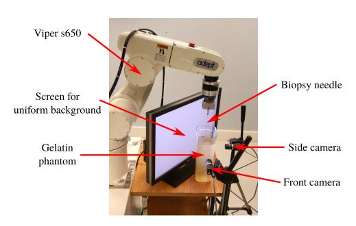
Figure 4.6: Picture of the setup used to test the hybrid base manipulation and duty-cycling controller.
