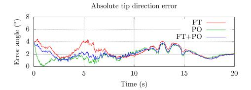
Figure 3.20: Example of absolute direction error (angle between two direction vectors) between the measured tip direction and the estimated one using three different combinations of feedback for the update algorithm: force and torque feedback (FT, red), tip position and orientation feedback (PO, green) and feedback from all sources (FT+PO, blue).
