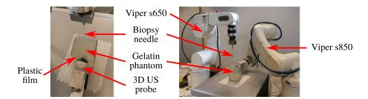
Figure 3.10: Picture of the setup used to acquire volume sequences of needle insertions in a gelatin phantom. The Viper s650 robot holds the needle on the left and the Viper s850 robot holds the probe on the right.
