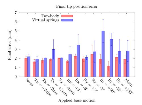
Figure 2.14: Absolute final error between the position of the simulated needle tip and the measured position of the real needle tip. For each type of base motions, the mean and standard deviation are calculated using the final position error across 3 different insertions performed in the phantom.
