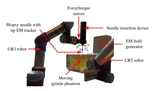
Figure 3.18: Experimental setup used to validate the performances of the tissue motion estimation algorithm when using force feedback at the base of the needle and position feedback at the needle tip.
