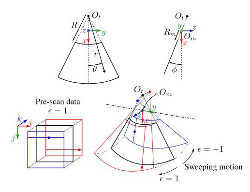
Figure 3.5: Illustration of 3D post-scan conversion for a convex transducer wobbling probe.
