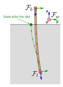
Figure 3.17: Illustration of the two-body model and definition of the state  $\boldsymbol{x}$  considered for the unscented Kalman filter (UKF).
