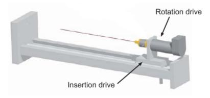
Figure 1.3: General concept of a needle insertion device (taken from [WMO05]).
