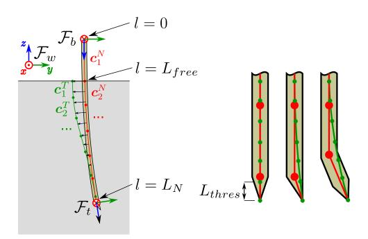
Figure 2.7: Illustration of the whole needle insertion model (left) and zoom on the tip for different tip geometries (right). Needle segments are in red and the rest position of the path cut in the tissues is in green. New segments are added to the cut path according to the location of the cutting edge of the tip.
