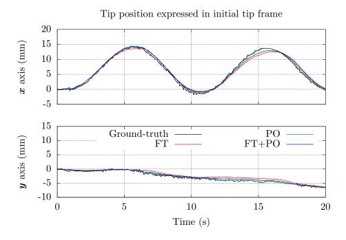
Figure 3.19: Example of tip position measured and estimated using three different combinations of feedback for the update algorithm: force and torque feedback (FT, red), tip position and orientation feedback (PO, green) and feedback from all sources (FT+PO, blue).
