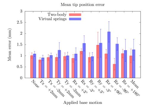
Figure 2.15: Average absolute error during the whole insertion between the position of the simulated needle tip and the measured position of the real needle tip. For each type of base motions, the mean and standard deviation are calculated over the whole length of the insertion and across 3 different insertions performed in the phantom.
