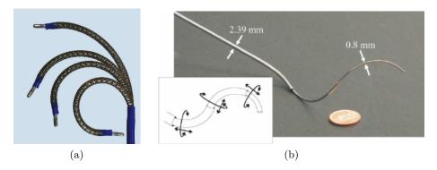
Figure 1.1: Example of (a) continuum robot (taken from [CMC<sup>+</sup>08]) and (b) concentric tubes (taken from [WRC09]).
