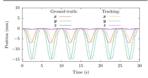
Figure 5.2: Illustration of the performance of the target tracking algorithm. The motion described by (5.4) is applied to the gelatin phantom with a period T = 5s. The global mean tracking error is 3.6 mm for this experiment. However it reduces to 0.6 mm after compensating for the delay of about 450 ms introduced by the data acquisition.
