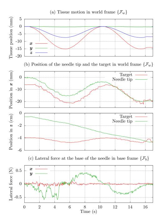
Figure 5.9: Measures during an insertion in a bovine liver embedded in gelatin: (a) Measure of the tissue motion from the UR5 odometry, (b) measure of the needle tip position from the electromagnetic tracker and measure of the target position from the tracking in 2D ultrasound, (c) measure of the lateral force exerted on the base of the needle. Overall the target can be reached and the lateral motion of the tissues is compensated such that the lateral force remains low.
