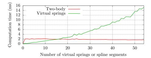
Figure 2.16: Computation time needed to get the shape of the needle from the base pose and position of the tissue model (virtual springs or spline segments).
