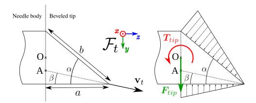
Figure 2.6: Illustration of the reaction forces applied on each side of the bevel (depicted on the right). Point O corresponds to the end of the 3D curve representing the needle. The current velocity of the needle tip  $\mathbf{v}_t$  defines the angle  $\beta$  in which the cutting occurs in the tissues.
