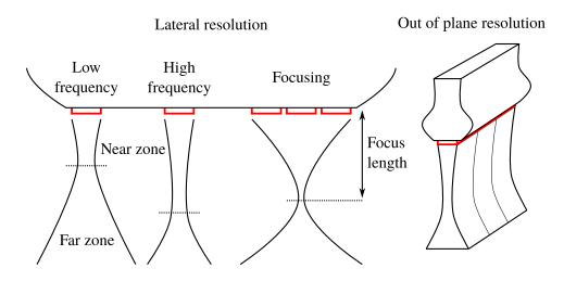
Figure 3.3: Illustration of the effect of US beam width on the lateral and out of plane resolution of an US probe. Piezoelectric elements are represented in red and only a linear transducer is depicted here.
