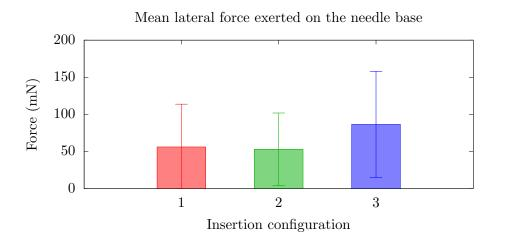
Figure 5.6: Mean value of the absolute lateral force exerted at the base of the needle. The mean is taken over time and across the four experiments for each configuration.
