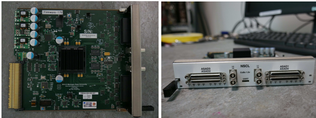
Figure 5.20: Photograph of a CoBo module of the TPC demonstrator at CENBG. The left picture shows the top-view of the card with the backplane connectors on the left. The right picture is the front view of CoBo. Four VHDCI connectors to the AsAd cards are here. The four LEMO connectors labelled L0, L1, L2 and L3 send the trigger signals (NIM) for each AsAd. A \mu USB port is available at the centre.
