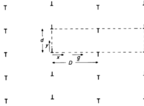
Figure 1.16 – Schematic view of the dislocation arrangement considered by Wilkens [30].
