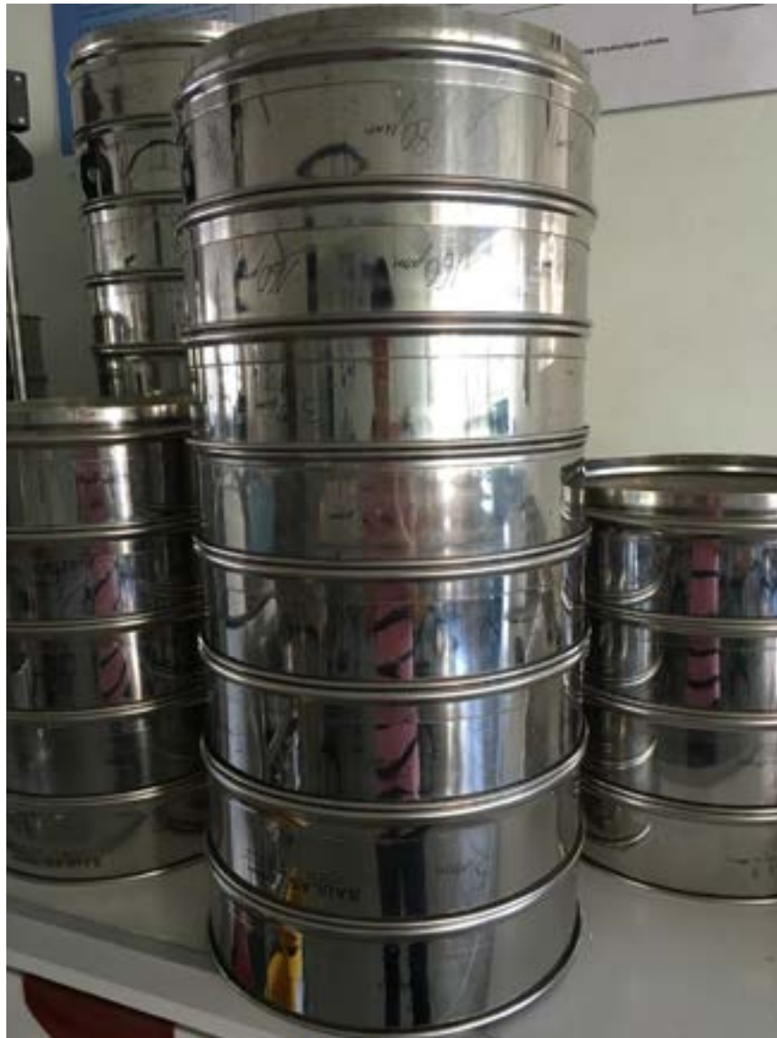
Figure 4.12 Sieves for granulometric analysis
