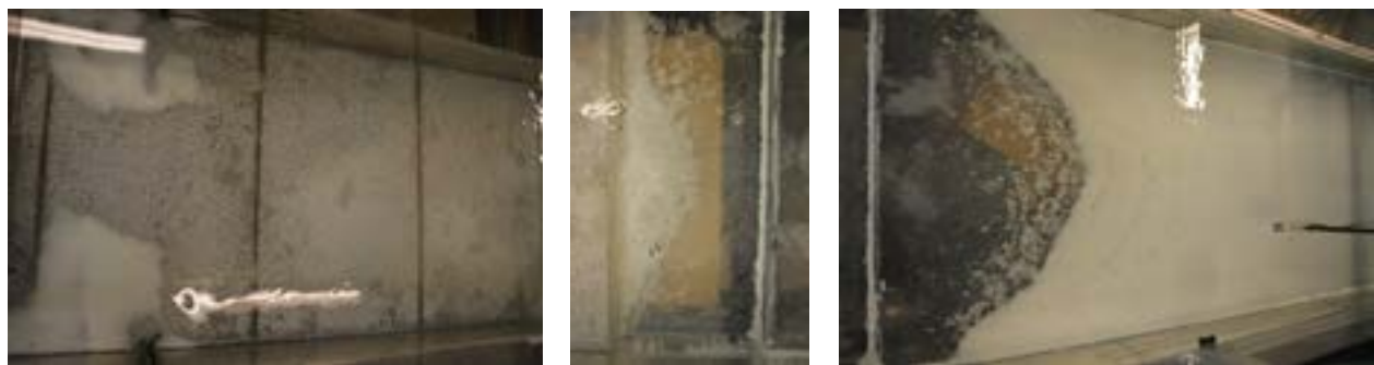
Figure 4.58 Sediment distribution at 3 L/s 2 hours after particle release
