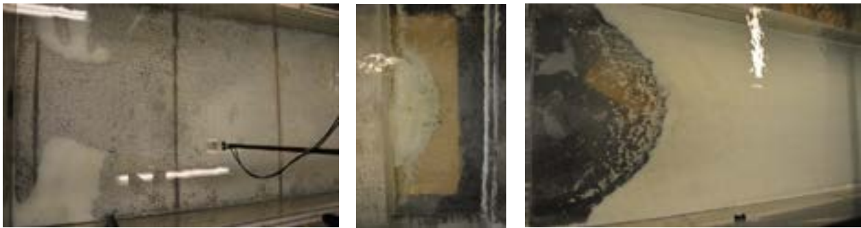
Figure 4.60 Sediment distribution at 3 L/s 4 hours after particle release
