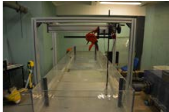
Figure 4.9 Support for fixing the transducer
