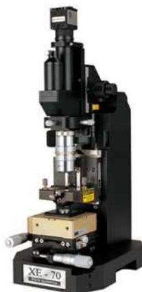
Figure A4.3: Microscope à force atomique XE-70 de Park Systems.
