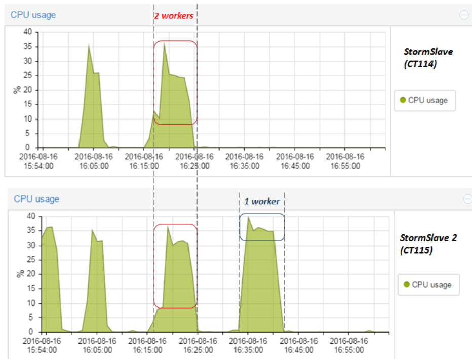
Figure 4.12: CPU consumption in the Storm supervisors when processing 1,200,000 streams
